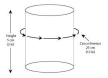
Fig. 4. Calculation of the Area of the Principal Display Area of a Cylindrical Container
