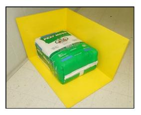
Figure 3-1. Dimensional Measuring Frame
