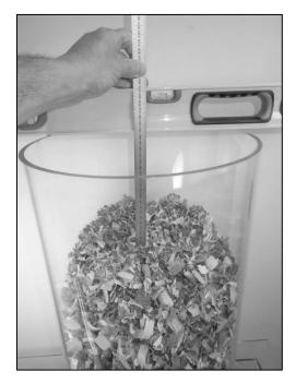
Figure 3-26. Placing the Ruler into the Test Measure with Zero End Down.
