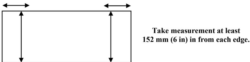
Figure 4-5. Determining Width.
