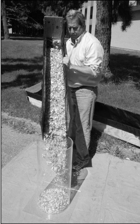
**Figure 3-23. Filling a 44 L Test Measure.**
