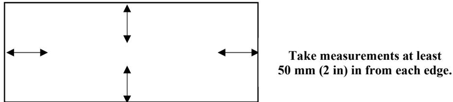
**Figure 4-6. Determining Thickness.**
