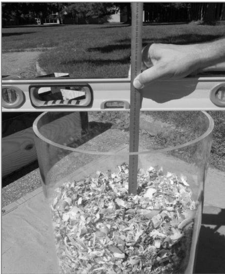
**Illustration 4.** Illustrating how the ruler is placed on the bedding with the headspace method. The ruler is read from the bottom edge of a straight edge or level from a position that reduces parallax.
