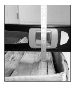
Figure 3-9a. Examples of the Headspace Measurement.
