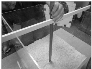
Illustration 4. Showing how the ruler is placed on the bedding with the headspace method. The ruler is read from the bottom edge of a straight edge or level from a position that reduces parallax.
