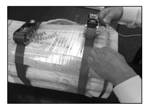
Figure 3-13a. Strapping the Ends of a Bundle.
