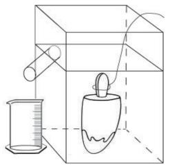
Figure 3-7. Example of a Displacement Vessel.
