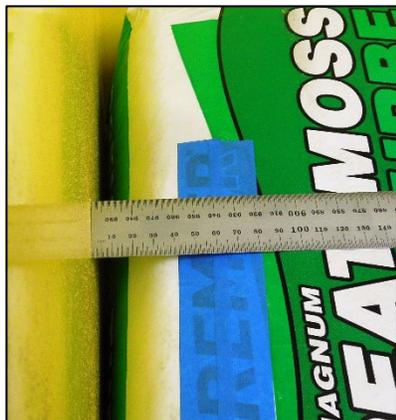
**Figure 3-3. Rigid Frame.** The rigid frame allows the observer to hold the zero reference point firmly in place.
