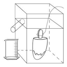
Figure 3-7. Example of a Displacement Vessel.
