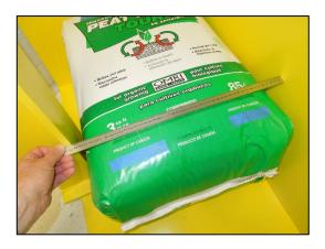
Figure 3-4. Length Measurement.
