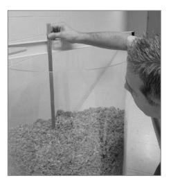
Illustration 3. Using the headspace measurement on a 279 L test measure. The ruler is read from the bottom edge of a straight edge or level from a position that reduces parallax.
