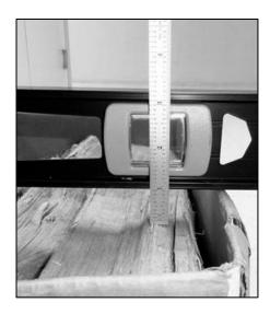
Figure 3-9a. Examples of the Headspace Measurement.
