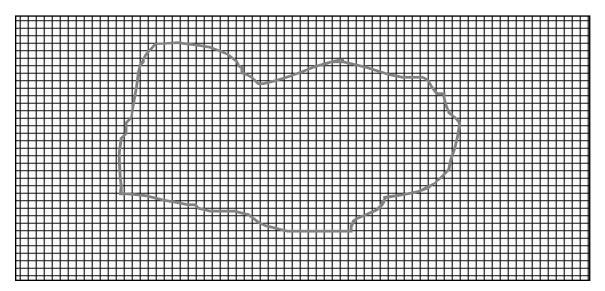
Figure 4.3. Template for Checking the Area of Chamois.
