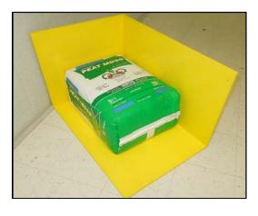
Figure 3-1. Dimensional Measuring Frame
