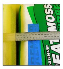
Figure 3-3. Rigid Frame. The rigid frame allows the observer to hold the zero reference point firmly in place.
