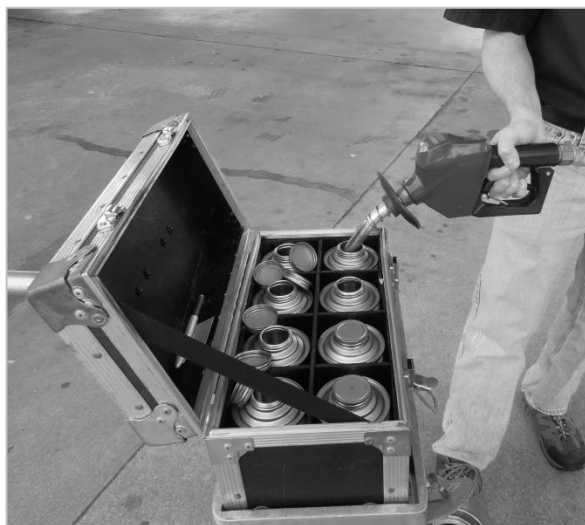
18. Fuel Sampling Cart with Sample Container bonded to cart and ground.*
