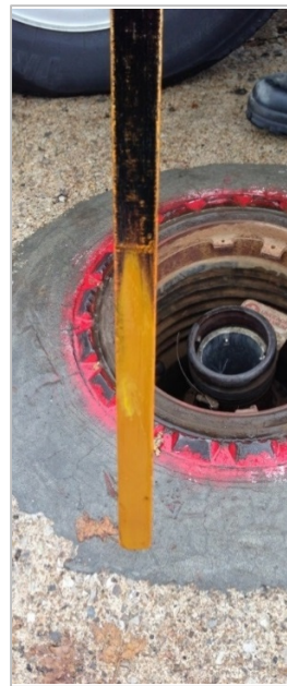
Figure 22. Stick with Paste – No Water Indicated.
