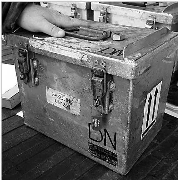
Figure 13c. Sample Box showing Security Seal in Place
