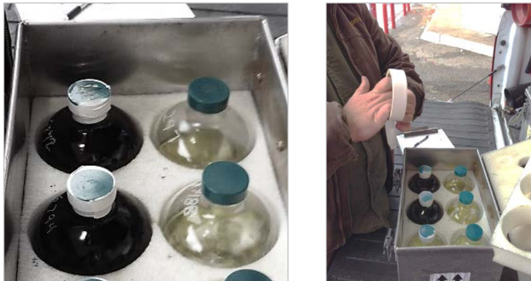
Figure 19. Sealing Tape Applied to Amber Sample Bottles
