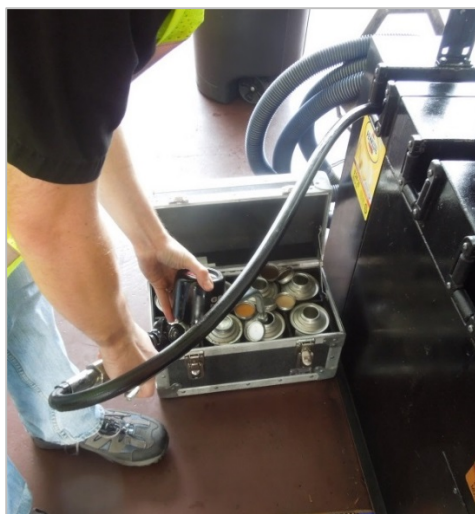
Figure 25. Taking Oil Samples – Metal Cans.
