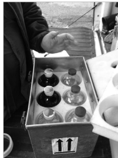
Figure 13b. Sample Box Showing Insulation.
