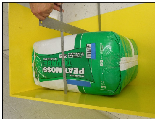
Figure 3-6. Width Measurement – The frame is rotated on its end to vertical so that the carpenter square does not compress the product.
