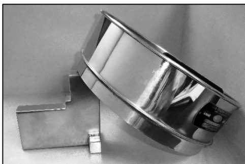
Figure 2-3. Sieve with Tilt Block Set at 30 Degrees.
