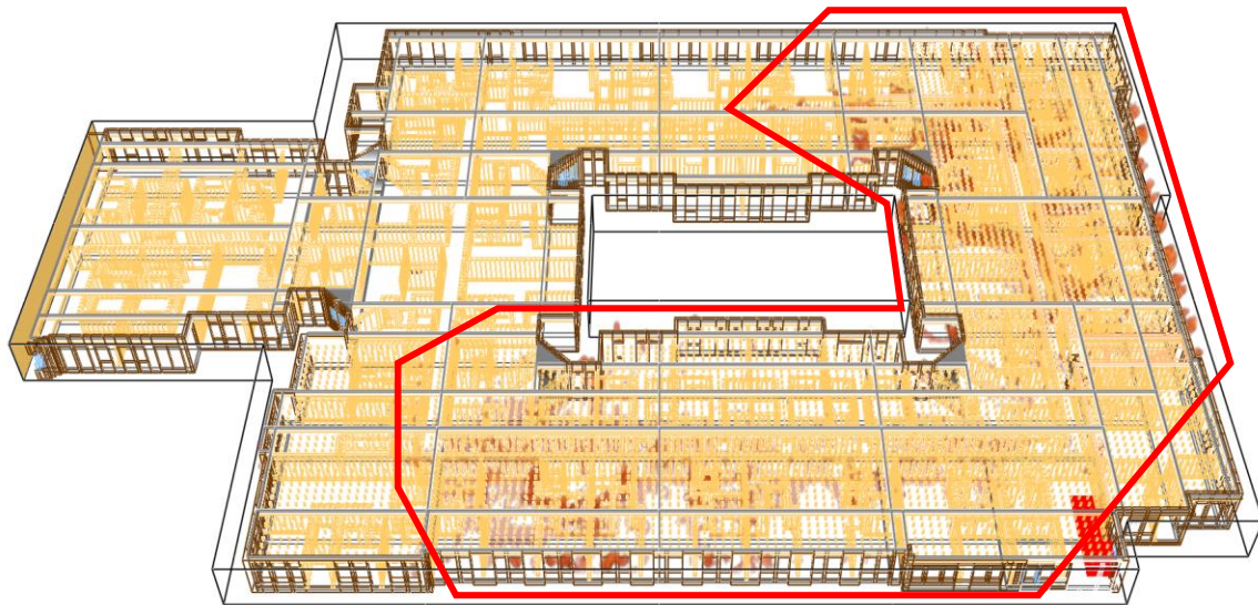
Figure 42. Baseline Low-Resolution Model Simulation at Time of Maximum HRR (t=1400s)
