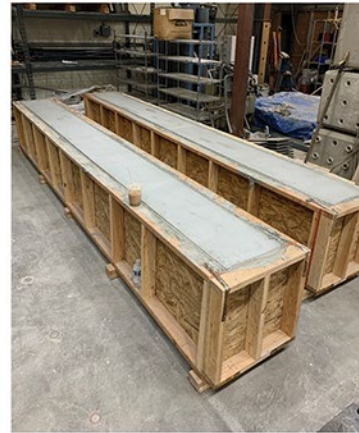
Large Beam Splice Tests (2) #8 Spliced Bars
