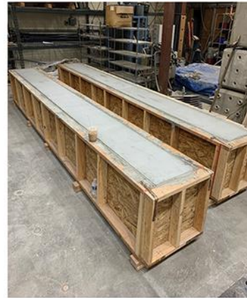
Large Beam Splice Tests (2) #8 Spliced Bars
