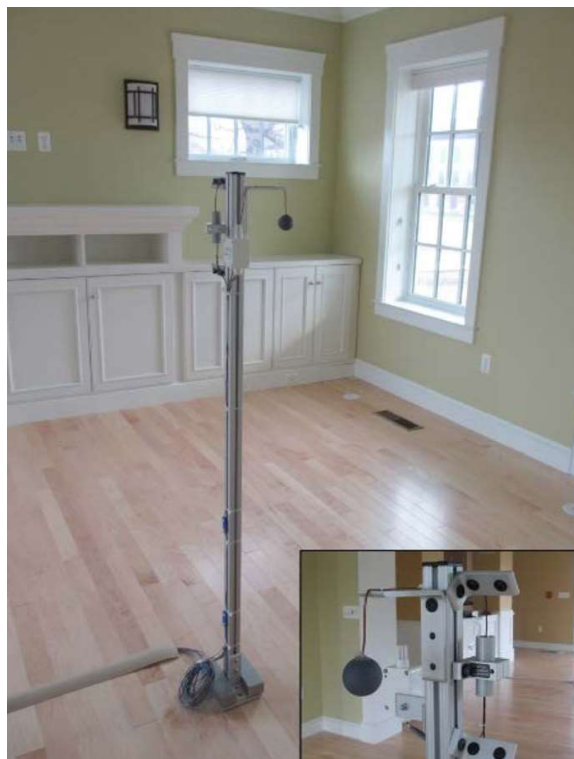
Figure 2: Sensors Mounted on the Metal Stand in the Center of the Room (Davis et al.).
