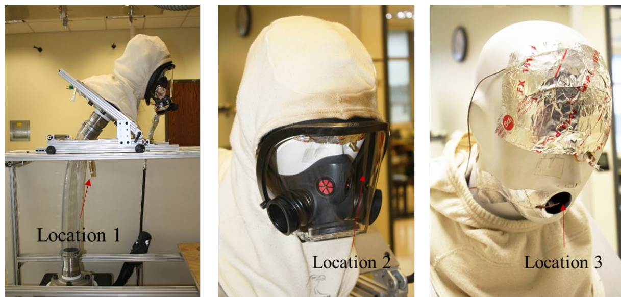
Figure 9. Sampling locations for gaseous injection in the GC-MS. Sampling in the airway (Location 1), between the SCBA lens and nose-cone (Location 2), and at the mouth (Location 3).
