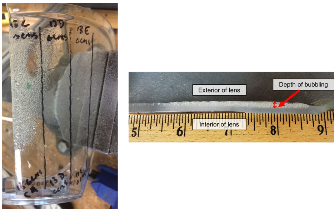
Figure 21. Damaged facepiece and cross-section showing damage only to exterior of facepiece.
