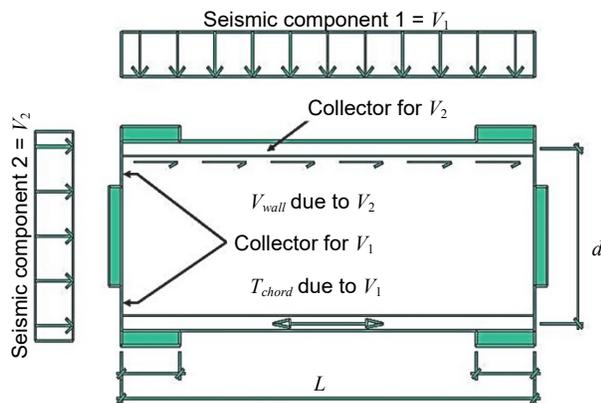
Figure 7-1. Diaphragm chords and collectors.
