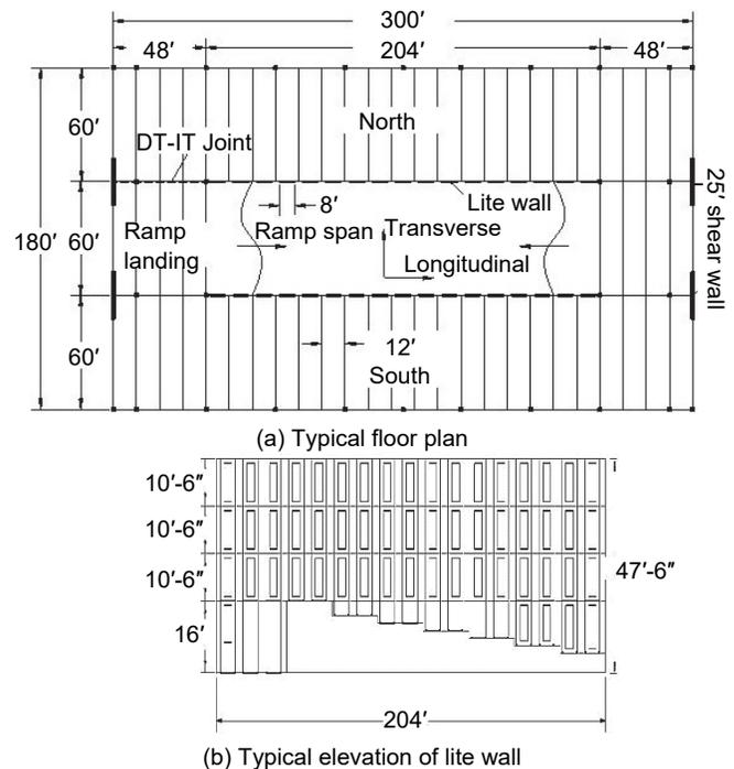
**Figure 4-4.** Example 1: Four-story perimeter shear wall precast concrete parking structure.
