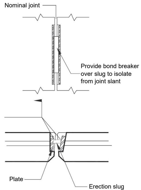
**Figure 2-8.** Welded chord connection detail, plan (top) and elevation (bottom).
