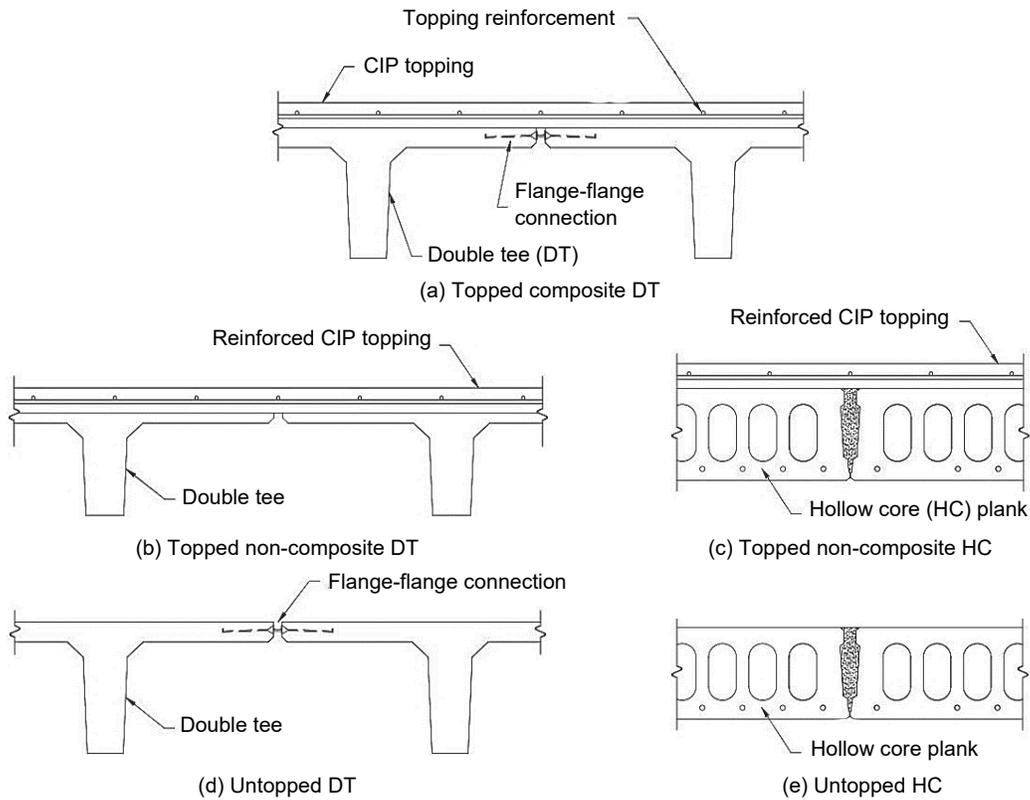
**Figure 2-4.** Double tee (DT) and hollow core (HC) configurations.
