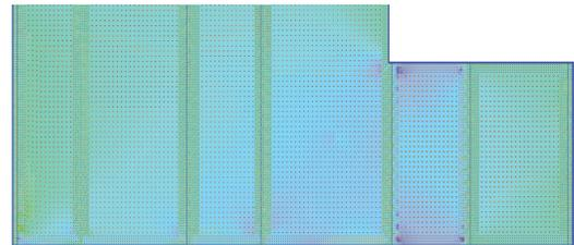
**Figure 5-6.** Detail of model output showing maximum principal stresses with darker color indicating increase at inside corner and extended sub-diaphragm.
