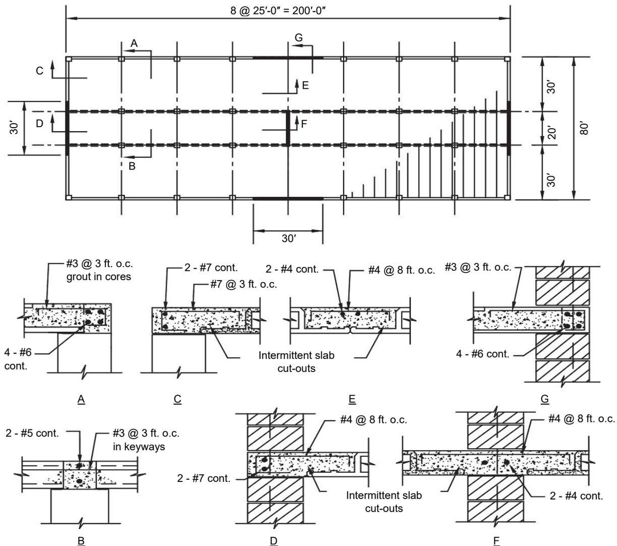
**Figure 2-9.** Typical chord details and shear friction reinforcement used for hollow core elements (PCI 2015).
