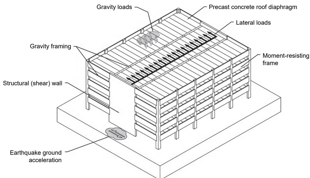
**Figure 1-1.** Building schematic showing SFERS elements including diaphragms.
