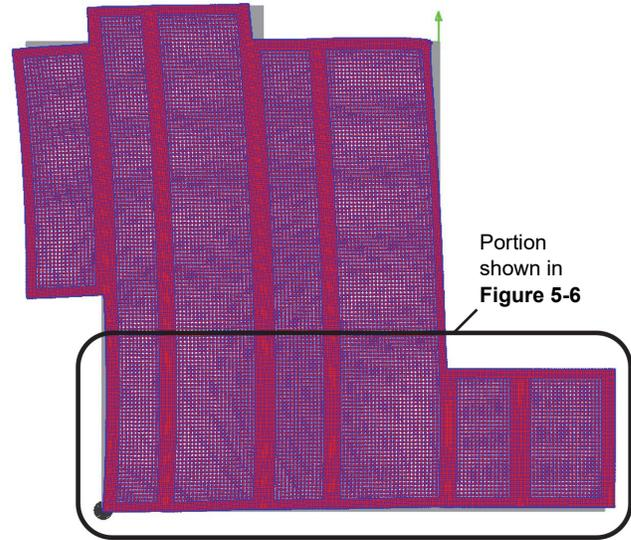
**Figure 5-5.** Deformed shape of finite element model representing the framing plan in Figure 5-3 for one direction of lateral loading.
