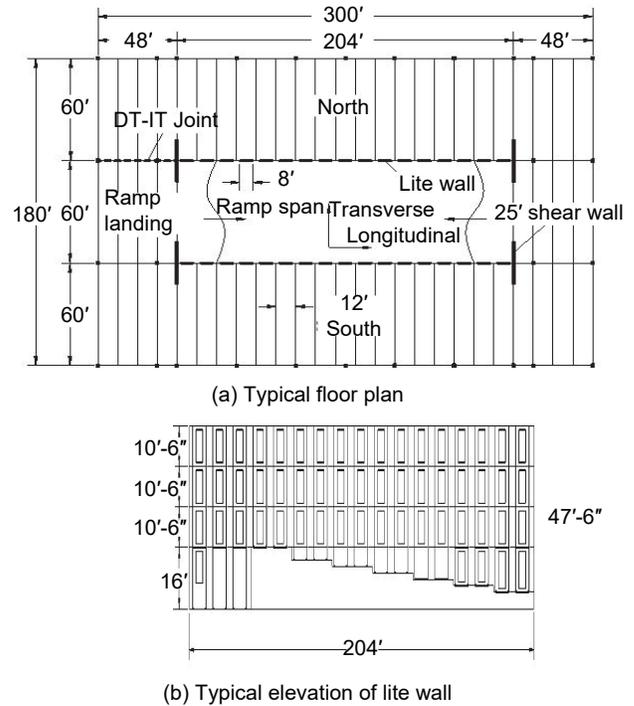
**Figure 4-6.** Example 2: Four-story interior shear wall precast concrete parking structure.
