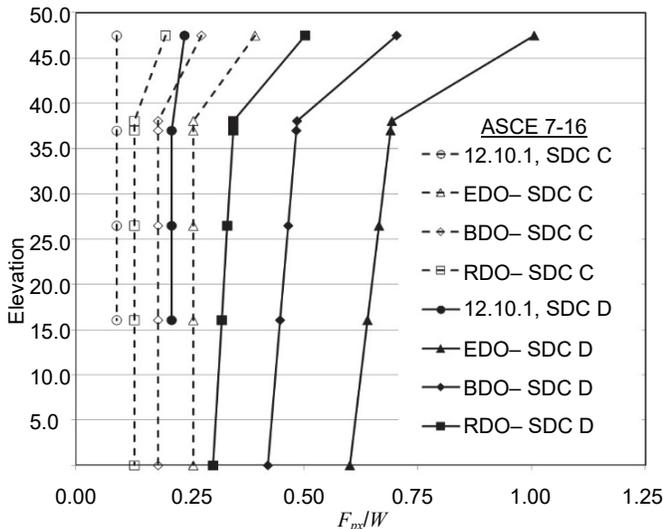
**Figure 4-5.** Design force level comparisons for Example 1 and 2 structures.
