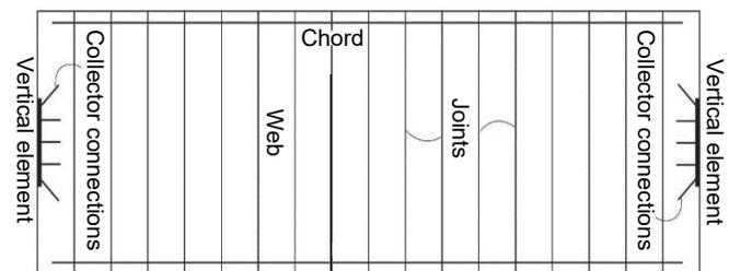
**Figure 5-1.** Diaphragm components according to beam analogy.
