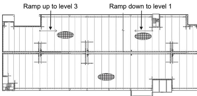
**Figure 2-7.** Topped diaphragm with chord reinforcement and topping reinforcement.
