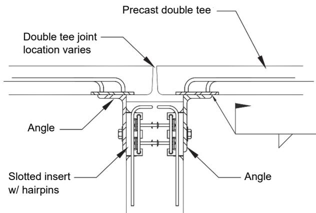
**Figure 2-11.** Sectional view of flange-to-wall connection under double tee flange using angle and slotted inserts.
