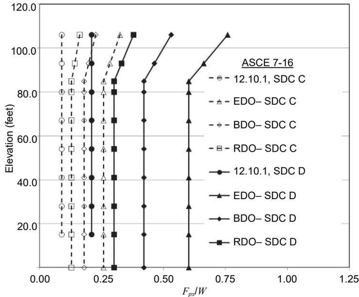
**Figure 4-8.** Design force level comparisons for Example 3 buildings designed for SDC C and D.
