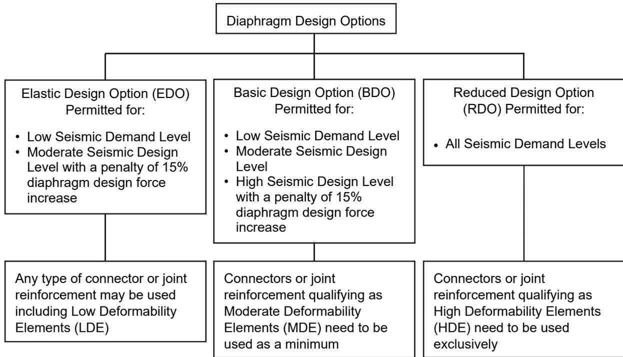
**Figure 6-2.** Diaphragm seismic design level – diaphragm design option – connector classification.
