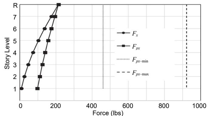
**Figure 4-2.** Distribution of  $F_x$  and  $F_{px}$  forces along the height of an example eight-story office building.
