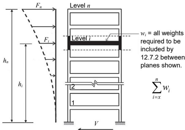
**Figure 4-1.** Seismic weights and lateral forces obtained from vertical distribution of design base shear at various floor levels (FEMA 2015).
