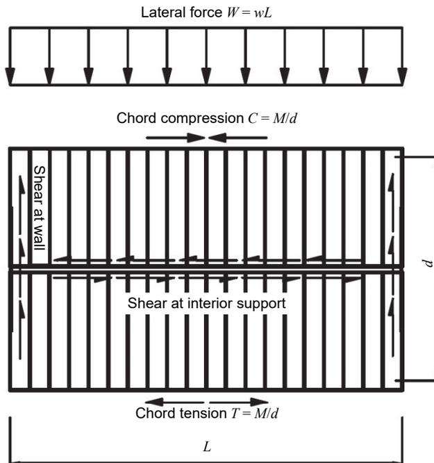
Figure 5-2. Diaphragm forces in a precast floor with multiple bays.
