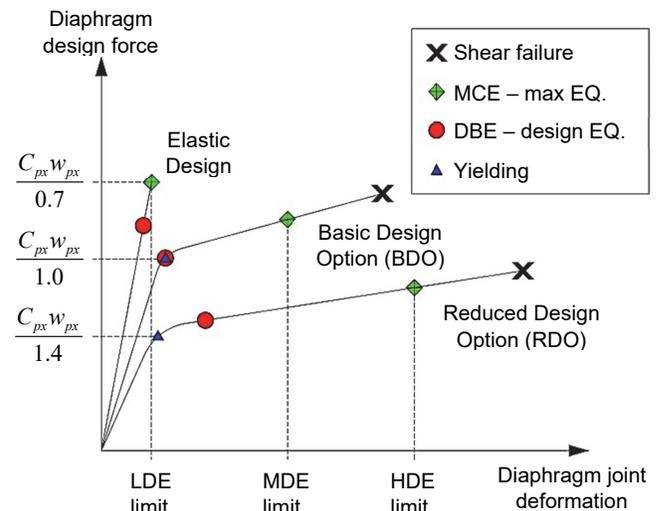
**Figure 8-1.** Diaphragm deformation relative to design option.
