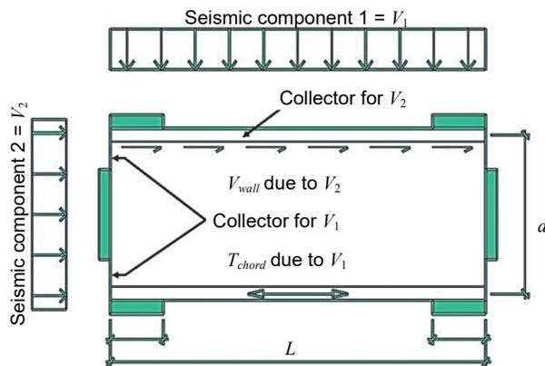
Figure 7-1. Diaphragm chords and collectors.
