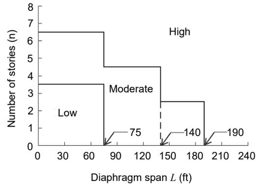
**Figure 6-1.** Diaphragm seismic demand level (ASCE/SEI 7-16 Figure 14.2-1, printed with permission from ASCE).
