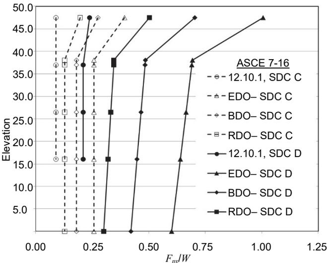
**Figure 4-5.** Design force level comparisons for Example 1 and 2 structures.
