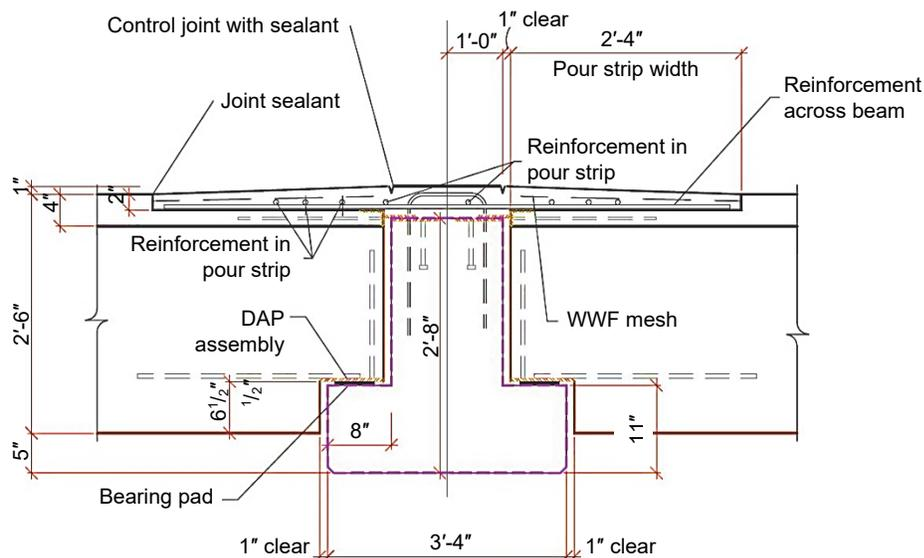
**Figure 2-13.** Section at inverted tee beam with composite concrete pour strip. DAP indicates dapped end.
