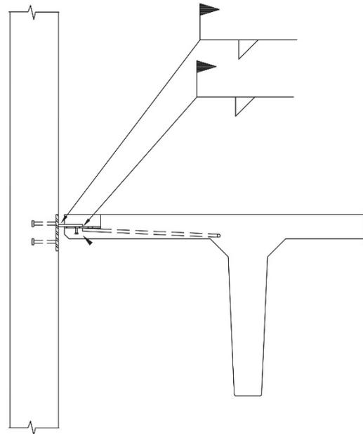
**Figure 2-12.** Flange-to-wall connection using welded plates and embedded plates with anchors.
