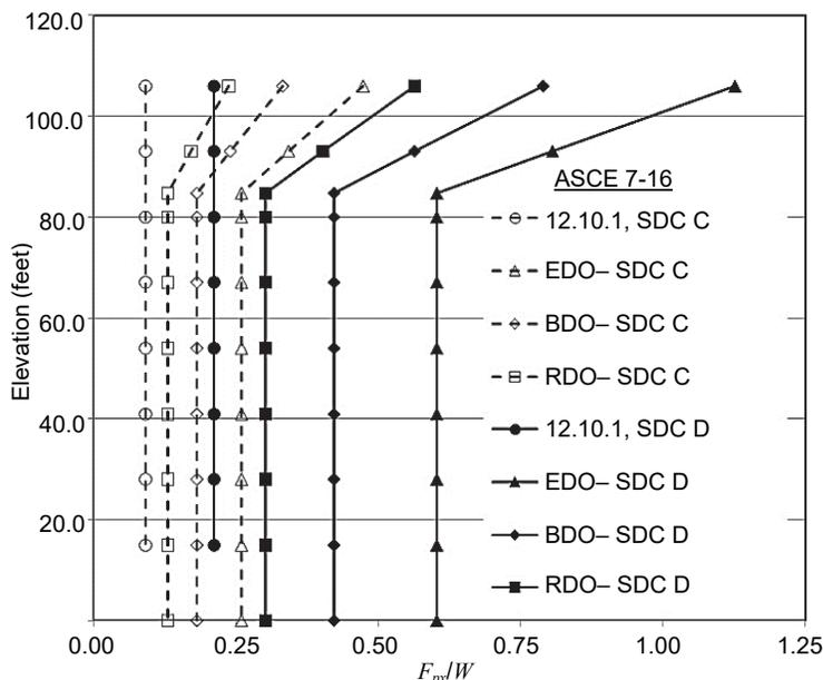
**Figure 4-10.** Design force level comparisons for Example 4 buildings designed for SDC C and D.
