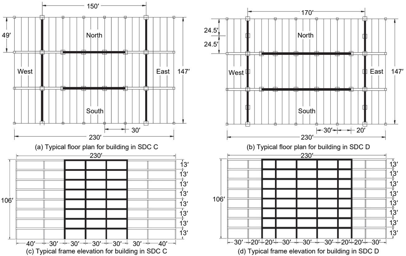
**Figure 4-7.** Example 3: 8-story moment resisting frame office building of precast concrete designed for SDC C and D.
