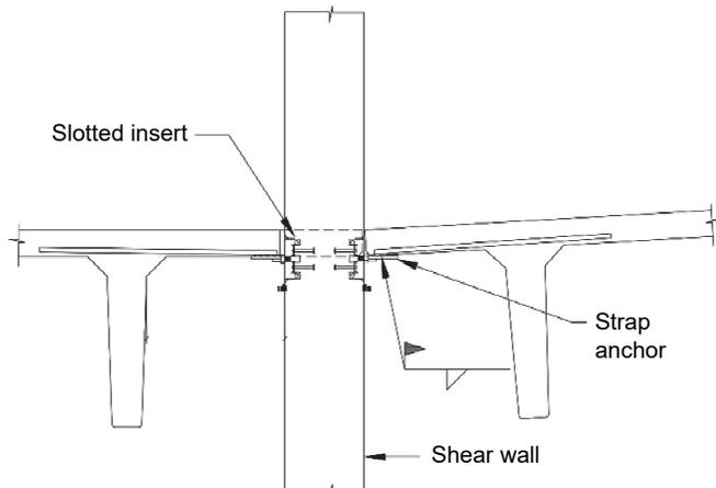
**Figure 2-10.** Flange-to-wall connection using strap anchors and slotted inserts.
