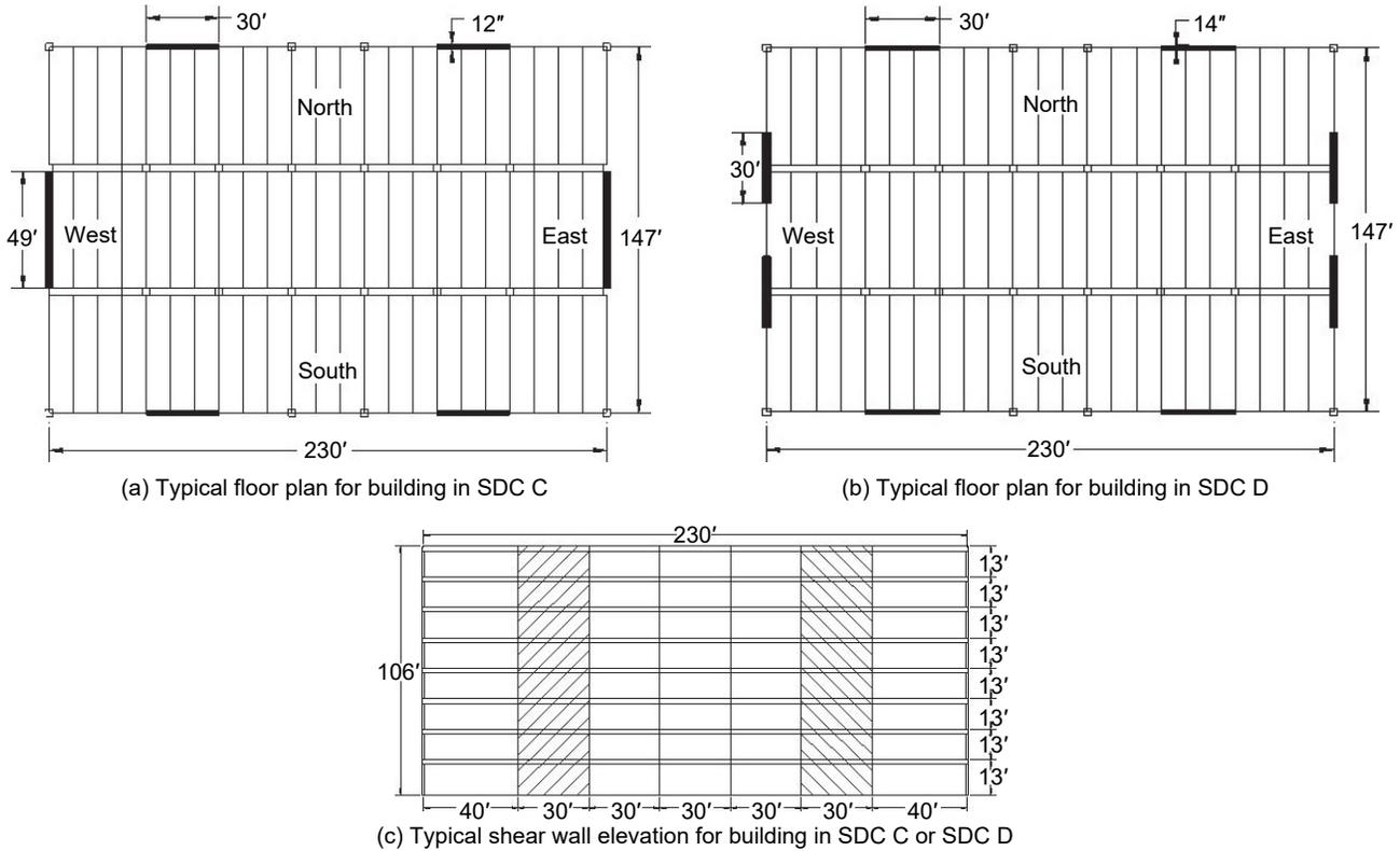
**Figure 4-9.** Example 4: Eight-story precast concrete shear wall office building designed for SDC C and D.
