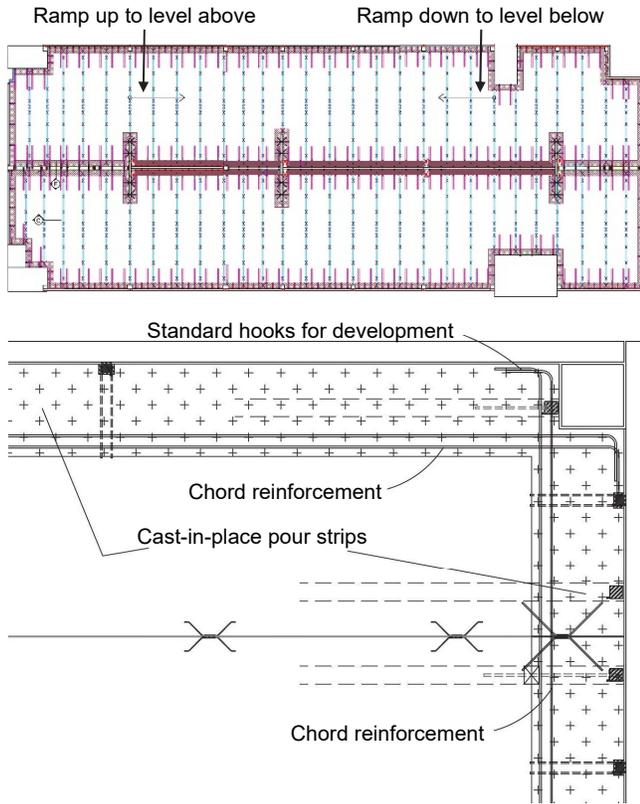
**Figure 2-6.** Untopped diaphragm with pour strips at ends of double tees and along perimeter.
