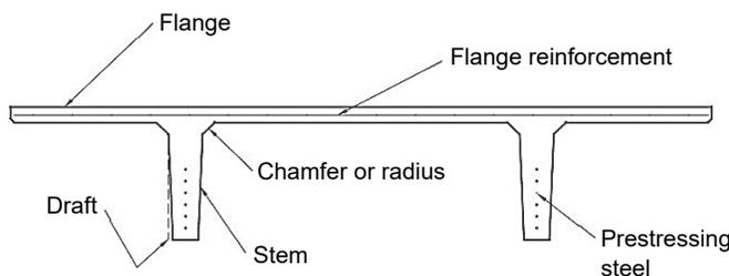
**Figure 2-2.** Double tee cross section with common terms for parts and features.
