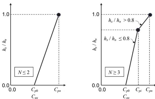
**Figure 4-3.** Calculating the design acceleration coefficient  $C_{px}$  in buildings two stories or less and in buildings three stories or more in height (values taken from ASCE/SEI 7-16 Figure 12.10-2).
