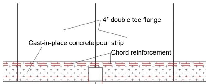
**Figure 9-2.** Pour strip at inboard exterior column.
