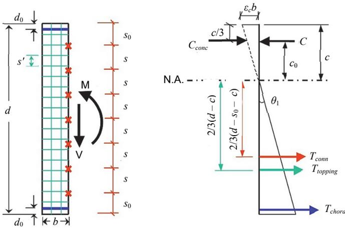
**Figure 7-3.** Free body diagram of a joint to determine effective section (Fleischman 2014).
