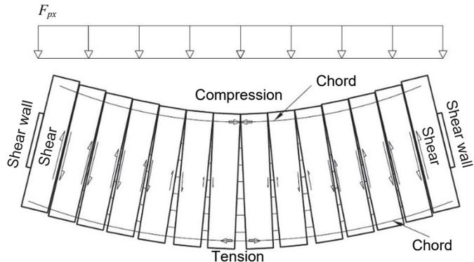
**Figure 2-5.** Beam analogy for precast diaphragm.
