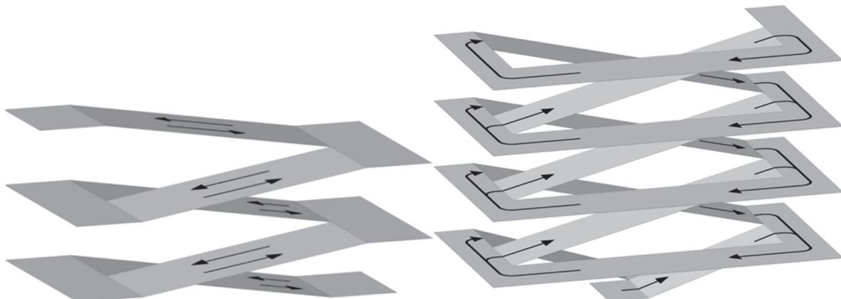
Figure 2-1. Single helix and double helix ramp configurations.
