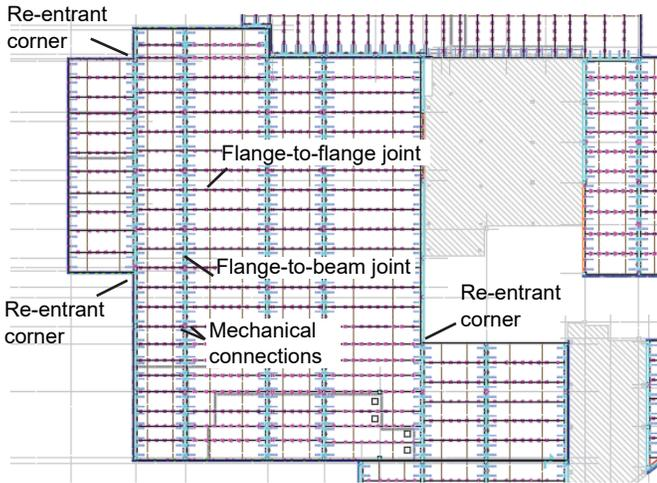
**Figure 5-3.** Partial framing plan of diaphragm.
