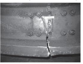
Figure 4-26 Weld fracture in welded column splice (Shaw, 2013).
