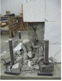
Figure 9-5 Crushing and bar buckling in a flexure-dominated wall (WSU-W-1A tested by Sherman, 2011).
