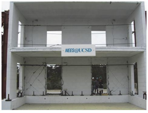
Figure 9-2 Shear failure of reinforced masonry walls in a three-story building tested on a shake table (Stavridis et al., 2016).
