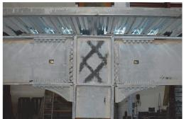
(a) Panel zone shear yielding(b) Panel zone shear bucklingFigure 4-23Typical hysteretic response of beam-to-column joint panel zone<br/>(Engelhardt et al., 2000; Newell and Uang, 2006b).
