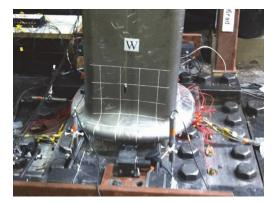
Figure 4-20 Elephant foot local buckling mechanism (Suzuki and Lignos, 2015).
