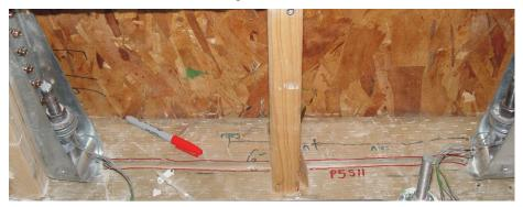
Figure 10-6 A <sup>1</sup>/<sub>2</sub>" wide sill plate split along a garage wall during a full scale building shake table test performed by Filiatrault et al. (2010).
