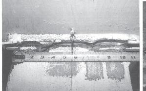
(a) Fracture across welded beam top flange
