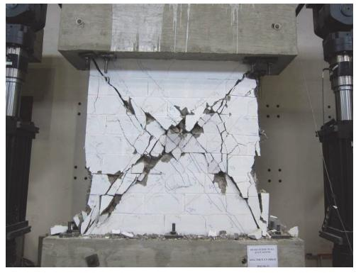
Figure 9-7 Failure of a shear-dominated wall (UT-PBS-02 tested by Ahmadi, 2012).
