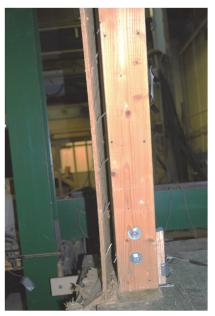
Figure 10-5 Sheathing rotating off resulting in complete loss of shear strength for the wood shear wall.
