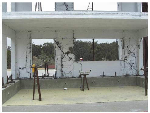
Figure 9-3 Shear failure of reinforced masonry piers in a two-story building tested on a shake table (Mavros et al., 2016).
