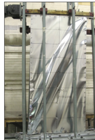
(f) Steel sheet shear wall exhibiting shear buckling during testing (adapted from Balh and Rogers 2010 Figure 2.18)
