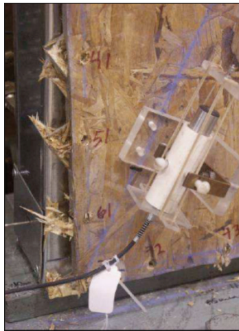
(b) Example of pull-through and edge tear-out at end of test (adapted from Hikita 2006 Figure 4-24)
