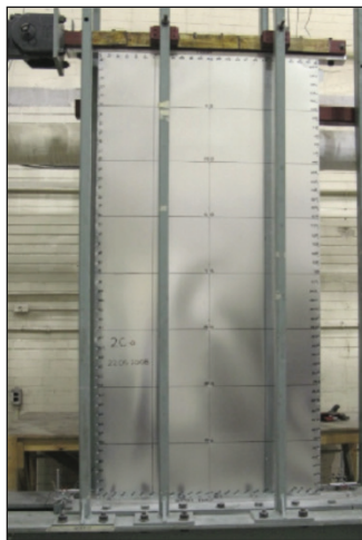
(e) Typical one-sided steel sheet sheathed specimen in test rig (adapted from Balh and Rogers 2010 Figure 2.17)
