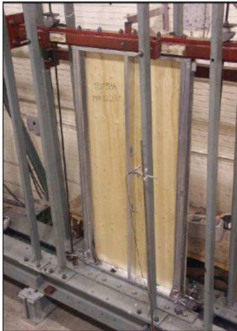
(a) Typical one-sided specimen in test rig (adapted from Hikita 2006 Figure 4-11)
