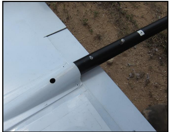
Figure 60: Insert the tail boom into the mounting guide on each wing.
