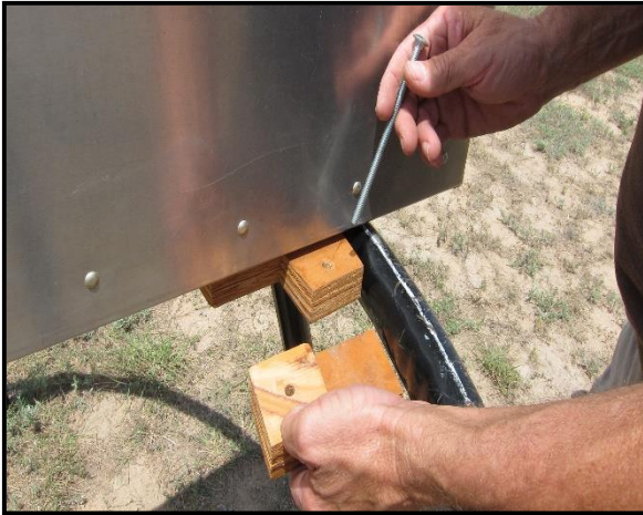
Figure 43: After the catapult, inside its transport housing, is in place; thread the support bracket carriage.
