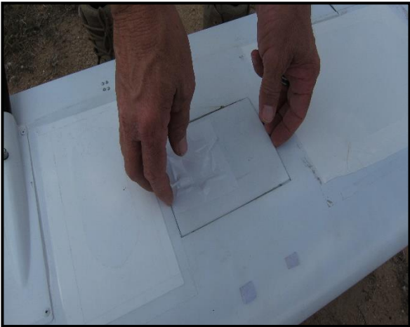
Figure 79: Locate and remove the wing camera bay cover.
