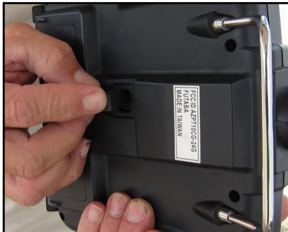
Figure 33: Firmly push the PIC GCS cable into the port of the PIC transmitter. Secure the cable to the transmitter via Velcro wrap or zip tie to insure cable does not disengage during flight operations.
