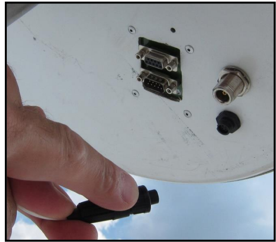
Figure 13: Attach the power cable to both units first.
