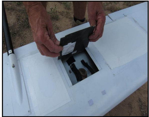
Figure 80: Once the cover is removed the mounting bay is exposed.
