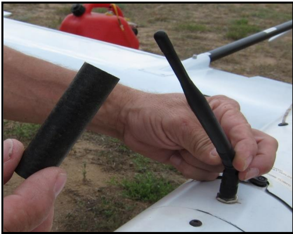
Figure 75: Place the carbon fiber collar over the telemetry antenna.
