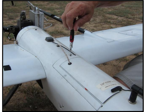
Figure 72: Replace the parachute bay securing screw and tighten.
