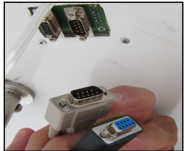
Figure 15: There are two serial connectors per radome. One is for primary tracking and the second cable attaches the units together.
