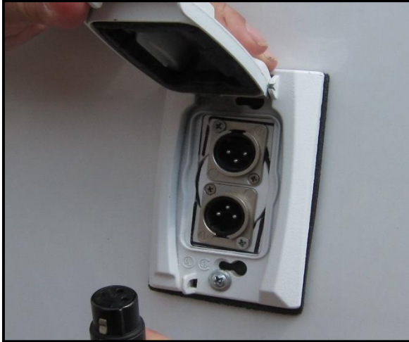
Figure 28: Locate the dual XLR bulkhead cable port on the trailer exterior.
