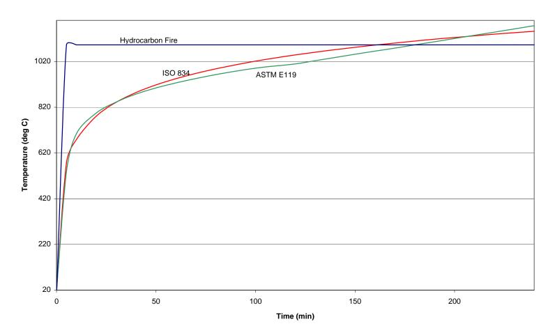
Figure 3.1 Fire Exposure Conditions
