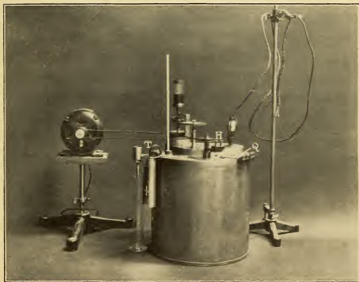
FIG. 4.—Assembled calorimeter B. S. 7602, showing stirring motor and calorimetric resistance thermometer
