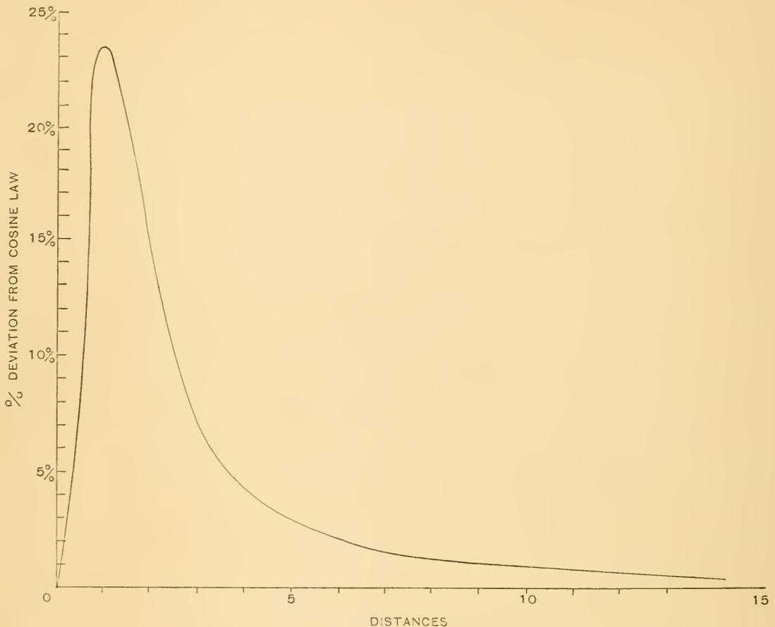
Fig. 9.—*Deviation of Radiation of Infinite Strip from Cosine Law. (45°).*
