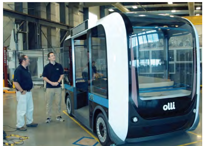
Figure 34. Additive manufacturing was used to produce Local Motors' first self-driving vehicle. Credit: IACMI
