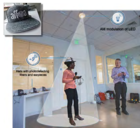
Figure 28. AFFOA-developed LiFi receivers have detectors woven into cap fibers that convert modulated light into audio signals. Credit: AFFOA
