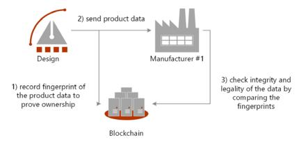
Fig. 3. Using a blockchain ledger to check product data integrity in a simple environment
