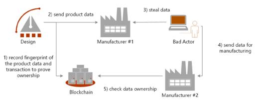
Fig. 4. Using a blockchain ledger to check product data ownership in a complex environment
