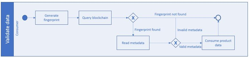
Fig. 12. Validating a transaction using the blockchain
