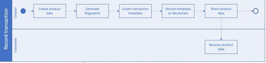
Fig. 11. Recording a transaction on the blockchain
