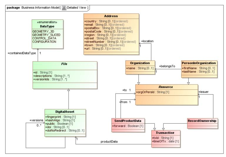
Fig. 6. Reference model for blockchain-based product data traceability
