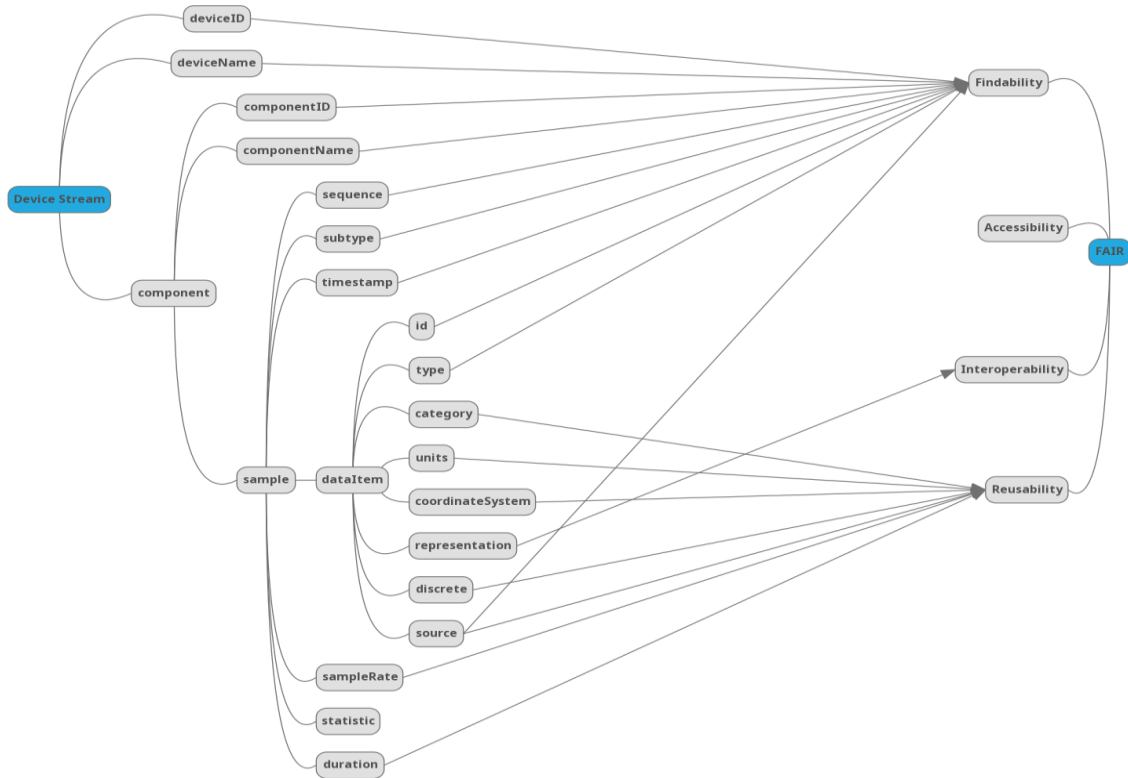
Figure 26: MTConnect data model mapping to the FAIR stack
