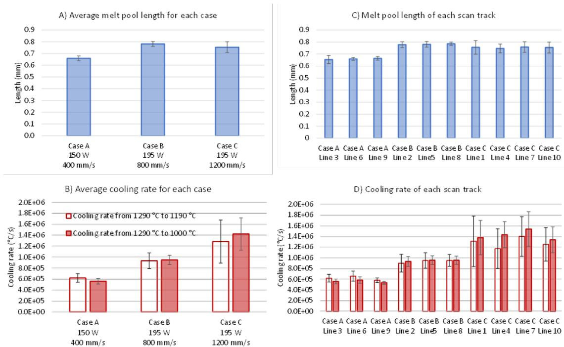
**Fig. 2** - The average melt pool length and cooling rate results from each scan line and each case.
