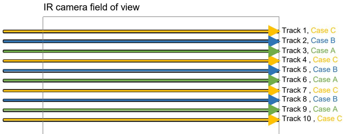
**Fig. 1** - Arrangement of the 10 scan tracks within the field of view of the IR camera. Note that this is slightly different than was originally proposed <https://www.nist.gov/ambench/amb2018-02-description>.
