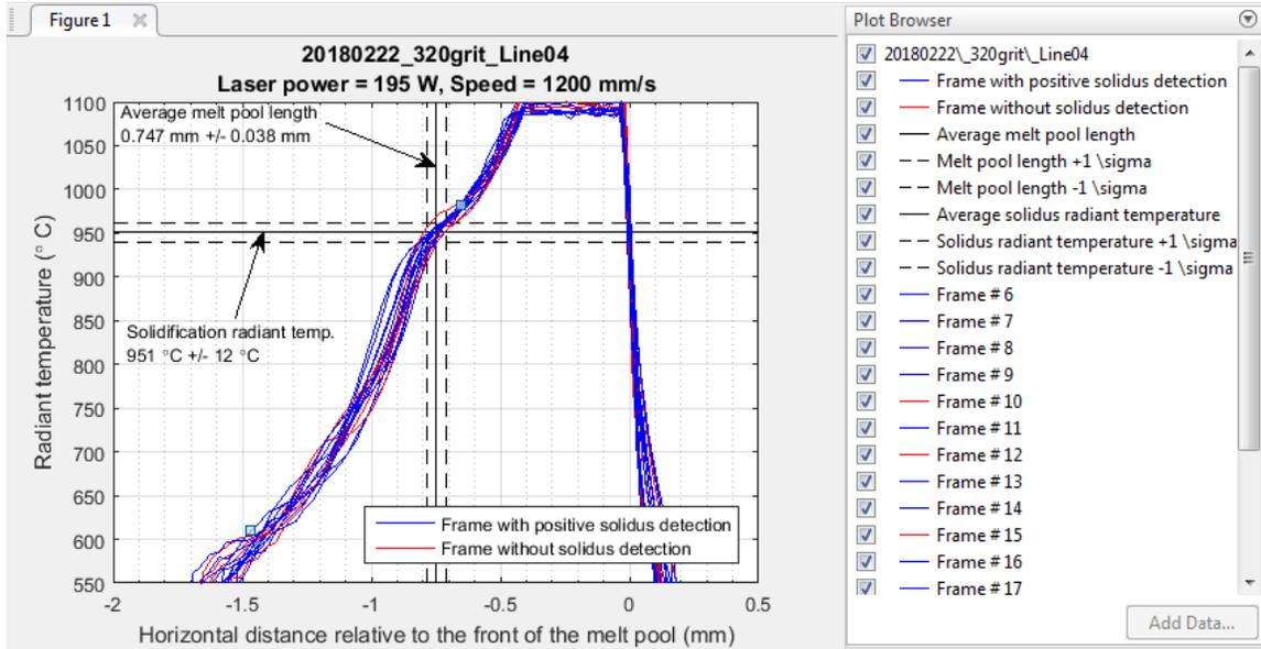
Fig. 4 - Demonstration of the radiant temperature profiles available in TemperatureProfilePlots.zip.
