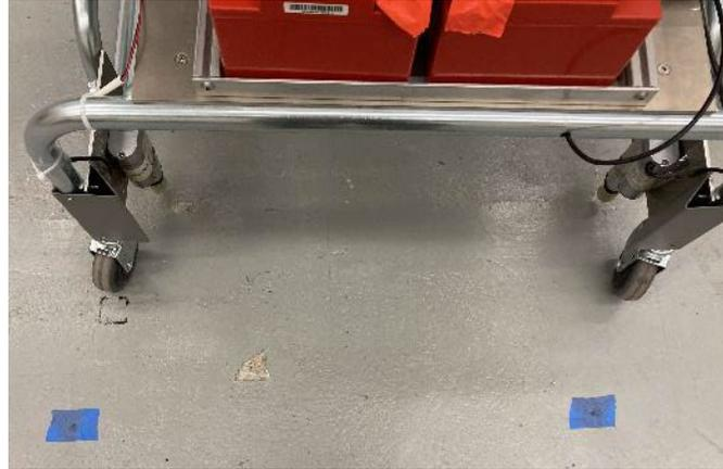
**Fig. 20.** Marked tape used to manually re-center the cart position between trials for run 2.
