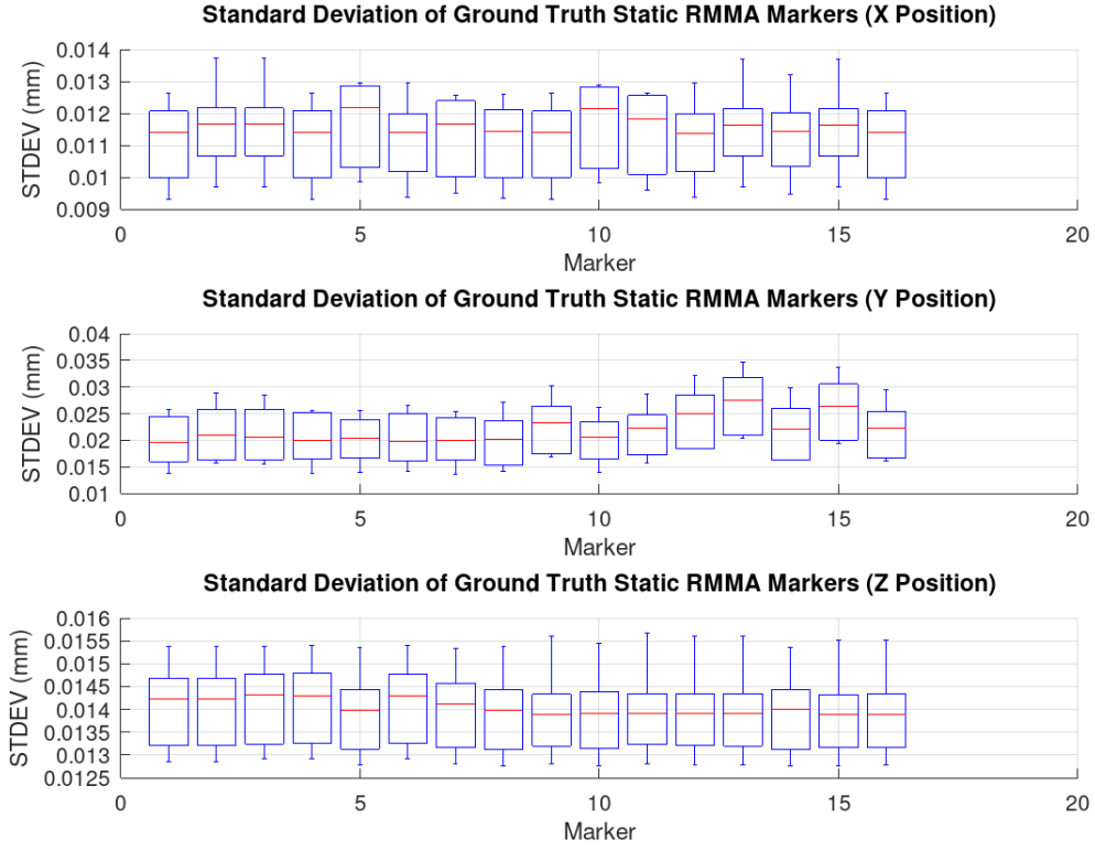
Fig. 13. Boxplots of the standard deviation marker position components for static ground truth RMMA measurements ('+' - Potential Outlier, 'O' - Outlier).
