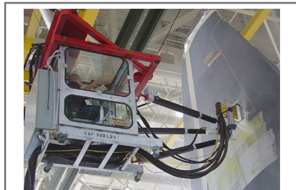
A worker in a protective cab on a NIST-developed revolutionary robotic platform strips paint off a U.S. Air Force C-130. The easily maneuverable platform uses computer-controlled cables to 'float' around the aircraft to reduce paint-stripping time per airplane, cut maintenance costs and lessen incidents of operator stress and injury.
