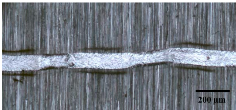
Fig. 5. Non-straight stainless-steel single track on the substrate. Samples manufactured using experimental testbed set-up by NIST.
