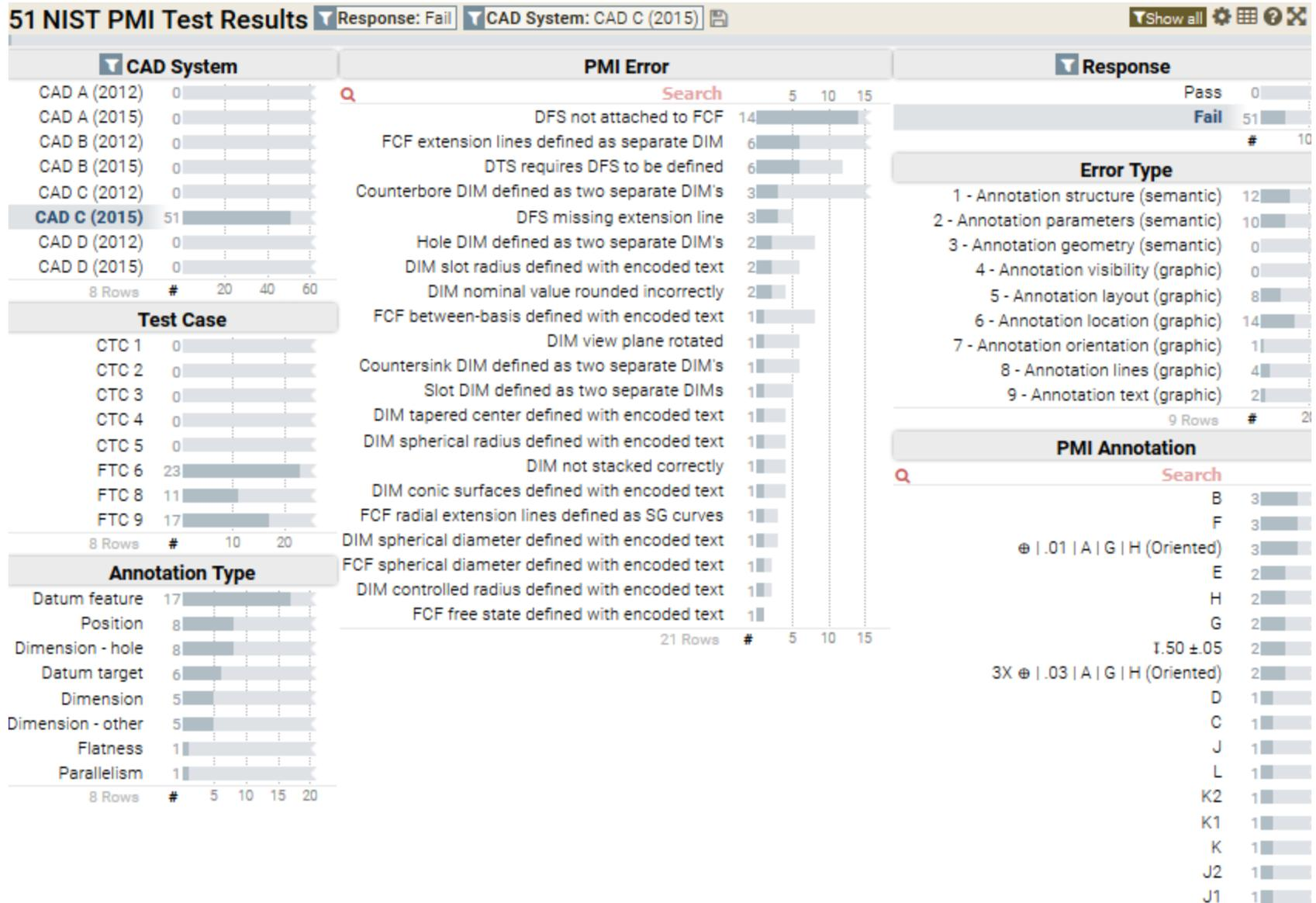
Figure 34: PMI errors for CAD system C (2015 version)
