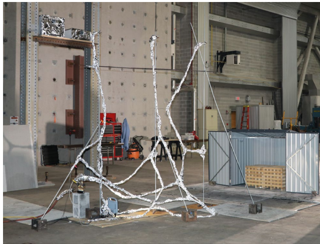
Fig. 51. Three heat flux gauge stands in front of the shed.
