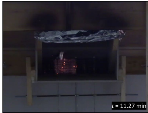
Flames through vent (11.27 min)
