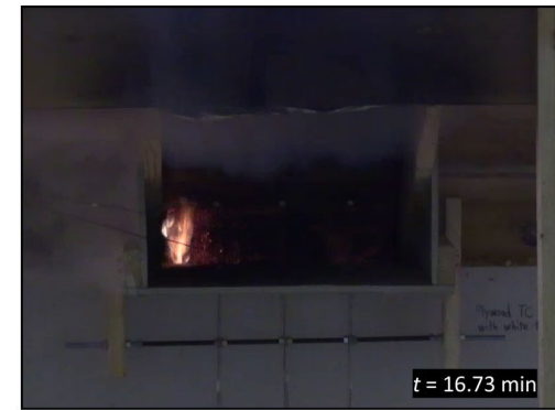
Flames through vent (16.73 min)
