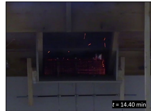
Flames through vent (14.40 min)
