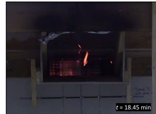
Flames through vent (18.45 min)
