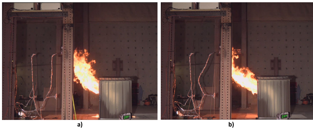
Fig. 54. Side view of experiments p2 and p6 at approximately maximum HRR.
