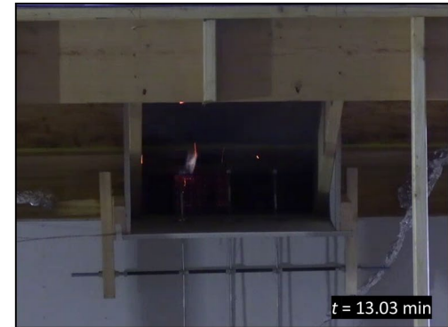
Flames through vent (13.03 min)
