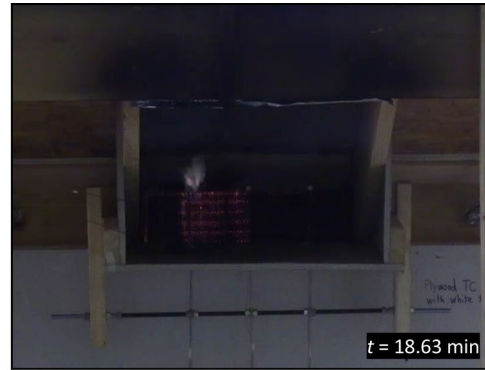
Flames through vent (18.63 min)
