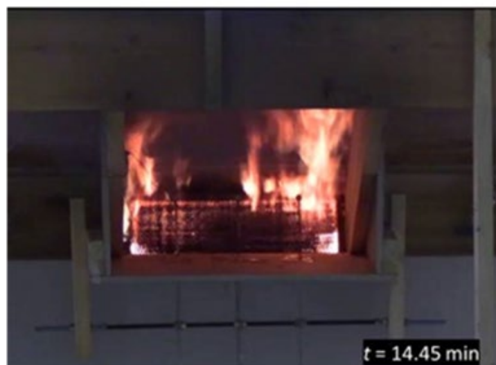
Fig. 26. Interior vent image showing flame penetration through the vent into the attic side following eave ignition during e10.
