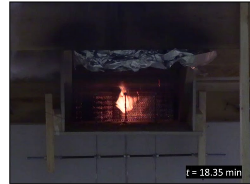
Flames through vent (18.35 min)
