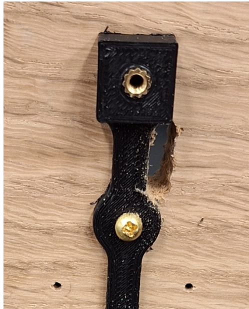
Figure 8: Cutout in the wood board for the connector on the 4-wire cable, which connects the control panel with the Arduino Shield board. Although a milling machine could be used, a few holes drilled with a hand drill and connected manually work well enough.
