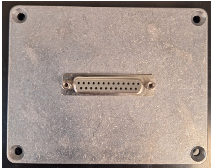
Figure 3: Diecast aluminum enclosure with 25-pin DSUB connector and hex standoffs that thread into the lid.
