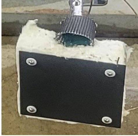
Figure 4. A photo of the front of the 10 cm x 10 cm modified plate thermometer.
