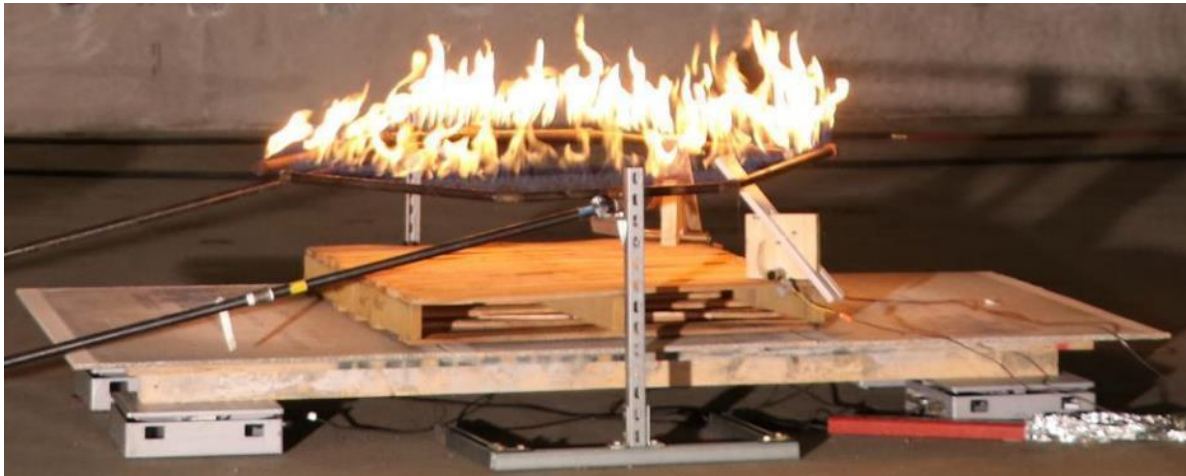
Figure 9. The early version of the burner with flames ignited.
