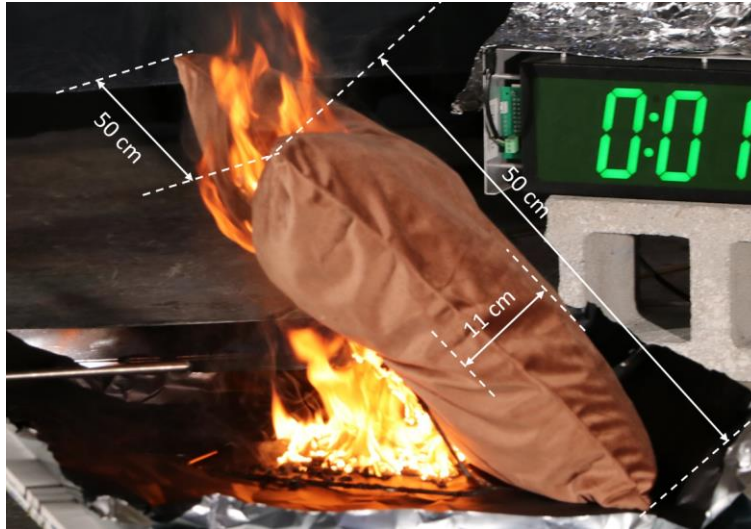
Figure A7. Test 7 photo with dimensions of Pillow A.
