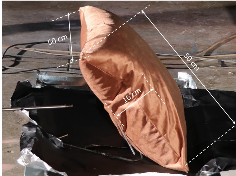
Figure A5. Test 5 photo with dimensions of Pillow E.
