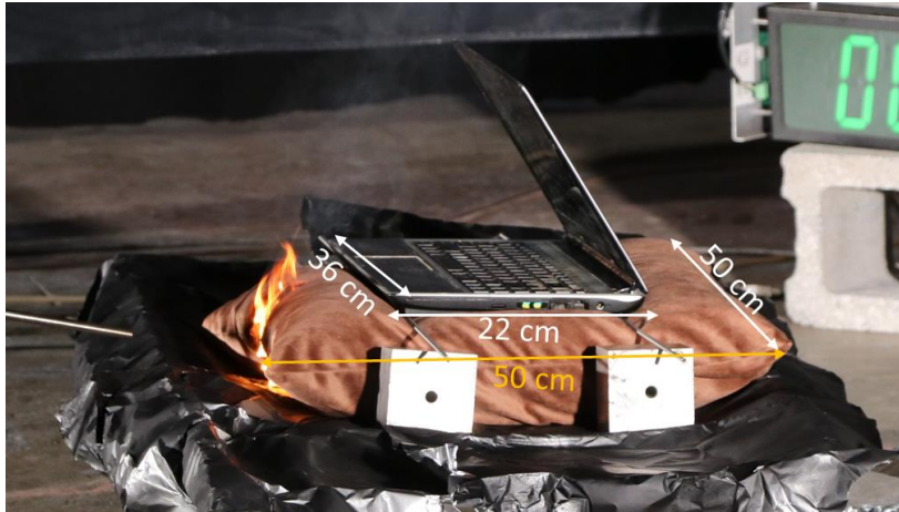
Figure A15. Test 15 photo with dimensions of Laptop B folded at 45 degrees after ignition of the front of Pillow A.
