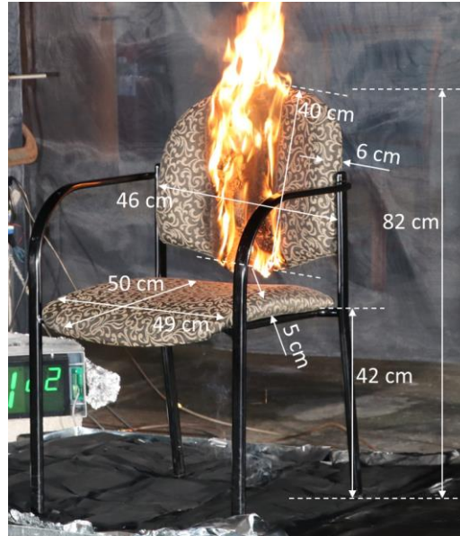
Figure A20. Test 20 photo with dimensions of Chair D.
