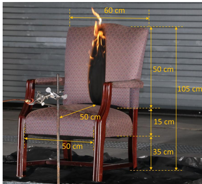
Figure A22. Test 22 photo with dimensions of large desk armchair E.
