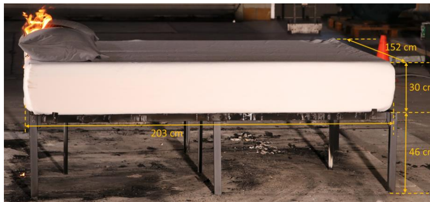
Figure A32. Test 32 photo with dimensions of Mattress C with two D pillows.
