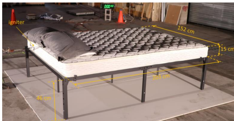
Figure A26. Test 26 photo with dimensions of Mattress A with two D pillows.
