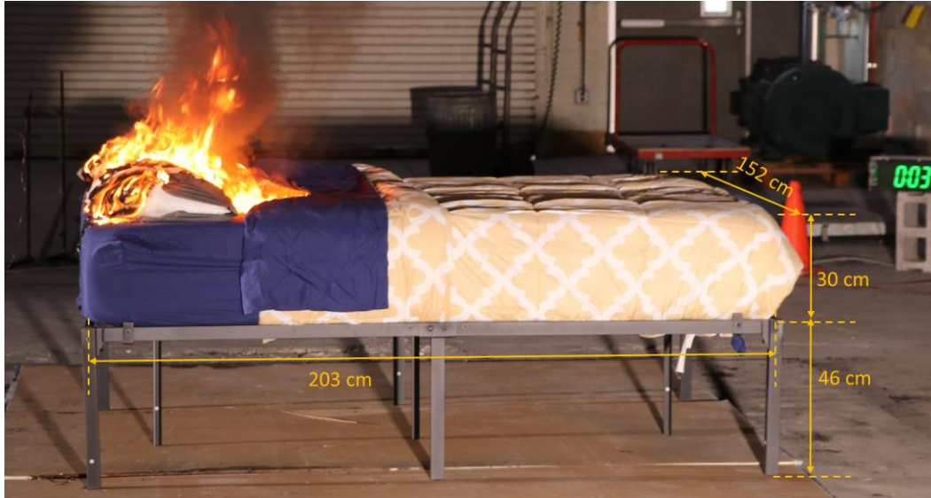
Figure A38. Test 38 photo with dimensions of Mattress C with two D pillows and bedclothes.
