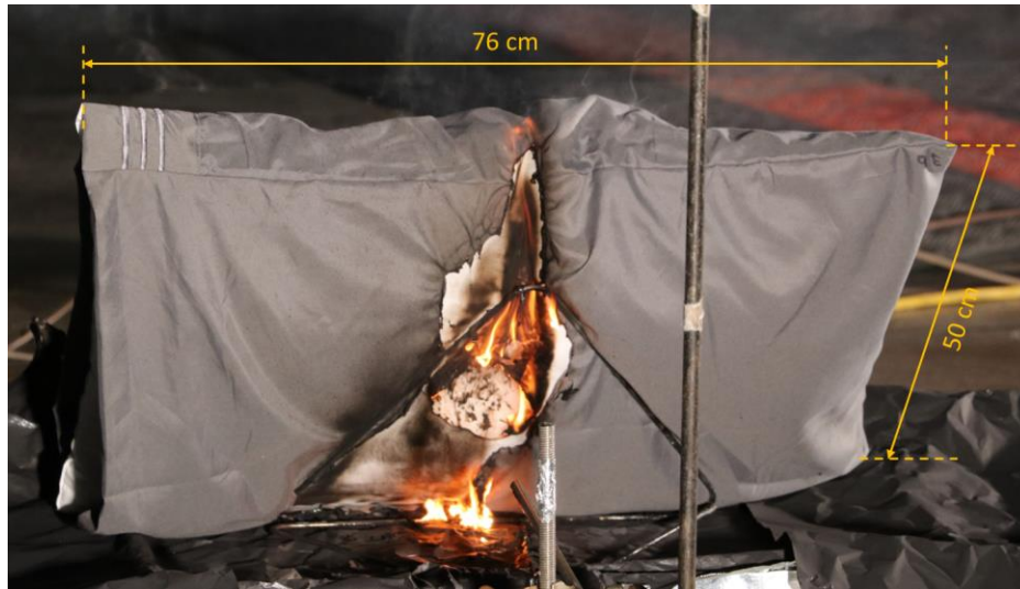
Figure A11. Test 11 photo with dimensions of Pillow D.
