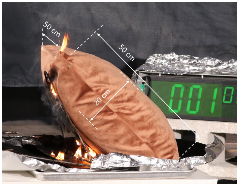
Figure A2. Test 2 photo with dimensions of Pillow B.
