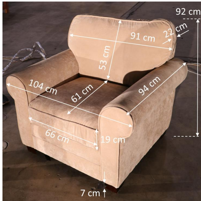
Figure A27. Test 27 photo with dimensions of large armchair H composed of a wood frame, PUF cushions, metal springs, and thin fiberglass cloth.
