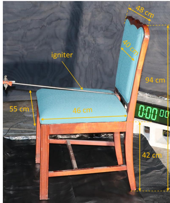
Figure A17. Test 17 photo with dimensions of Chair B.
