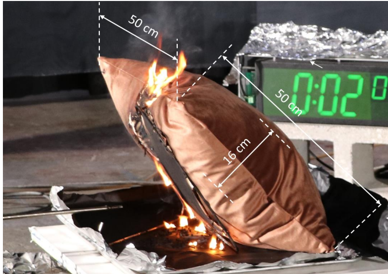
Figure A3. Test 3 photo with dimensions of Pillow C.
