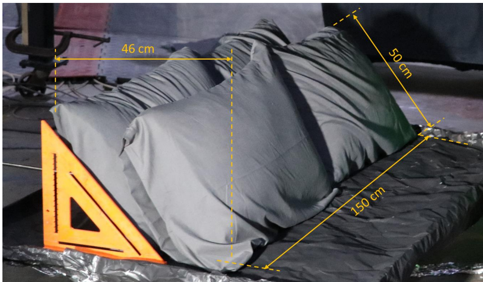
Figure A10. Test 10 photo with dimensions of four D pillows.
