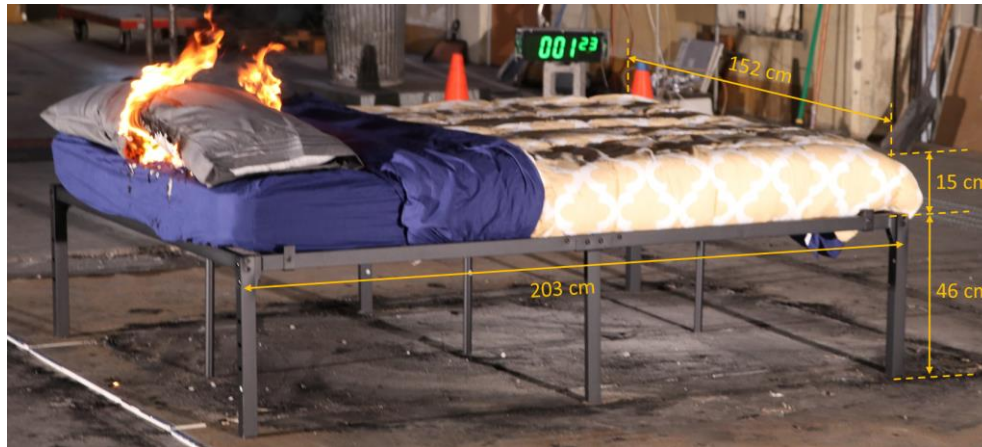
Figure A39. Test 39 photo with dimensions of Mattress A with two D pillows, bedclothes, and a mattress topper.
