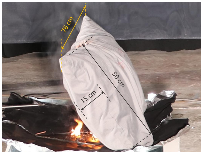
Figure A4. Test 4 photo with dimensions of Pillow D.
