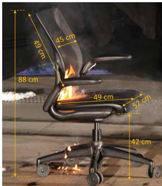
Figure A48. Test 48 photo with dimensions of wheeled office Chair K.
