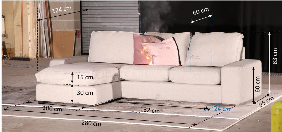
Figure A36. Test 36 photo with dimensions of chaise Sofa B with two A pillows on the middle of the sofa.
