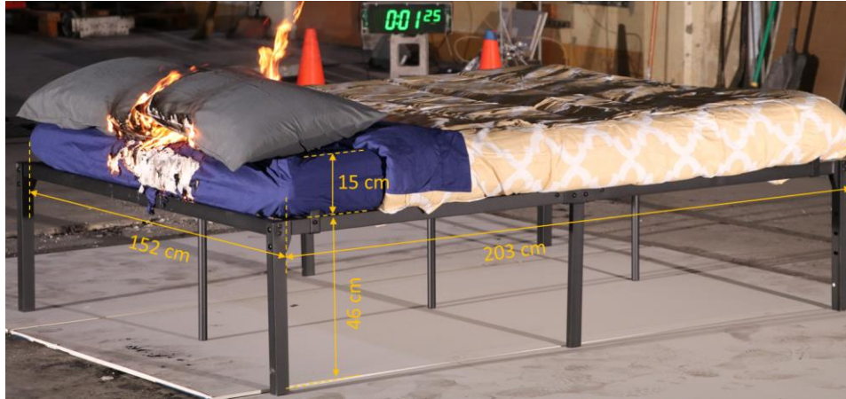
Figure A37. Test 37 photo with dimensions of Mattress B with two D pillows and bedclothes.
