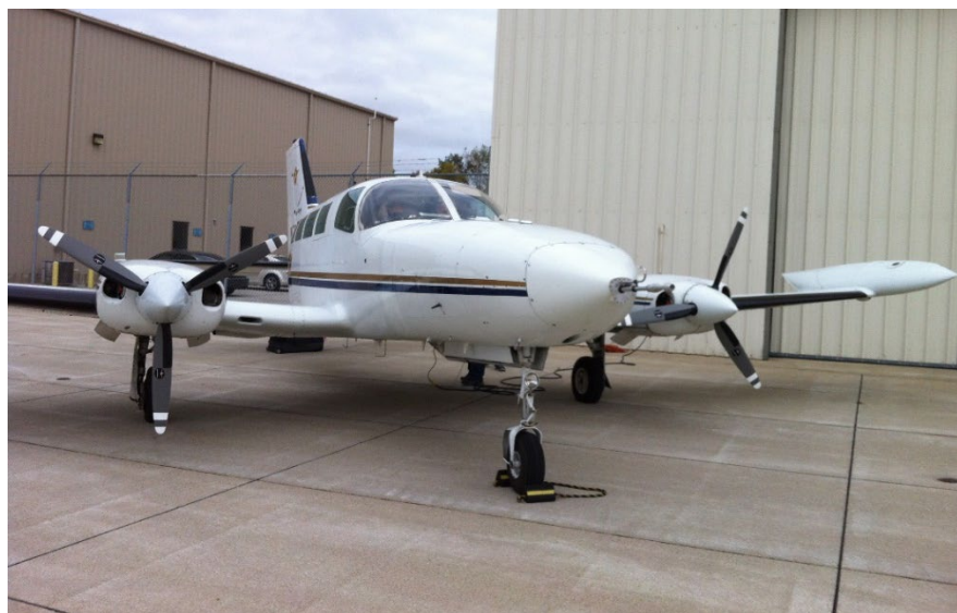
Figure 23. University of Maryland experimental Cessna 402B research aircraft used for airborne mass balance experiments. www2.atmos.umd.edu/~flaggmd/
