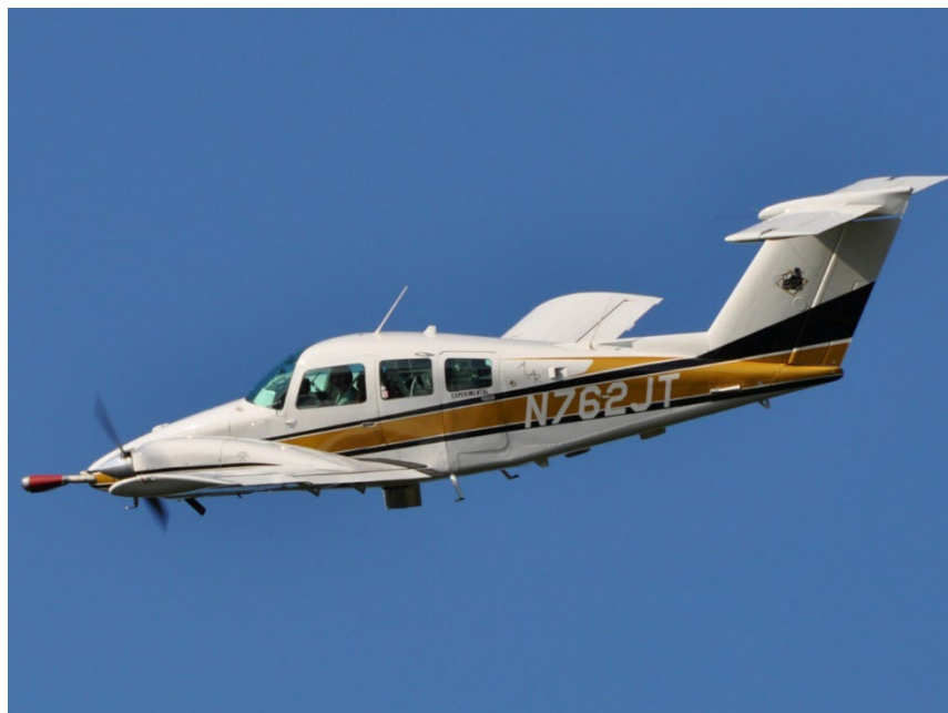
Figure 15. Instrumented Beechcraft BE76 Duchess aircraft that serves as Purdue University's Airborne Laboratory Atmospheric Research (ALAR)
