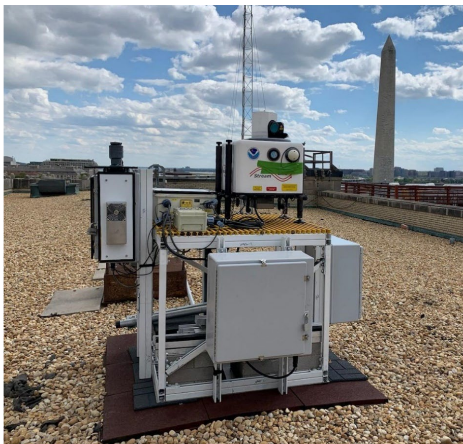
Figure 28. NOAA and NIST installed a Doppler LIDAR instrument on top of the Department of Commerce's Herbert Clark Hoover Building in Washington, D.C. on April 16, 2021, for a research project studying urban greenhouse gas emissions.
