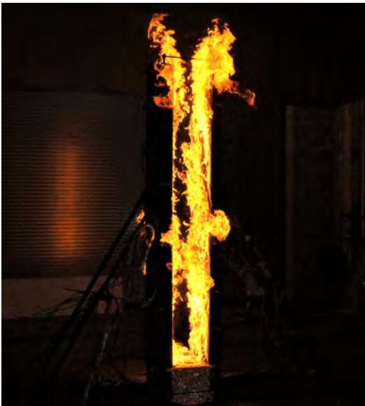
(c) Near first peak in HRR, \dot{Q} = 500 kW
