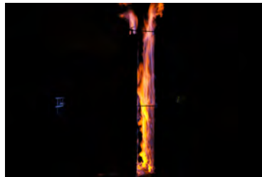
(e) Flame sheet covering full surface of left panel wall in Test R3 near peak burning, \dot{Q} > 450 kW ( t = 650 s)
