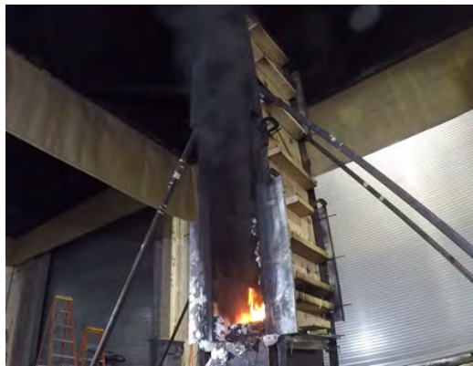
(c) Continued burning of (and heavy soot formation) charred sample remnants at the base of panels, towards the end of a test
