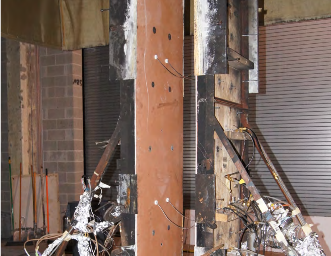
Fig. 5. Photograph of GPO-1 prior to testing showing mounting, support, and shielded of heat flux gauges. Here, each panel wall is instrumented with heat flux gauges; on the left wall, two gauges at each height z = 100 cm and z = 180 cm are shielded by 2.54 cm diameter insulation discs to ensure clean gauge readings of \dot{q}_{\text{rad}}'' and \dot{q}_{\text{total}}'' .
