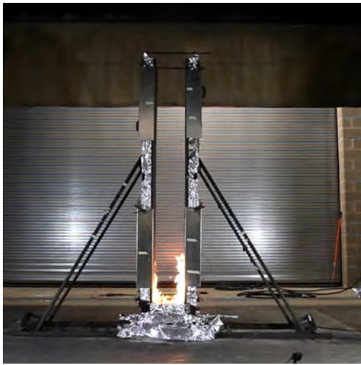
(a) Test XLPE2_R1 showing preferential flame attachment to the right wall ( x = 15 cm)
