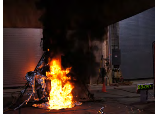
(d) Continued burning and heavy soot formation of pool fire
