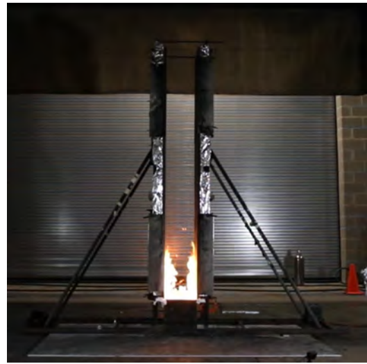
(b) Test XLPE2_R2 showing uniform flame attachment to both panel walls
