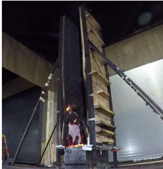
(c) Nominal thickness = 2.0 in., unburnt sample visible at backside of panels away from burner
