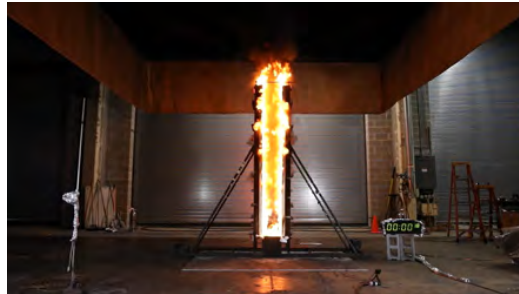
(c) Nominal thickness = 2.0 in., \dot{Q} = 0.80 MW
