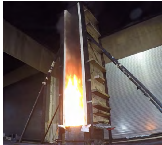
(b) Initial flame height seconds after ignition of 2.0 in. thick polyiso samples
