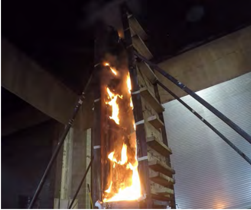
(a) Nominal thickness = 0.5 in., complete burnout and fragmentation of residue
