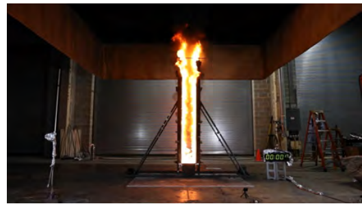
(b) Nominal thickness = 1.0 in., \dot{Q} = 0.97 MW
