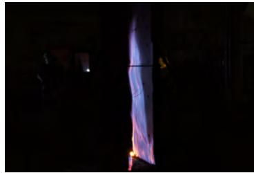
(b) Flame sheet covering left panel wall in Test R3, showing transparent blue flame ( t = 280 s)
