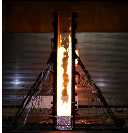
(b) Early flame spread, \dot{Q} = 300 kW
