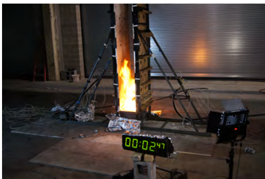
(a) Ignition of base of panel walls, just prior to burner shutoff
