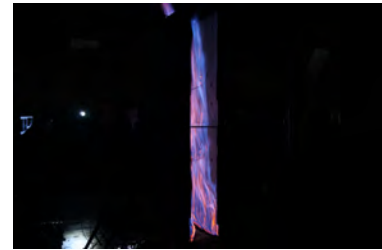
(c) Flame sheet covering base of left panel wall in Test R3; still primarily transparent, and reaching the top of assembly ( t = 438 s)
