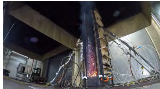
(d) Extinction shortly after burner shutoff: charring at the front surface of samples and smoldering combustion near the burner
