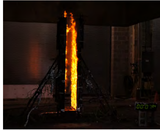
(b) Flame spread, \dot{Q} = 165 kW
