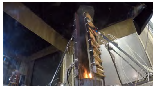
(b) After 20 min. exposure to 63 kW burner
