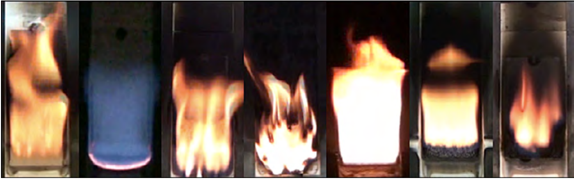
Fig. 4. Representative behavior of laminar wall flames supported by six common commodity plastics: (from left to right) PMMA, POM-GF, HIPS, ABS, PBT (reinforced with 20 wt. % chopped glass fibers), and fiberglass-reinforced polyester.
