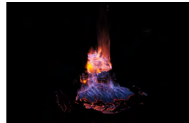
(f) Continued burning of melted POM-GF at the front base of panels, towards the end of Test R3 ( t = 1474 s)
