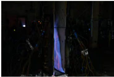
(a) Initial flame height shortly after the sample is ignited and the burner is covered in Test R3 ( t = 194 s).
