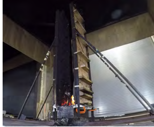
(b) Nominal thickness = 1.0 in., near complete burnout, residue mostly in tact
