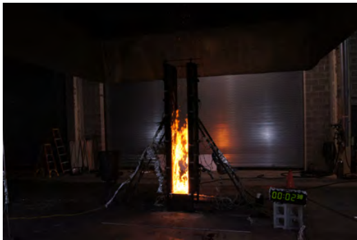
(c) Charring at the front surface of samples (top) and continued flaming (bottom, near burner) at time, t = 160 \text{ s} after ignition
