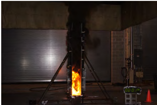
(a) Ignition of panel walls, approximately 90 s after burner exposure
