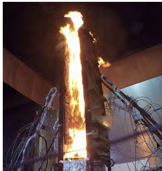
(d) Decay: Local burnout, smoldering (glowing combustion) of charred panels, and continued flaming of remaining sample remnants
