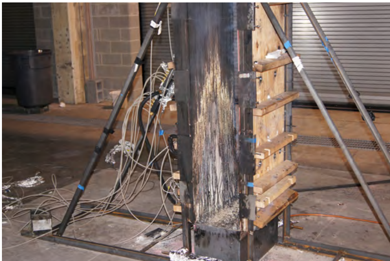
(c) Burnout at base of panels after 25 minute burner exposure
