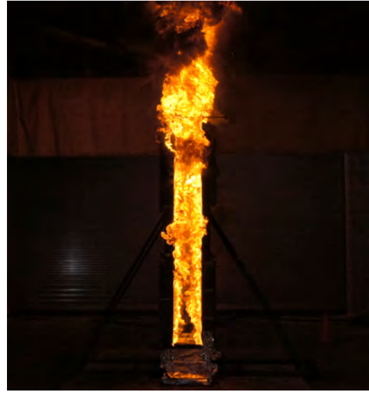
(b) Flame spread 60 s after sample ignition; \dot{Q} = 2.5 \text{ MW}
