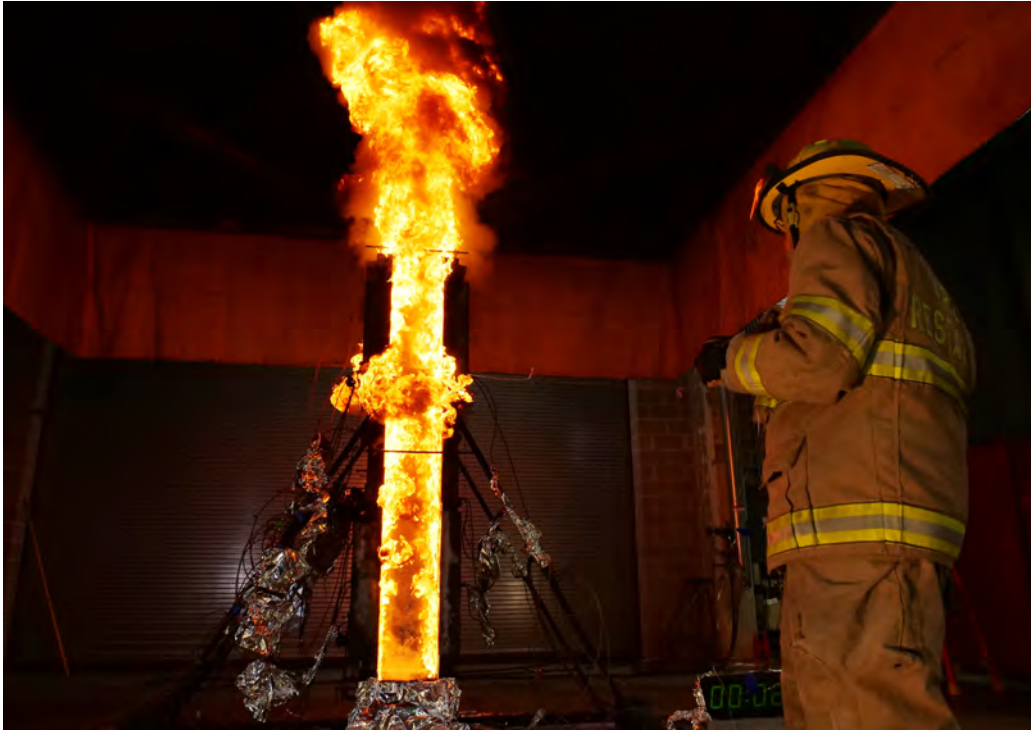
Fig. 74. Senior Technician Laurean DeLauter safely removes shields from heat flux gauges to enable measurements of flame-to-surface radiation heat flux during Test ABS R3.
