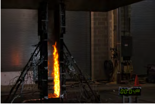
(a) Shortly after ignition, \dot{Q} = 120 kW
