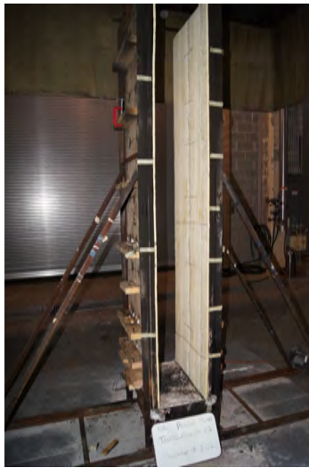
(a) Mounting of Polyiso panels prior to ignition
