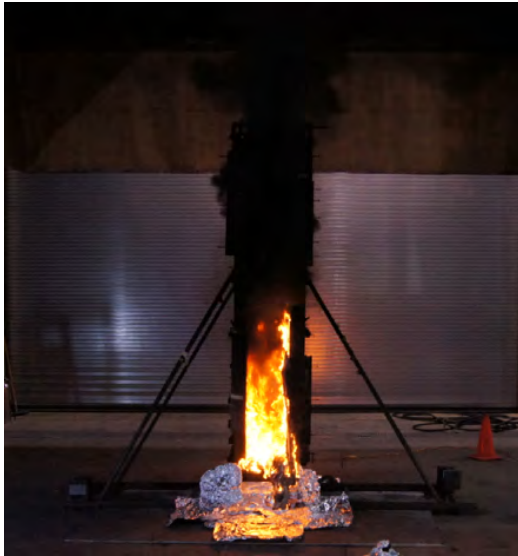
(c) Dripping and Heavy Soot Formation
