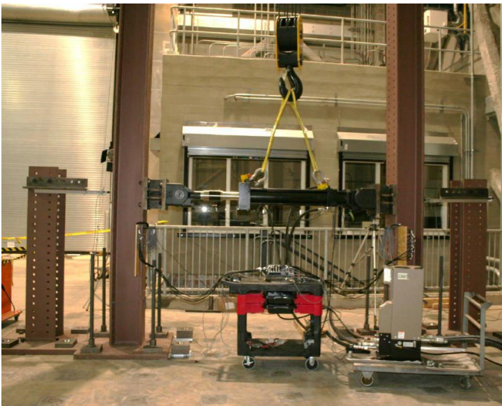
Fig. 40. Stiffness test to calibrate boundary conditions at the column base plates.
