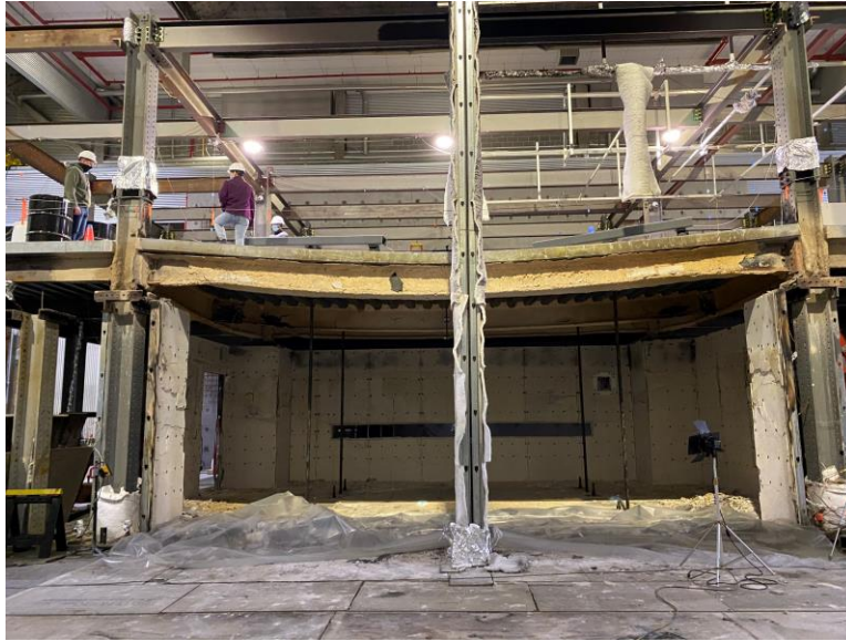
Fig. 1. The composite-steel-framed floor system tested in the NIST NFRL CF2 Test [Choe et al. 2022]
