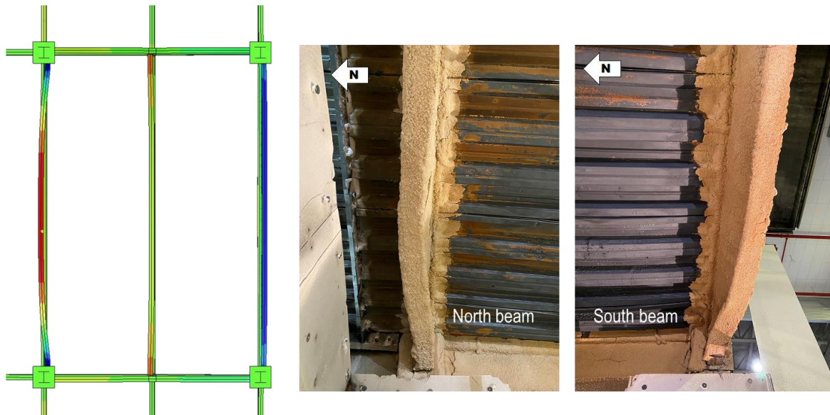
Fig. 110. Simulated and observed lateral displacement of bottom flanges of the north, and south W16×31 beams (test pictures are from Choe et al. 2022).
