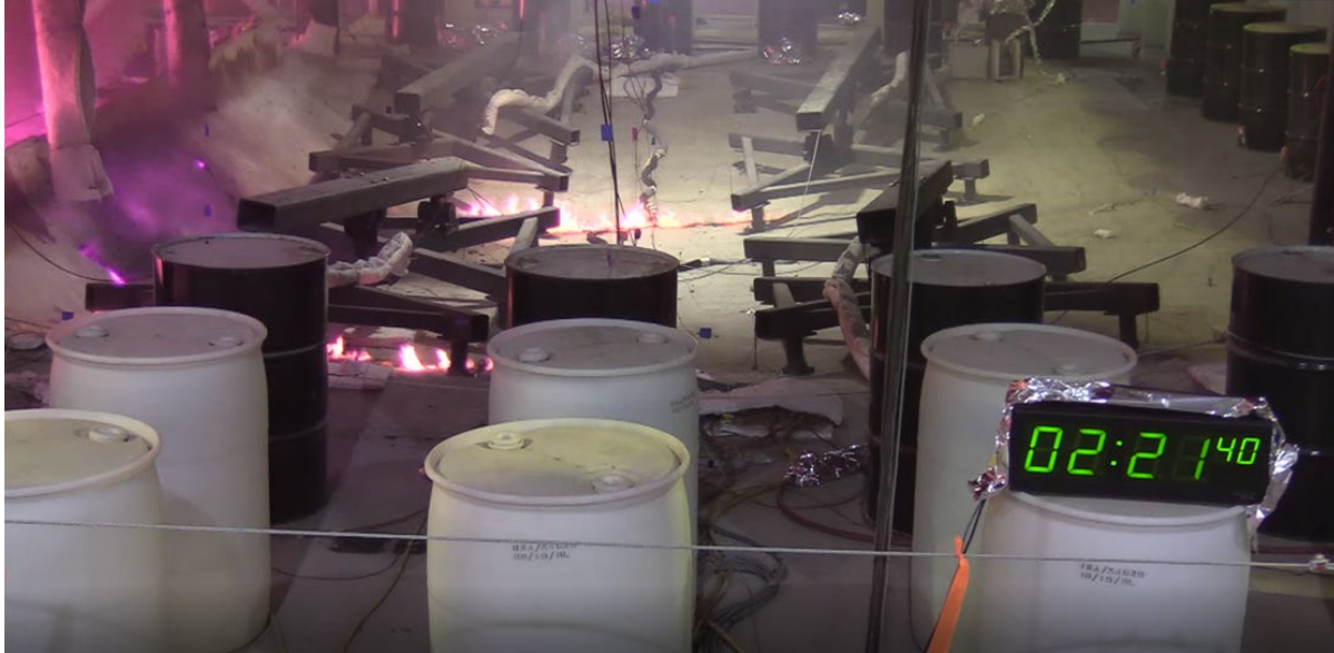
Fig. 15. Snapshot from the test video showing top of the test floor specimen at 142 min (2 hr:22 min) after the burner ignition. The pink color at the left side of this image is a camera artifact.
