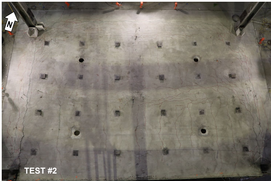
Fig. 3. Test #2 composite floor after cool down.
