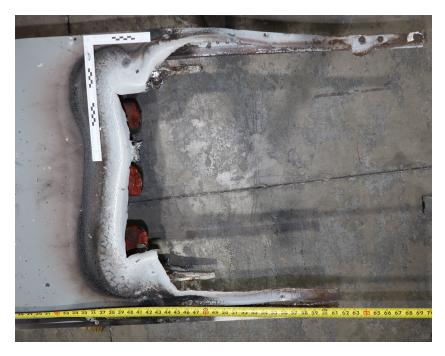
Fig. 171. Post-Experiment 2-28 Enclosure Breach
