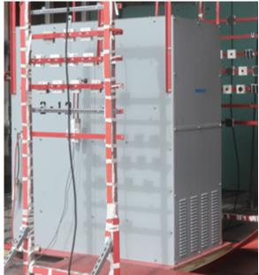
Fig. 150. Pre-Experiment 2-12 (as procured by the NRC). Top left (Front door showing relays and controls), Top right (Front instrumentation and breaker compartment with door open) Bottom (Rear offangle view showing louver ventialtion on the rear bottom panel).
