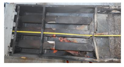
Fig. 60. Photo of Experiment 2-30 bus bars post-experiment (arc location shown right).
