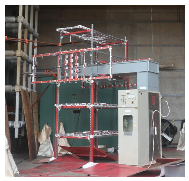
Fig. 14. Photo of bus duct instrumentation configuration prior to experiment
