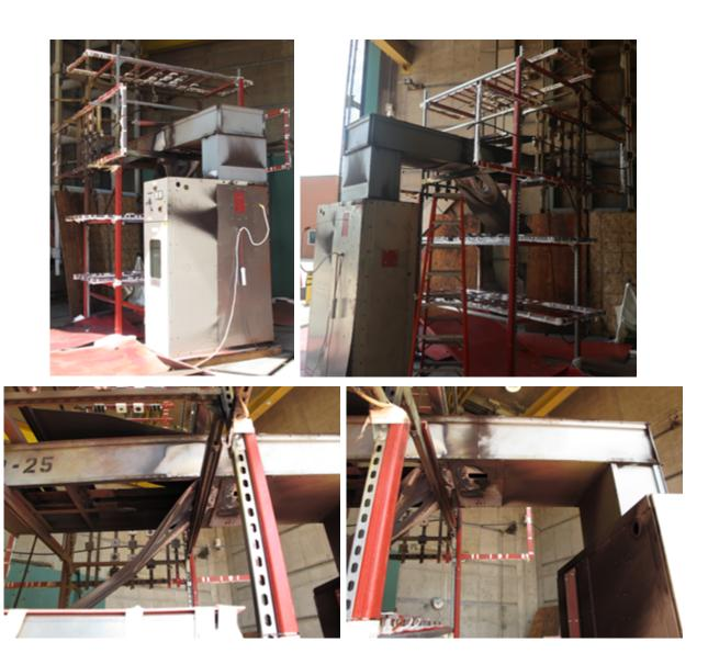
Fig. 156. Post-Experiment Experiment 2-25 (clockwise from top-left, Front angle; rear angle; front showing panel damage; front showing splice joint with breather)
