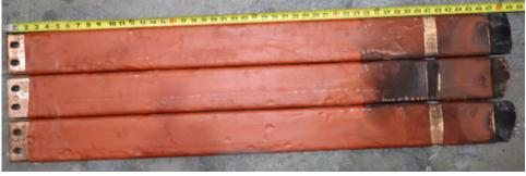
Fig. 165. Post-Experiment 2-27 Conductors (top – conductors in duct at end of experiment; bottom – conductors removed A-B-C: top to bottom)
