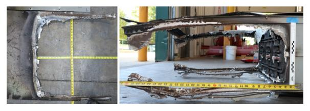
Fig. 166. Post-Experiment 2-27 Enclosure Breach (Top-left – top cover; Top-right – front side; Bottom-left – bottom cover; Bottom-right – rear side)
