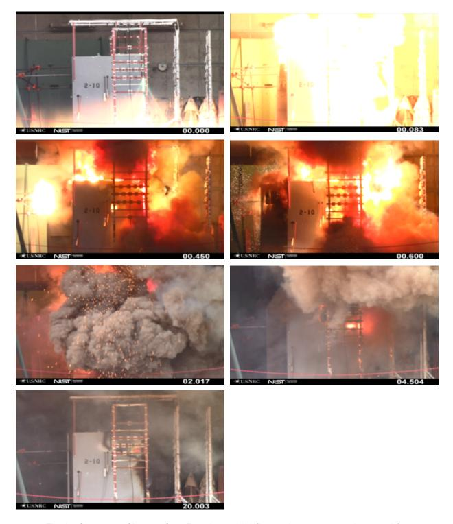
Fig. 16. Sequence of Images from Experiment 2-10 (image time stamps are in seconds).
