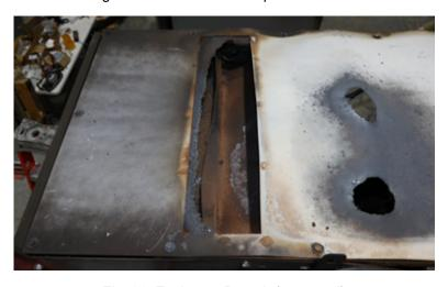
Fig. 26. Enclosure Breach (top panel)
