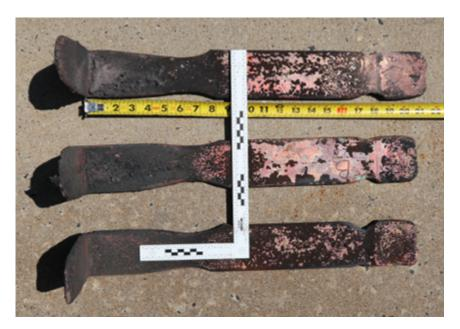
Fig. 27. Photo of Experiment 2-12 bus bars post-experiment (arc location shown right).
