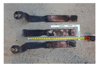
Fig. 19. Photo of Experiment 2-10 bus bars post-experiment (arc location shown right).
