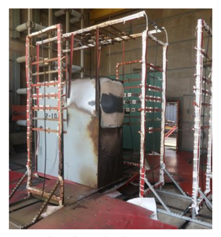
Fig. 18. Enclosure Post-Experiment 2-10.
