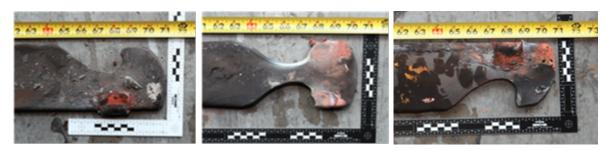
Fig. 162. Post-Experiment 2-26 Conductors (top – with conductors in duct; Bottom conductor ends A-B-C left to right)
