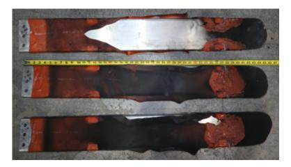
Fig. 66. Photo of Experiment 2-30B bus bars post-experiment (arc location shown center).
