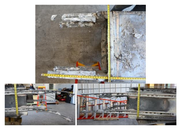
Fig. 190. Post-Experiment 2-32 Enclosure Breach 90 degree steel duct (Top – overhead view; Bottom-left – rear; Bottom-right – front)
