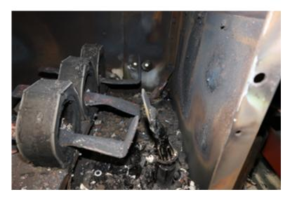
Fig. 22. Photo of severed bus bars at insulating bushing (breaker stab bottles).
