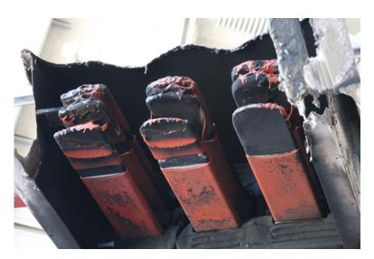
Fig. 78. Photo of Experiment 2-32 bus bars post-experiment
