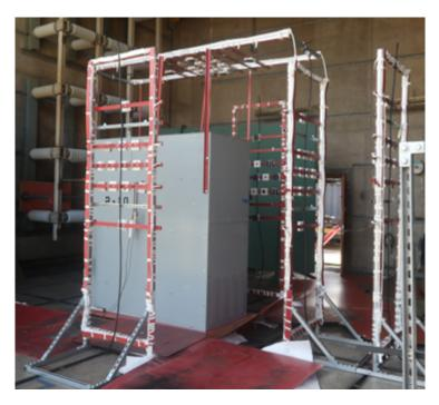
Fig. 11. Photo of instrumentation racks during experimental setup
