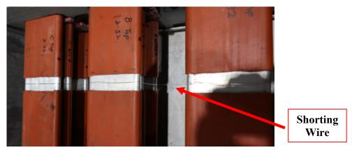
Fig. 74. Shorting wire location Experiment 2-32.
