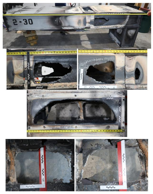
Fig. 175. Post-Experiment 2-30 Enclosure Breach (Top – front; Upper-Mid-left – front breach; Upper-Mid-right – rear breach; Lower-Mid – top breach; Bottom-left – lower cover front; Bottom-right – lower cover rear)
