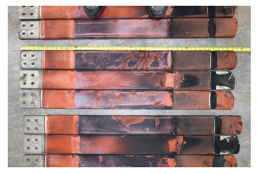
Fig. 79. Photo of Experiment 2-32 bus bars post experiment (arc location shown right)
