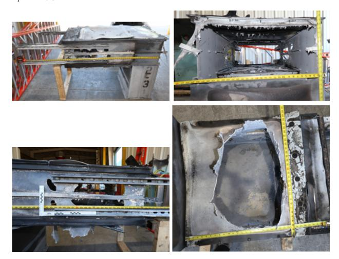
Fig. 184. Post-Experiment 2-31 Enclosure Breach (Top-left – 90 degree front; Top-right – 90 degree end; Bottom-left – 90 degree rear; Bottom-right – 90 degree lower cover)
