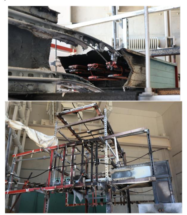
Fig. 187. Post-Experiment 2-32 (Top – rear view of enclosure breach and conductors; Bottom – Front view)
