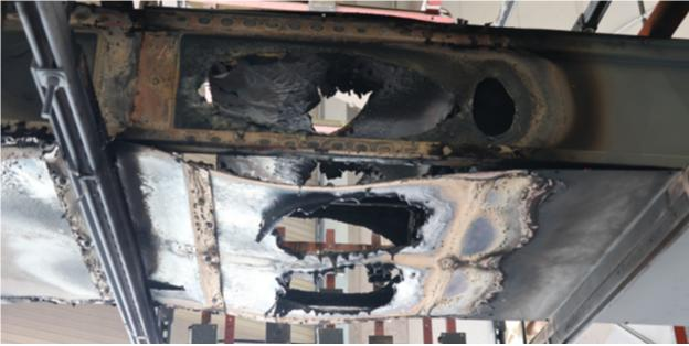
Fig. 179. Post-Experiment 2-30B Enclosure Breach (Top – view from below duct front; Bottom – view from below duct rear)
