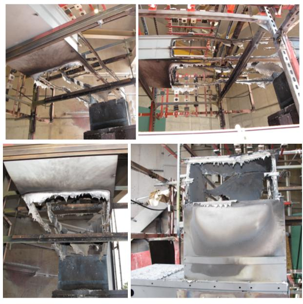
Fig. 164. Post-Experiment 2-27 (Top left – below bus duct front; Top-right – front; bottom-left (directly below duct; bottom-right (end of duct at 90 degree bend))
