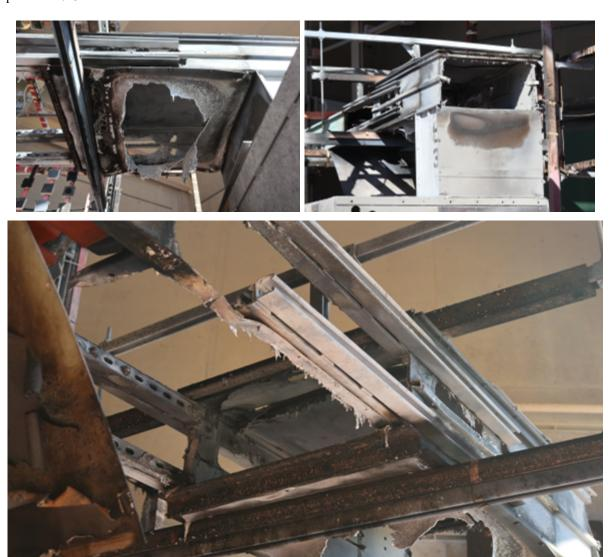
Fig. 182. Post-Experiment 2-31 (Top-left – bottom horizontal duct cover on 90 degree; top-right – end view of 90 degree; bottom – view from below duct in front)
