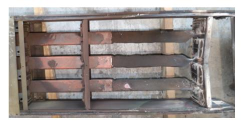
Fig. 39. Photo of Experiment 2-26 bus bars post-experiment (arc location shown center).
