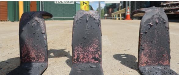
Fig. 149. Post-Experiment Conductors. Top (Plan view of primary cable connection bus bars; top – Phase C, middle – Phase B, bottom – Phase C), Bottom (elevation view of primary cable connection bus bars; left – Phase A, center – Phase B, right – Phase C)
