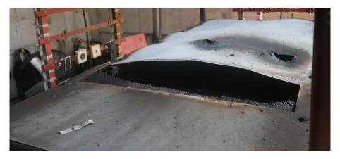
Fig. 154. Post-Experiment Enclosure Breach
