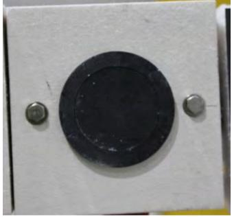
Figure 10 Cross-section of ASTM Slug (top) nominal dimensions in millimeters, photo of device being prepared in the field (bottom). Note that the two bolts on each side of the device are used for mounting to the DIN rail of the instrumentation rack.
