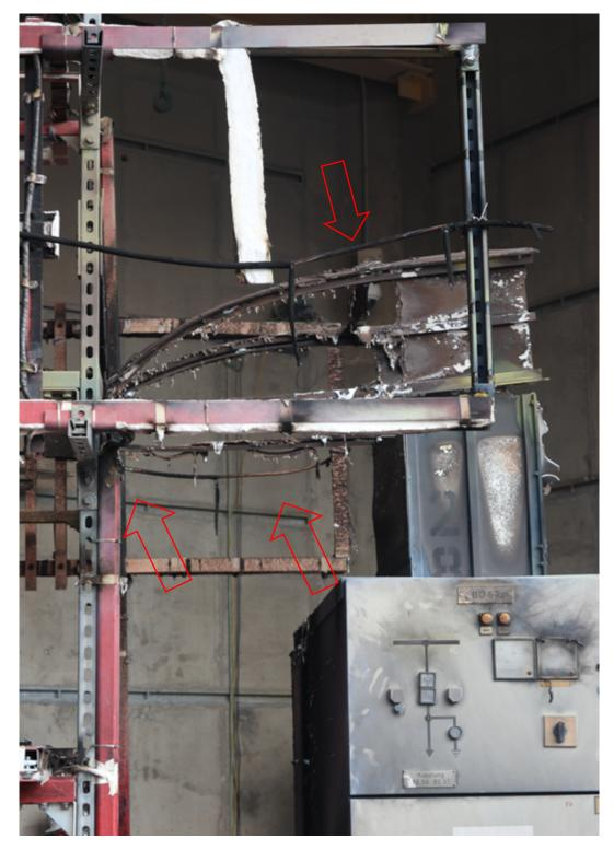
Fig. 48. Location of cable jacket damage relative to equipment. (Red arrows identify locations missing cable jacket and in some cases conductor jacket)
