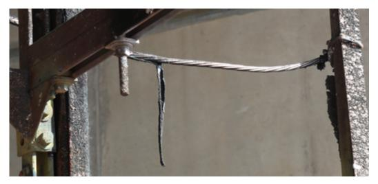
Fig. 170. Post-Experiment 2-28 insulated conductor Rack 2 at 90 degree bend end
