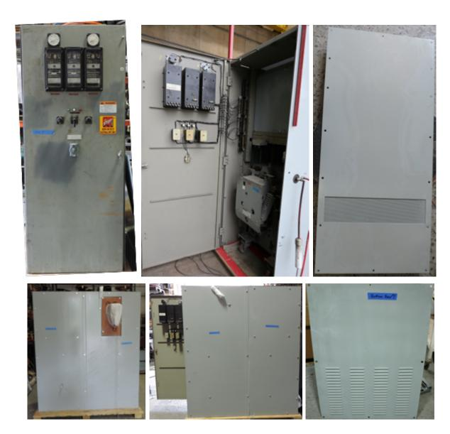
Fig. 146. Pre-Experiment 2-10 (as procured by the NRC). Top left (Front door showing relays and controls), Top center (Front instrumentation and breaker compartment with door open), Top right (top of enclsoure showing vent, vent located over main bus and near front door), Bottom left (power supply side with main bus extensions covered with foam for personal protection), Bottom center (opposite side from power supply side), Bottom right (rear panel showing louver vents).
