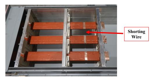
Fig. 41. Shorting wire location Experiment 2-27
