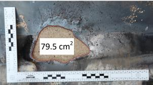
Fig. 145. Photos showing breach opening with size estimate.
