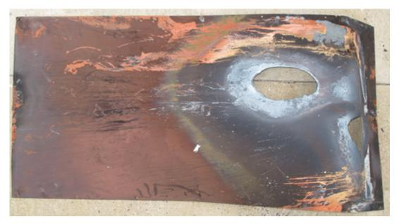
Fig. 159. Post-Experiment Experiment 2-25 Enclosure Breach (note panel is not lying flat on ground near right side, there is a bend downward near the right breach).
