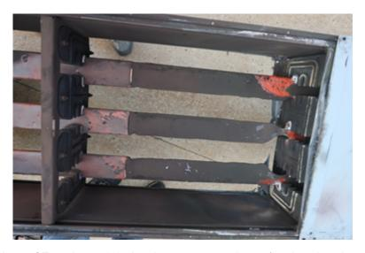
Fig. 33. Photo of Experiment 2-25 bus bars post-experiment (arc location shown center).
