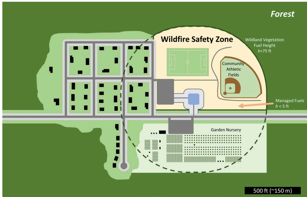
Fig. 11. Conceptual illustration of a 100 ft × 100 ft (30 m × 30 m) safety zone surrounded by non-uniform, yet managed, fuels. Two access pathways are also provided.
