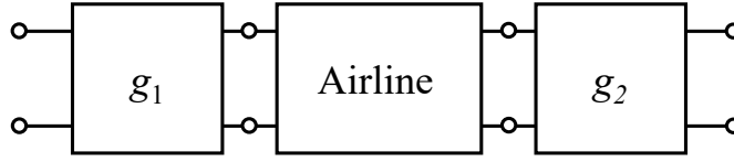
Fig. 3. Airline connected to two-port VNA has a gap at each port.
