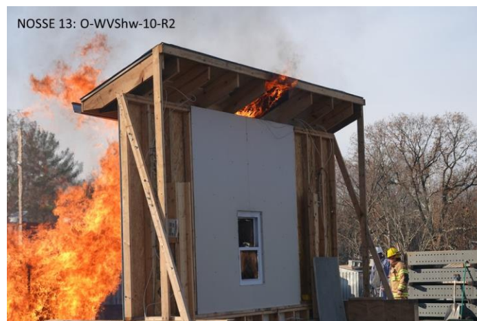
Fig. 53. Photograph showing flames penetrating through the vent for test O-WVShw-10-R2 .
