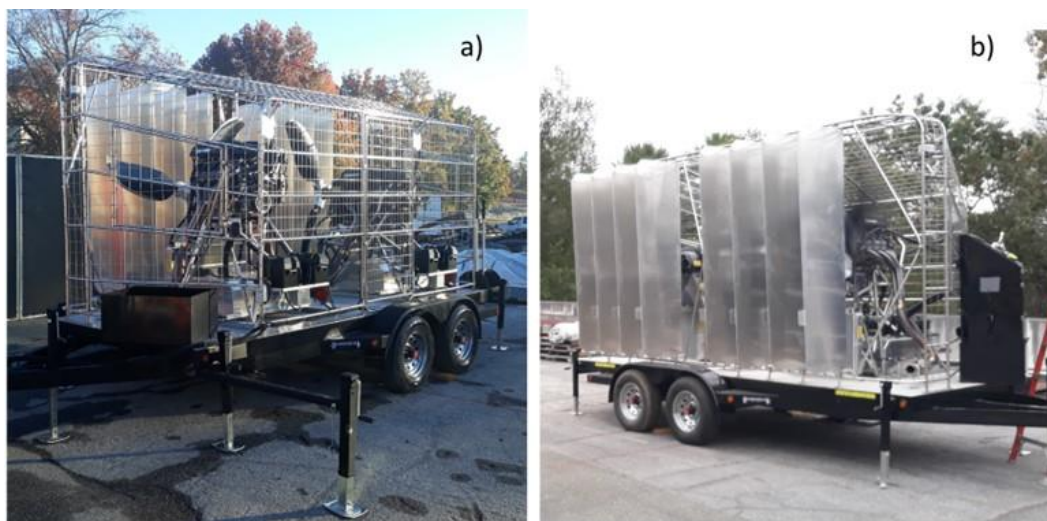
Fig. 6. Dual fan wind machine, a) rear view, and b) front view.
