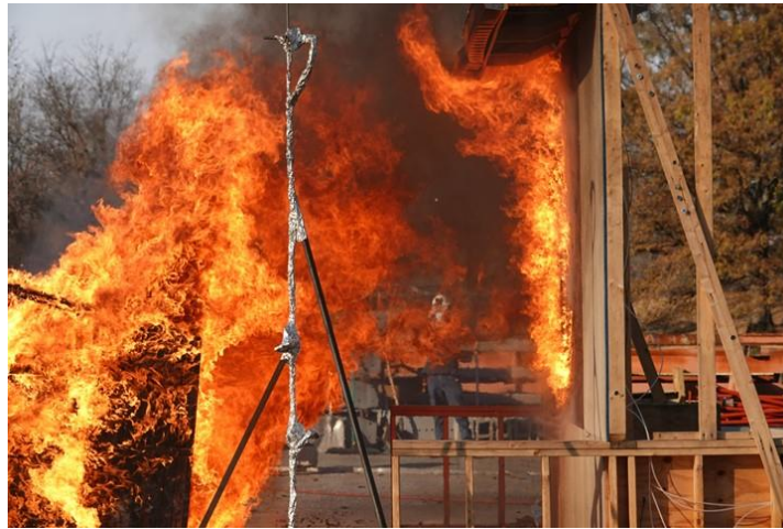
Fig. 48. Photograph showing ignition of exposed OSB in Test NOSSE13: O-WVShw-10-R2 .
