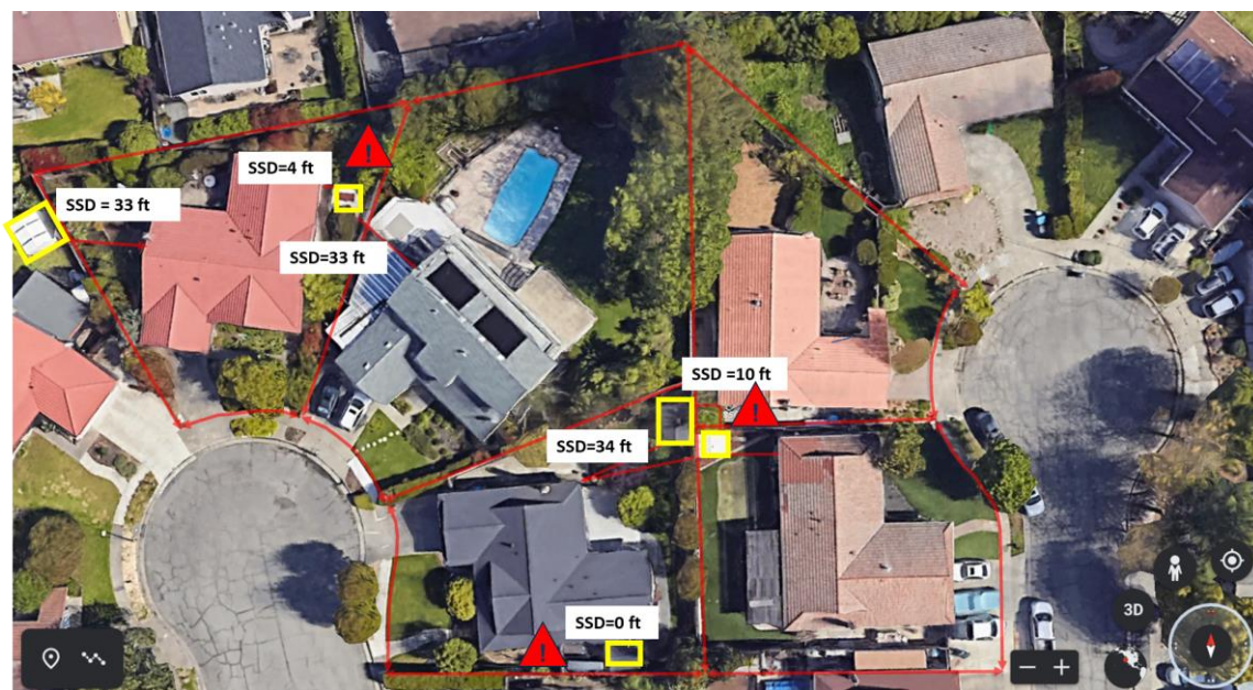
Fig. D-5. Case 3: Community showing shed hazard only for neighboring residence. (1ft = 0.305 m)
