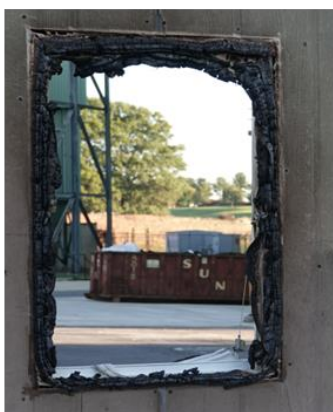
Fig. 49. Photographs showing window damage for different exposures.
