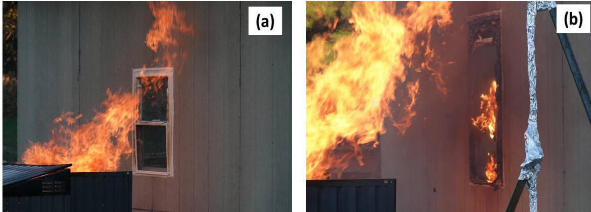
Fig. 50. Photographs showing (a) flame jetting from noncombustible steel Closet in test O-Schw-5 and (b) ignition of vinyl frame.
