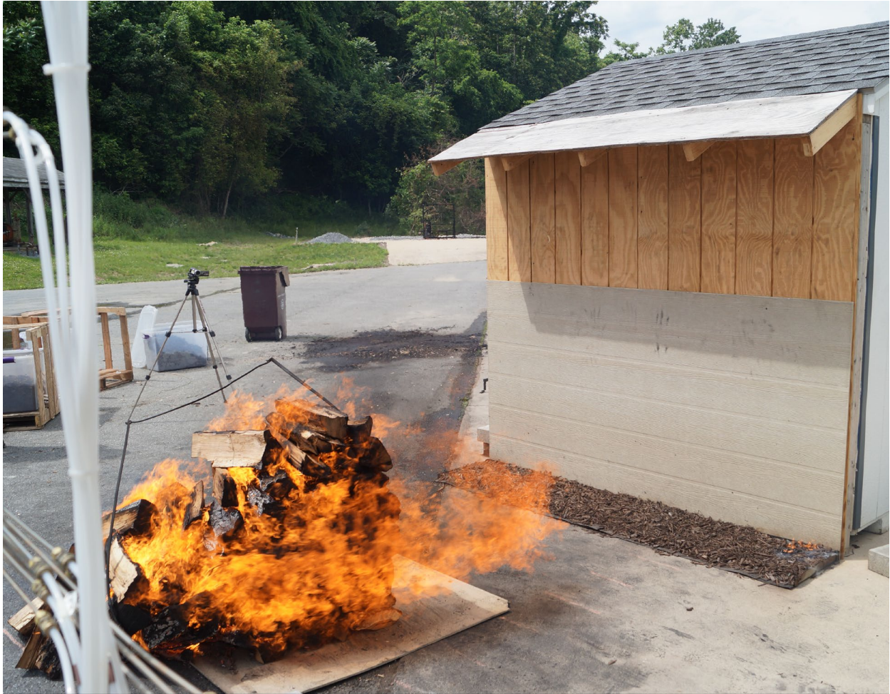
Fig. 61. A photo of a collapsed tall, sides, no rack dry oak woodpile under 6 m/s (13 mi/h) winds.
