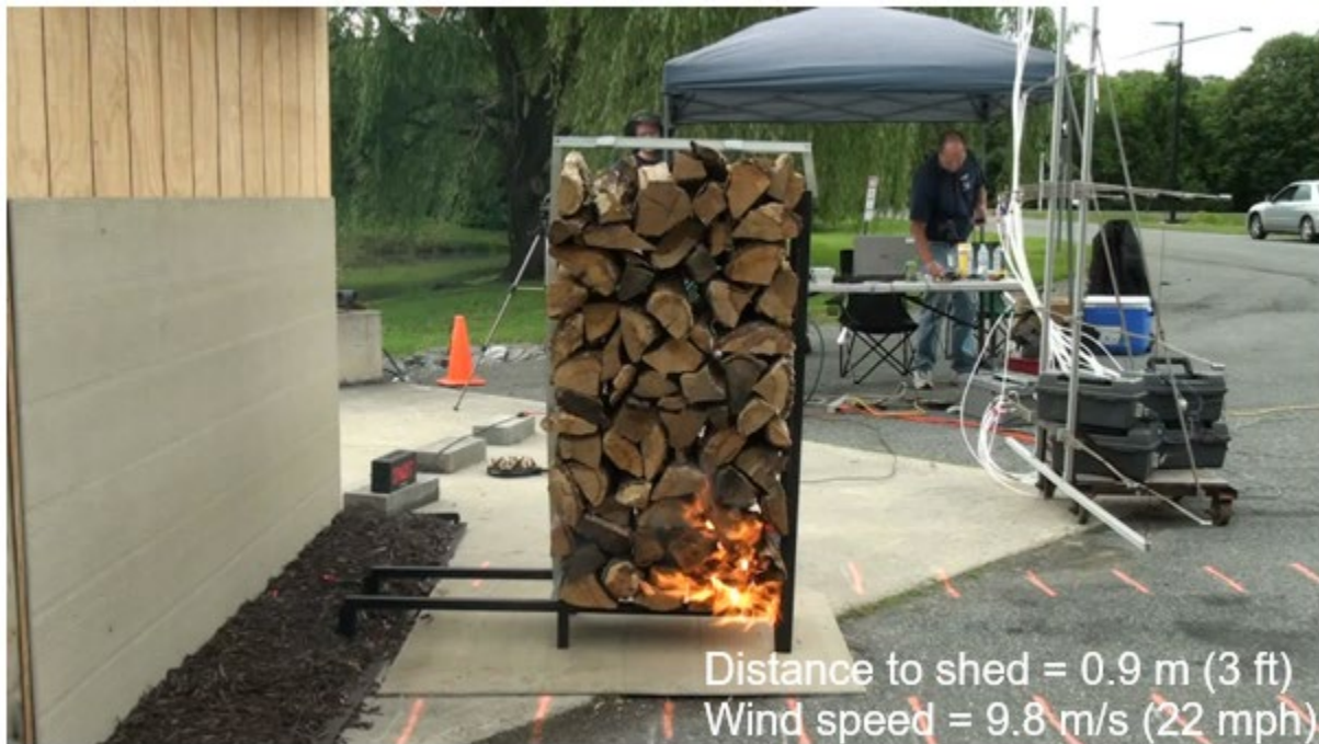
Fig. 17. A 0.91 m (3 ft) separation distance oak logs experiment in a tall, sides, elevated configuration, within 30 s of wind initiation.
