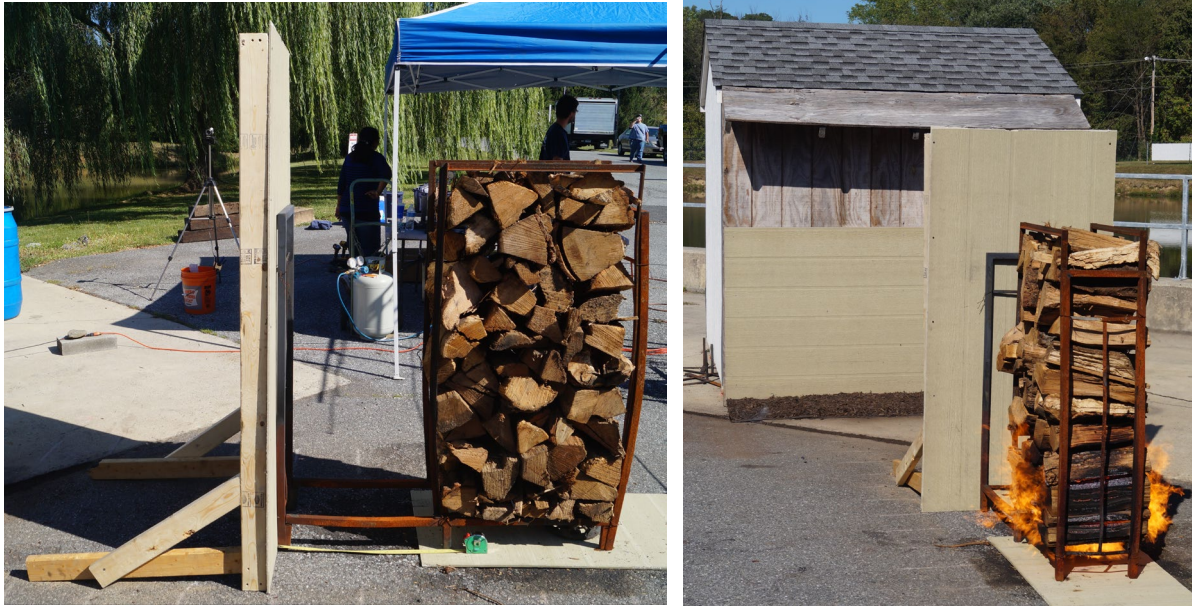
Fig. 63. Photographs showing the first woodpile mitigation experiment, which used a noncombustible wall as a shield in an attempt to decrease downwind spot fires.
