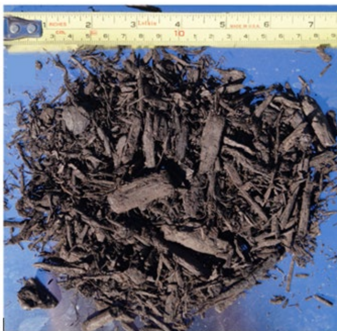
Fig. 6. A photograph of the shredded hardwood mulch used in the target mulch bed.
