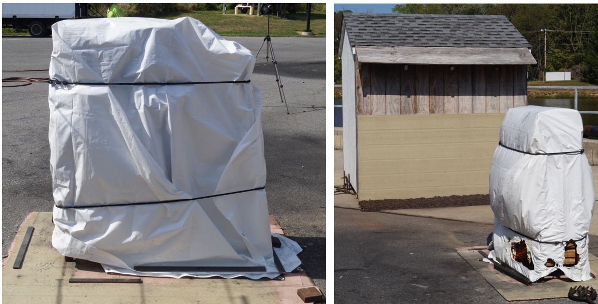
Fig. 64. Photographs showing the woodpile mitigation experiment using a fire-retarded tarp in an attempt to decrease downwind firebrand spot fires.
