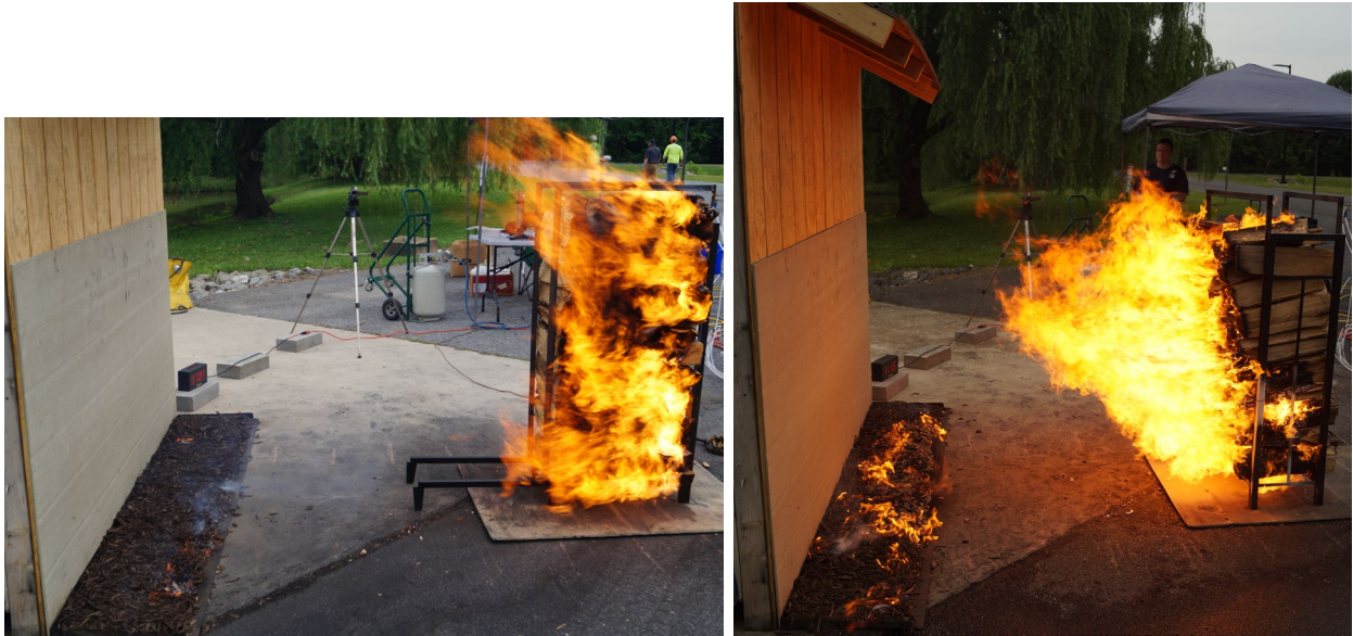
Fig. 43. Photographs of sides (left) and ends (right) dry oak woodpile experiments configured as tall with racks at 1.83 m (6 ft) separation and low winds.
