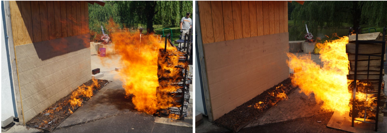
Fig. 52. Photographs of no-rack (left) and with-rack (right) dry oak woodpile experiments configured as ends and tall at 1.83 m (6 ft) separation and low winds.
