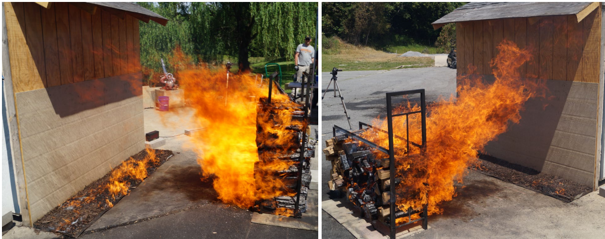
Fig. 34. Photographs of tall (left) and short (right) dry oak woodpile experiments configured as ends with racks at 1.83 m (6 ft) separation and low winds.
