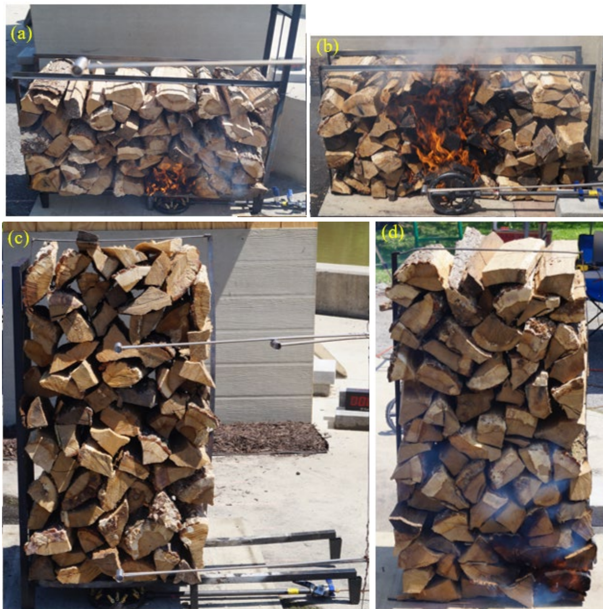
Fig. 8. Photos of woodpile configurations (clockwise from top left): (a) short with a rack, (b) short without a rack, (c) tall with a rack, and (d) tall without a rack.
