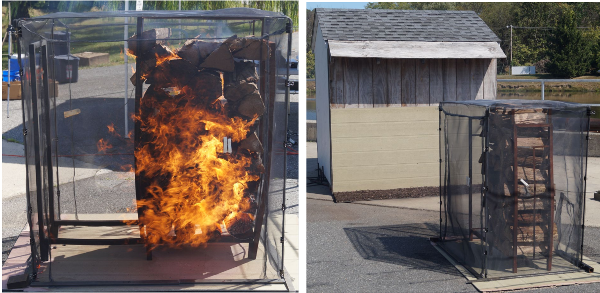
Fig. 65. Photographs showing the woodpile mitigation experiment using a screen enclosure in an attempt to decrease downwind firebrand spot fires.
