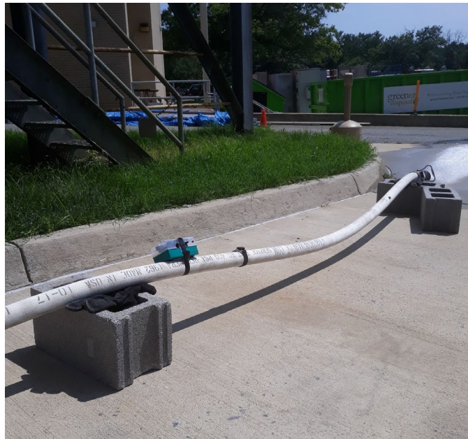
Fig. 7. The accelerometer was elevated off the ground at the front hose location in the stationary holding position. The accelerometer was suspended between two blocks simulating the hose condition where the hose nozzle and hose were held off the ground.
