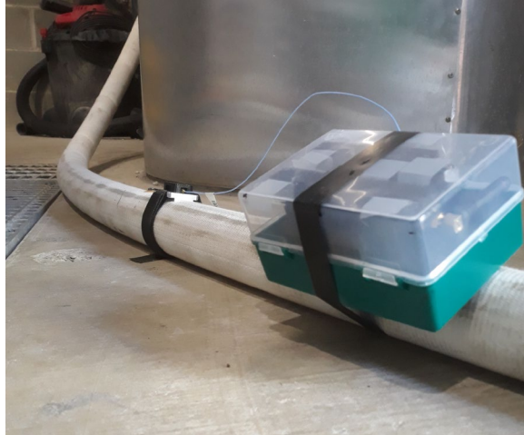
Fig. 6. The accelerometer at the back hose location for the hose in the stationary position where the accelerometer was attached to the hose resting on concrete.
