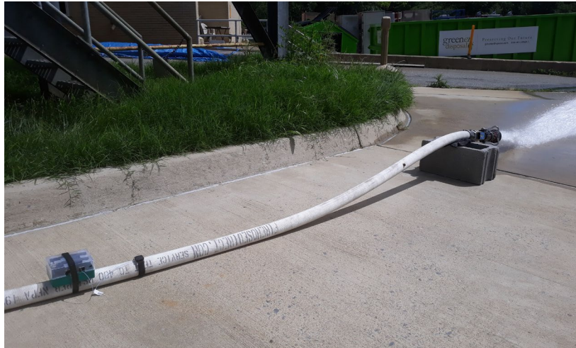
Fig. 4. The accelerometer at the front hose location for the hose in the stationary on ground condition, where the accelerometer was attached to the hose resting on concrete. The nozzle was elevated by the block to prevent vibrations between the nozzle and concrete.
