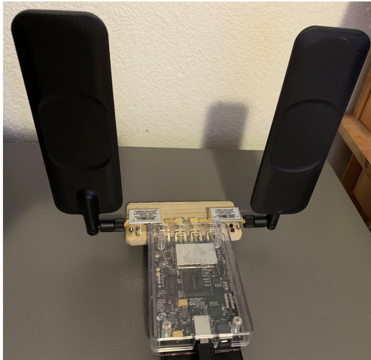
Figure 3.1: An assembled sensor node, with an SDR enclosed inside the transparent enclosure. The antennas shown were the omni-directional models used in the residential telework setting.
