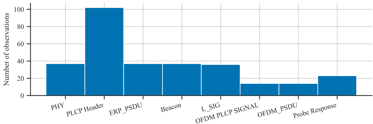
Figure E.21: Histogram of packet types observed in WLAN measured from hospital 2021-09-24 data at 2462.0 MHz
