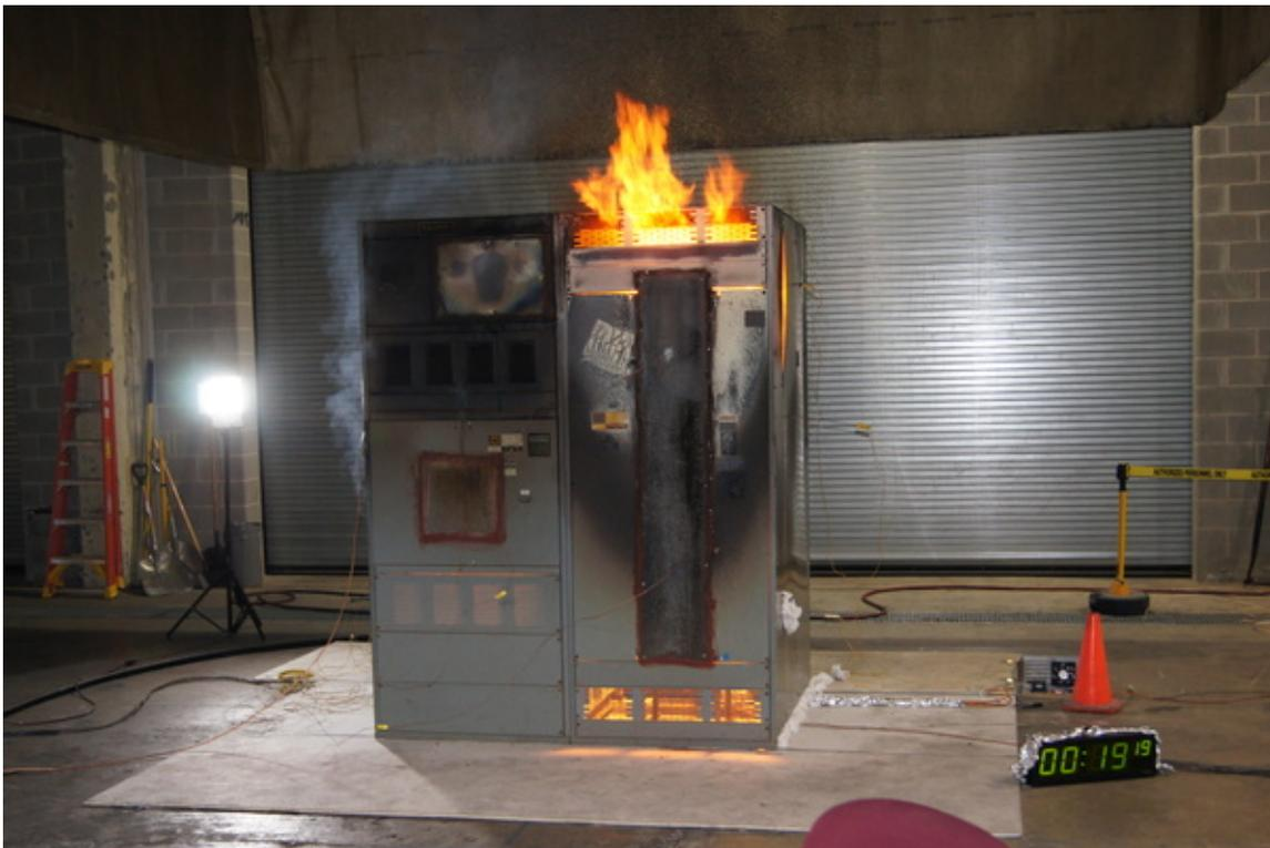
**Fig. 19.** Heat release rate, gas concentrations, and photograph of Experiment 2.
