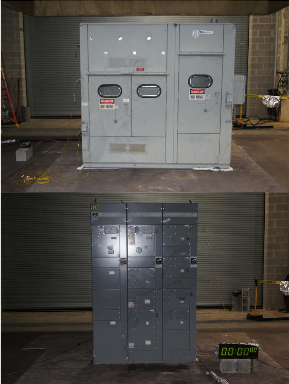
**Fig. 4.** Photographs of Enclosures #7 (top) and #8 (bottom). The acrylic windows in the top photograph were lined with aluminum tape to prevent their rubber gaskets from melting.
