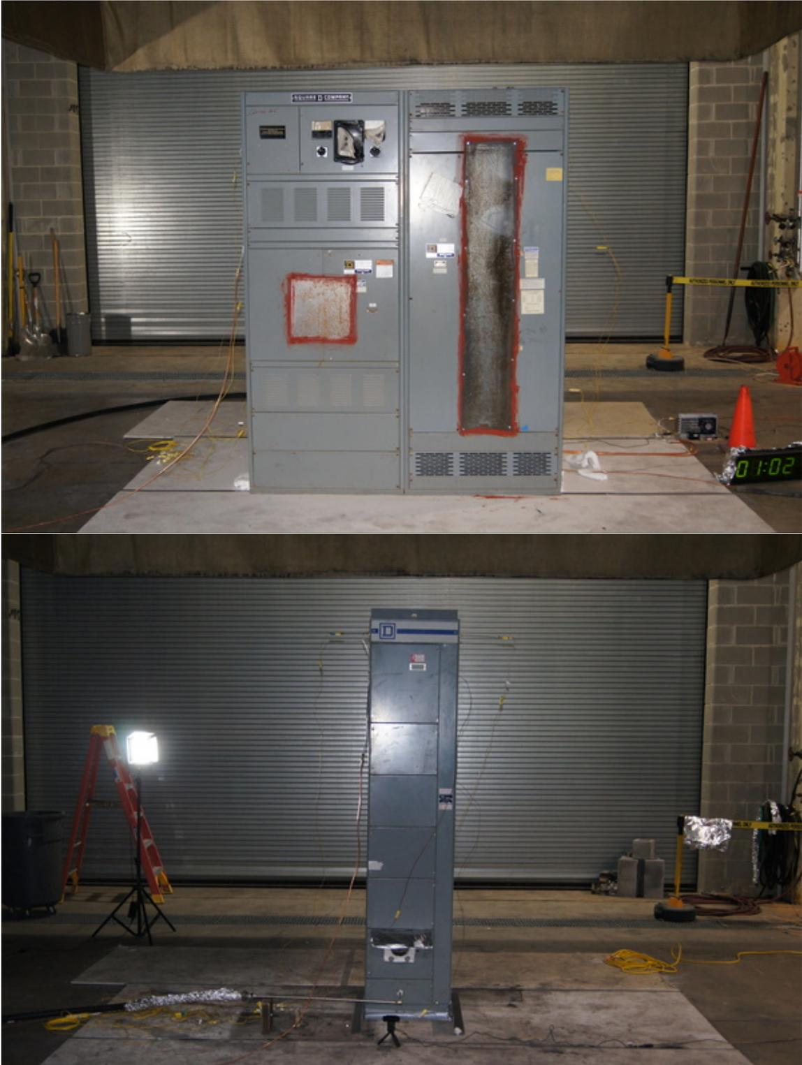
**Fig. 3.** Photographs of Enclosures #5 (top) and #6 (bottom). Steel plates sealed with heat-resistant caulk replace control panels.
