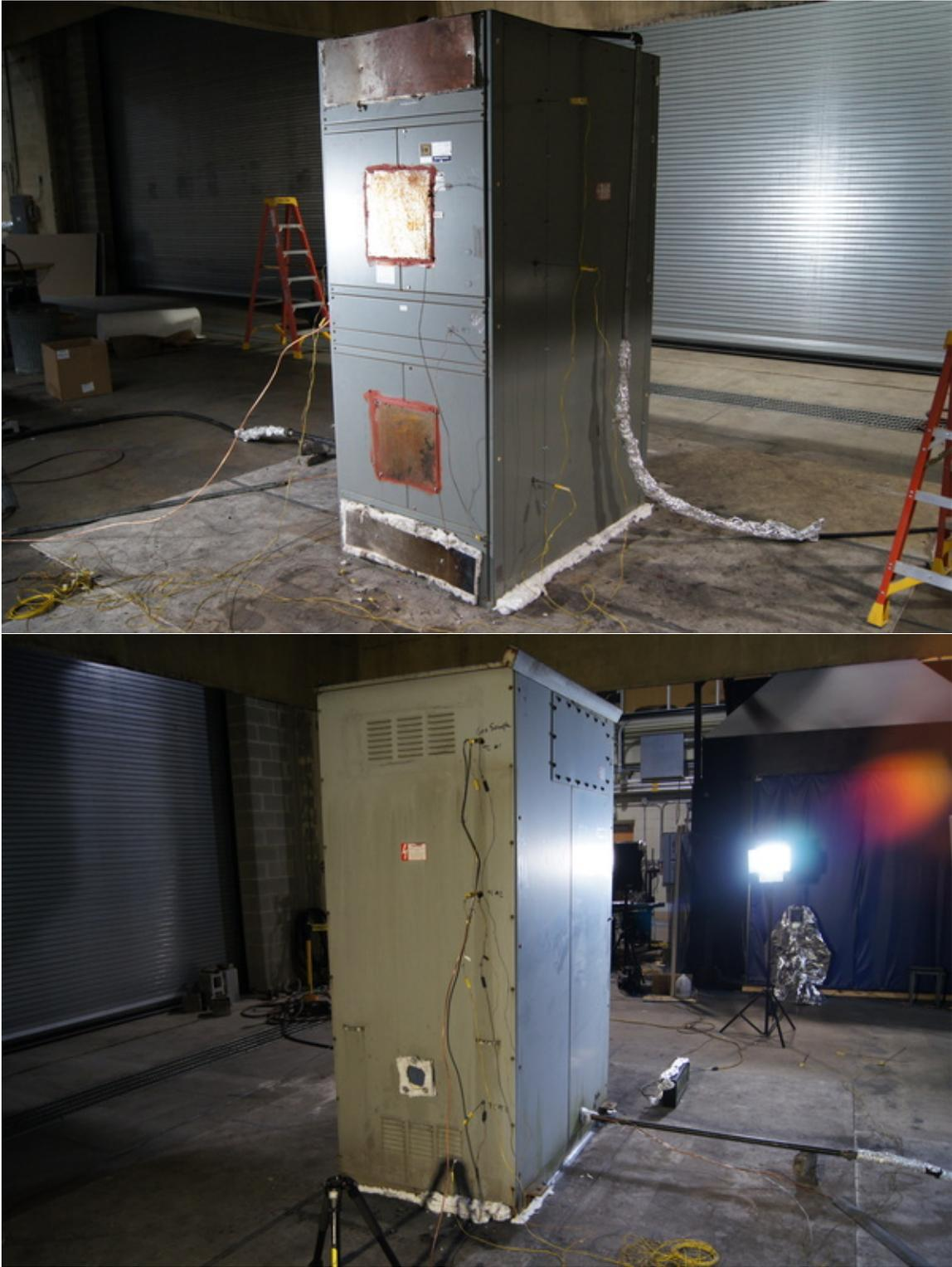
**Fig. 2.** Photographs of Enclosures #3 (top) and #4 (bottom). The steel plates in the top photograph have replaced control panels and are sealed with heat-resistant caulk. The hose leading to the top is an *ad hoc* sprinkler system. The circular window in the bottom photograph is a view port that was added to ensure that the fire did not extinguish.
