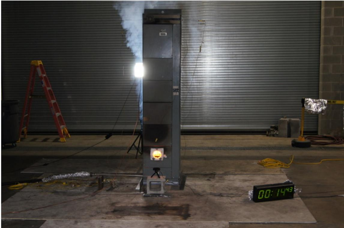
**Fig. 26.** Heat release rate, gas concentrations, and photograph of Experiment 9. Note the small quartz glass view port cut into the door opening to the lowest compartment where the burner was positioned.
