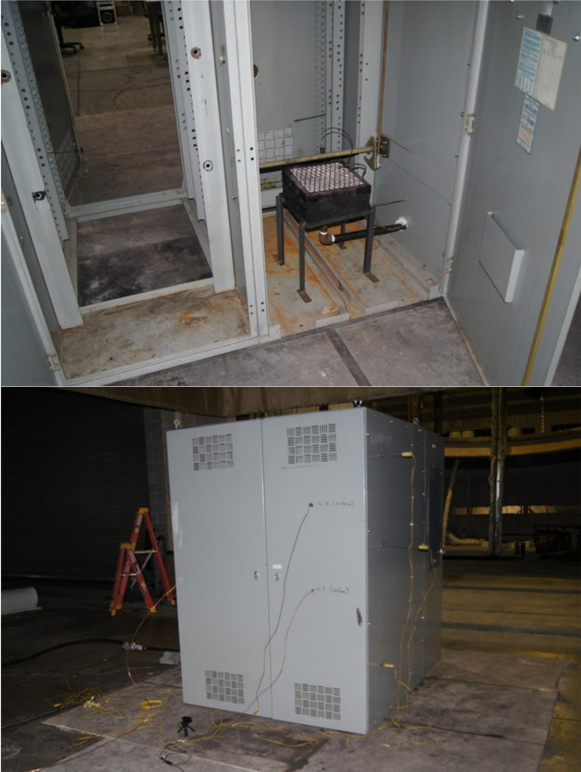
**Fig. 1.** Photographs of Enclosures #1 and #2. The exteriors of each are identical. At right in the top photograph is the natural gas burner. The exterior wiring is for thermocouples.
