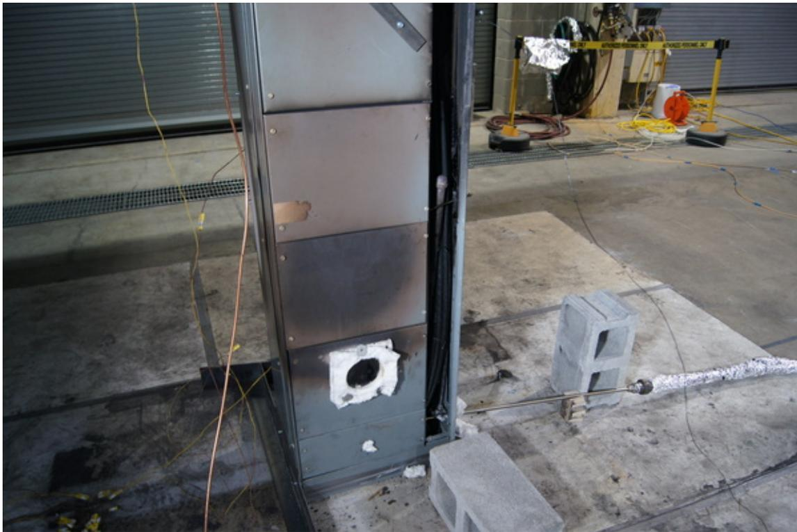
**Fig. 28.** Heat release rate, gas concentrations, and photograph of Experiment 11. The photograph shows the cables hung along the right channel with a steel pipe burner used to ignite them.
