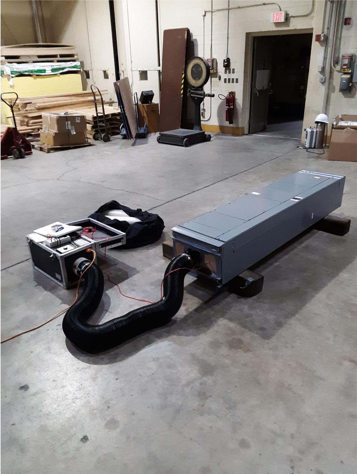
**Fig. 5.** Leakage measurement for Enclosure #6 using the DM4 Dual Digital Micro-Manometer manufactured by Infiltec Inc., Falls Church, Virginia.
