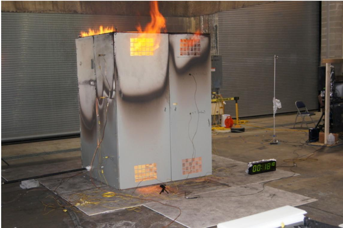
Fig. 8. Photograph showing flames emerging from a seam.
