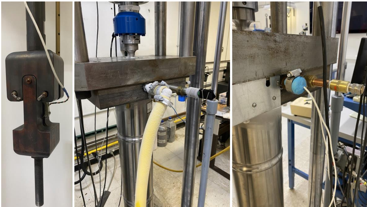
Figure 4 – (Left) Fracture toughness specimen placed into both fixtures, plus a rod-like liquid helium level indicator is visible behind the fixtures. (Middle) A smaller double-walled cylinder was placed in contact with the reaction frame (silicone seal placed between cylinder and frame) and tightened into place with threaded nuts. Each port on the experiment was either equipped with (middle) a gas recovery hose, a plug, (right) a seal around instrumentation wires, or a pressure relief valve.
