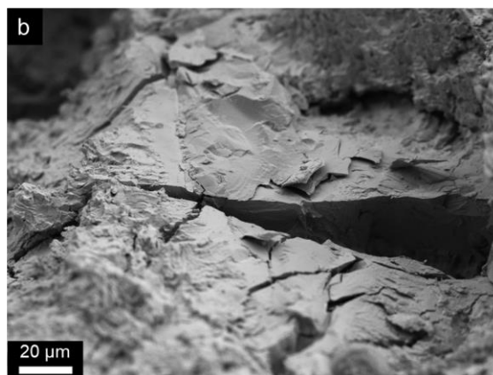
a) Crack jump, b) cleavage fracture
