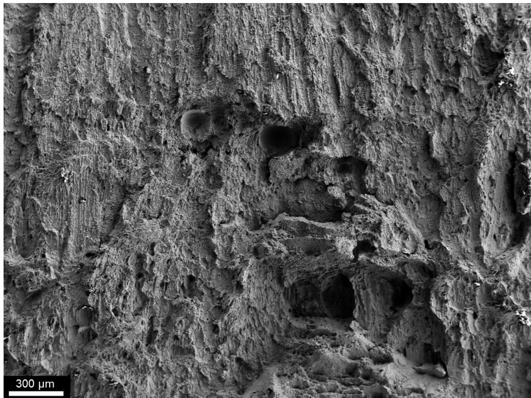
Large FOV of the fracture surface displaying lack of fusion porosity
