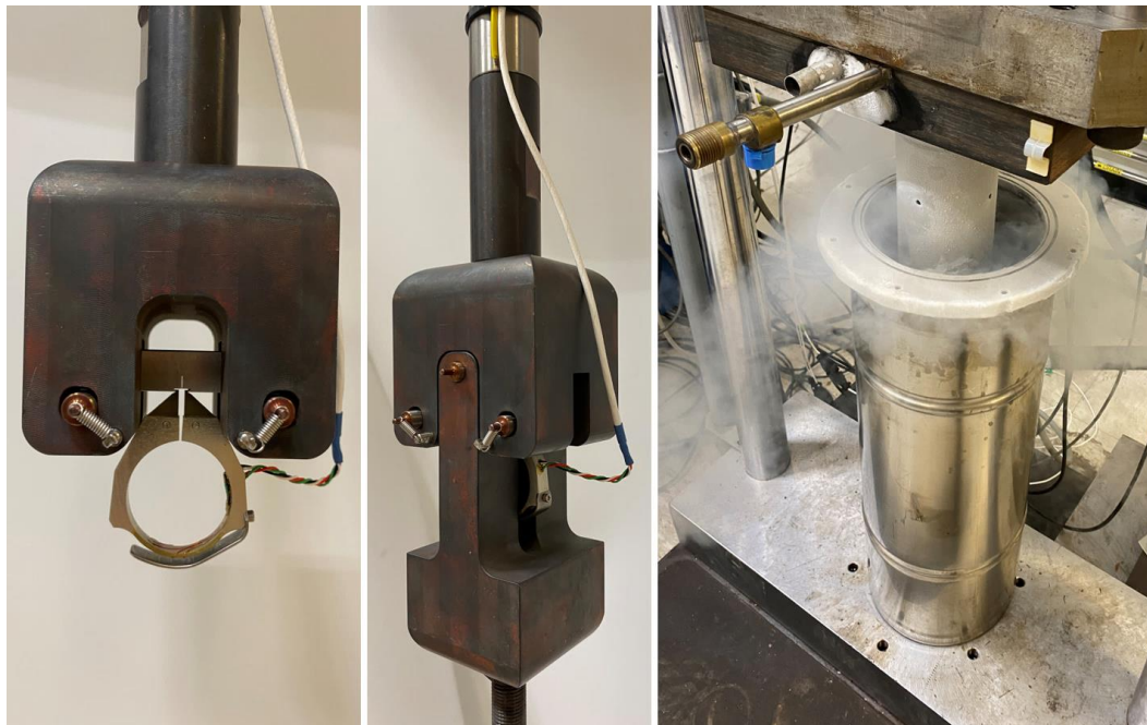
Figure 3 – (Left) Fracture toughness specimen placed in the upper fixture with the clip gage attached and (middle) lower fixture placed over the specimen and 3 rd loading pin inserted above the specimen. (Right) The sheath that protects the experimental setup and enables load bearing on the specimen is lowered into a double-walled cylinder filled with LN2.
