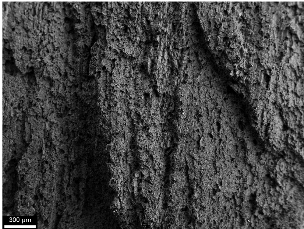
Large FOV of the fracture surface displaying a crack jump.
