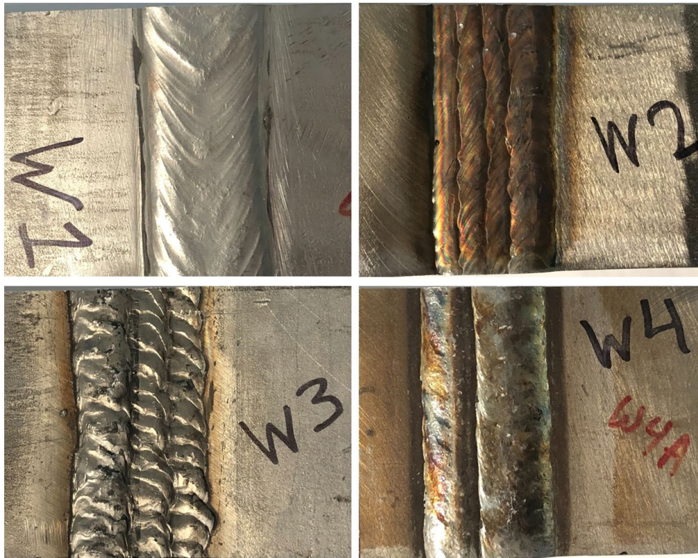
Figure 1 – Representative view of the top of each weld (weld cap / final cover pass). W1 used a single final pass, W2 used four final passes, W3 used three final passes, and W4 used two final passes.
