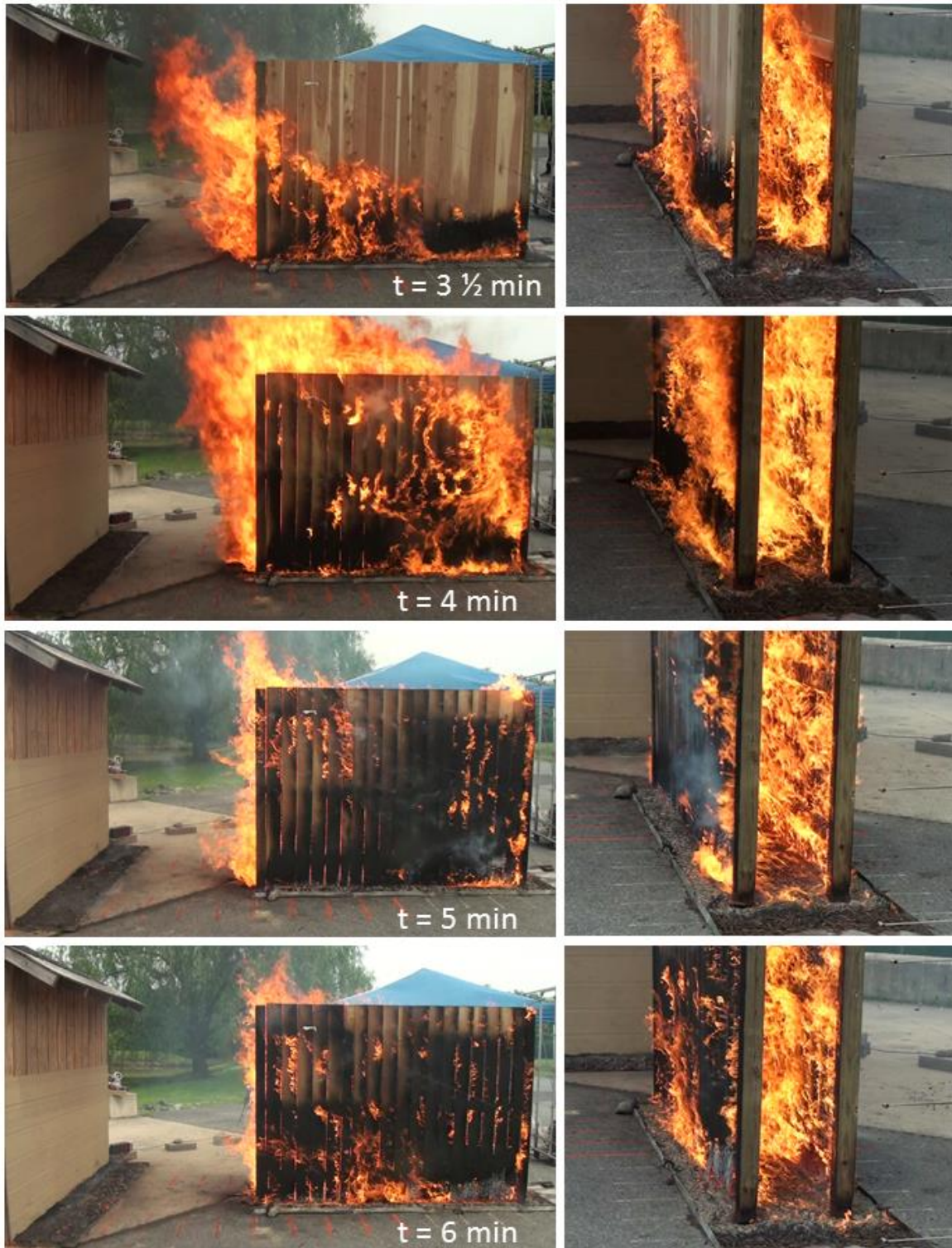
Fig. 117. Time sequence for parallel WRC privacy fences with shredded hardwood mulch at 46 cm (18 in) spacing and low wind speed [Test C-6], for times from 3 ½ min to 6 min.
