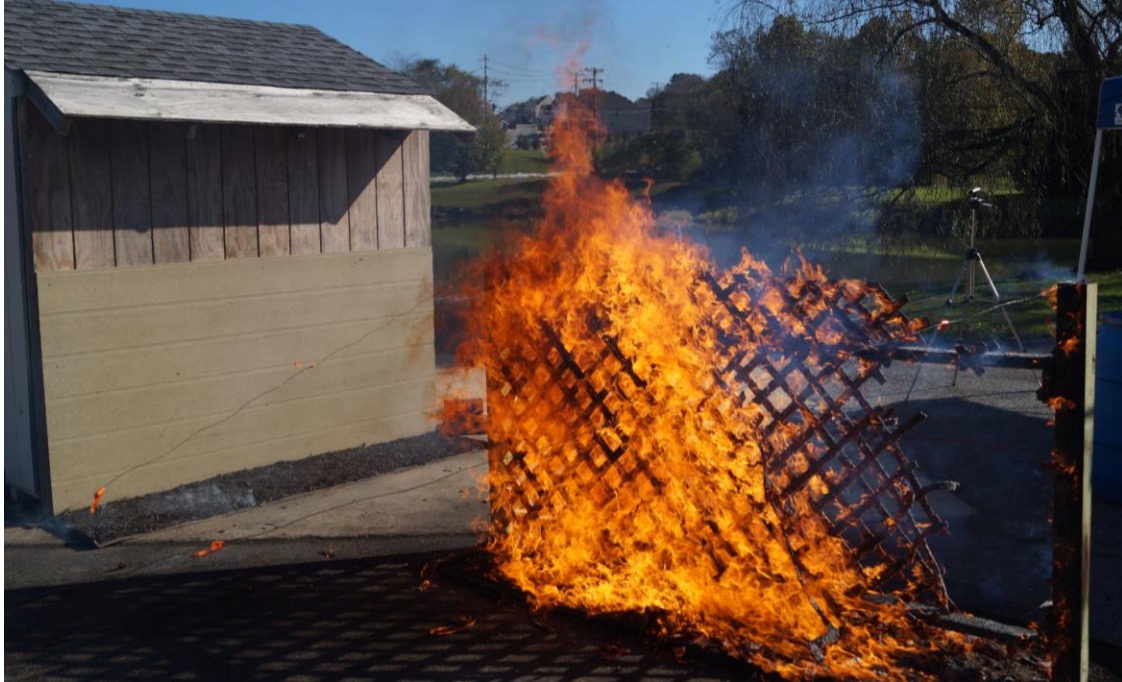
Fig. 120. Double pine lattice fence with shredded hardwood mulch at low wind speed, at about t = 3:15 [Test C-29]. Note spot fires in the target mulch bed at the base of the structure caused by firebrands.
