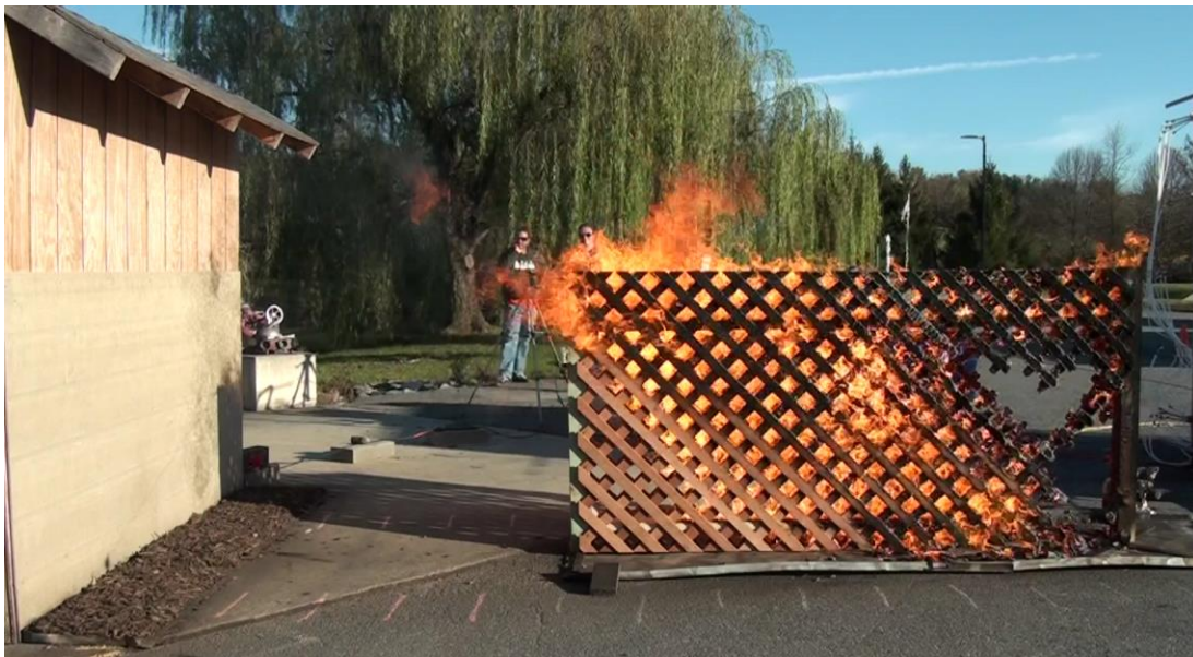
Fig. 131. Double redwood lattice fences without mulch at t = 4 min with low wind speed [Test A-110].
