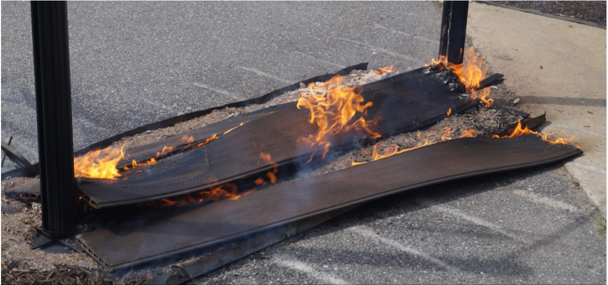
Fig. 101. Final configuration of wood-plastic composite boards after Test F-1 .
