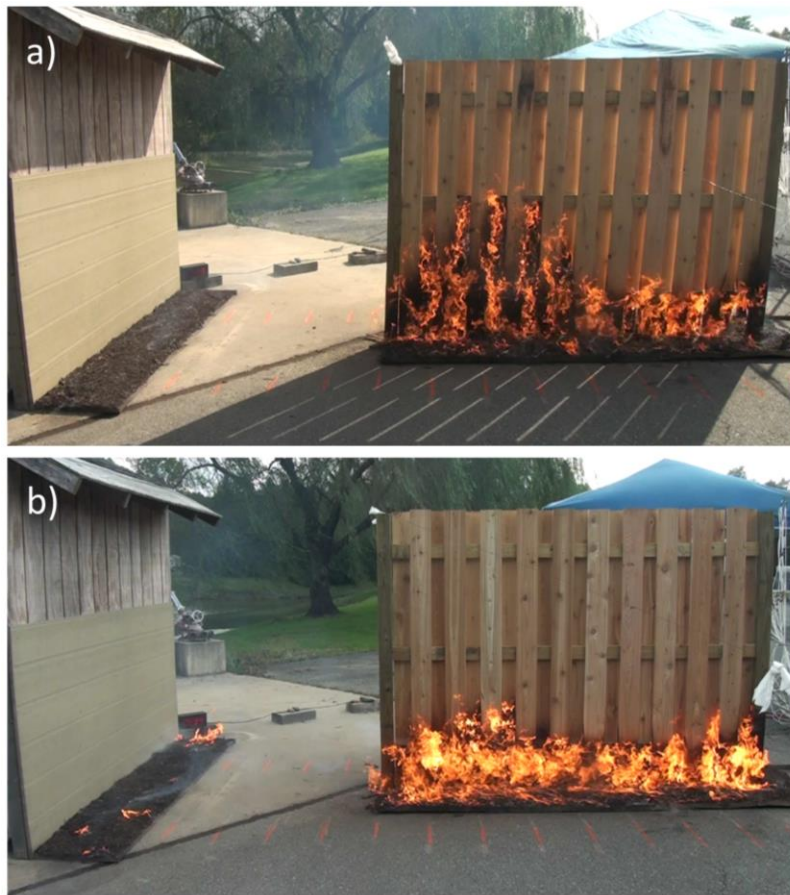
Fig. 95. Good neighbor fence experiments at a) t = 4.5 min for medium wind speed [Test C-22] and b) t = 2.6 min for high wind speed [Test C-23].
