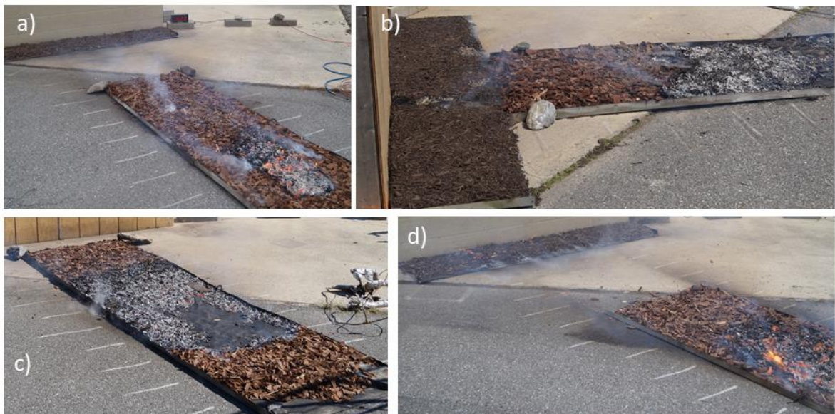
Fig. 39. Fire behavior examples for pine bark mulch beds with a) medium [Test A-100], b) low [Test C-4], c) medium [Test A-72], and d) high [Test A-86] wind speeds.
