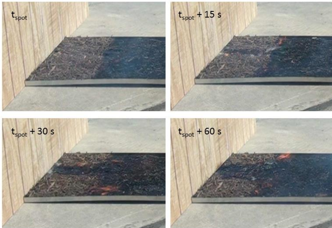
Fig. 34. Time evolution of firebrand spot fire ignited at wall of structure, beginning with first sign of spot fire at t_{\text{spot}} [Test A-2].
