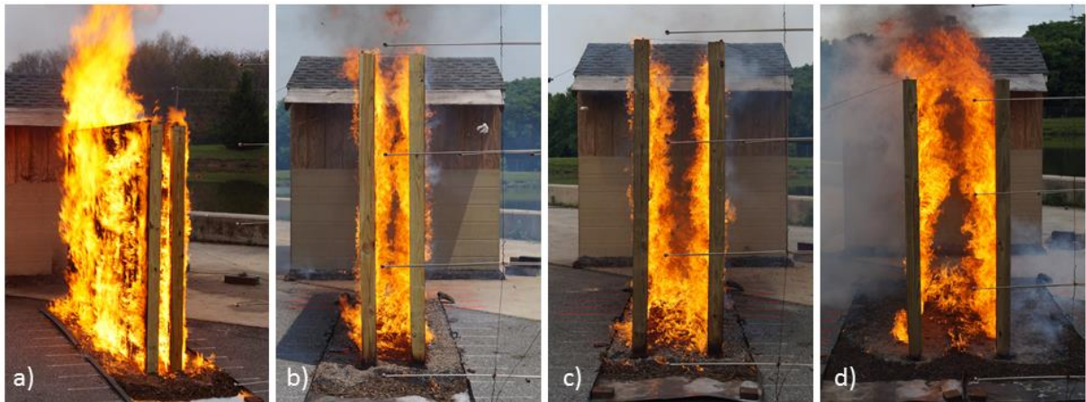
Fig. 122. Fire behavior of parallel WRC privacy fences at fence panel spacings of a) 20 cm [Test B-82], b) 30 cm [Test C-5], c) 46 cm [Test C-6], and d) 61 cm [Test C-7].
