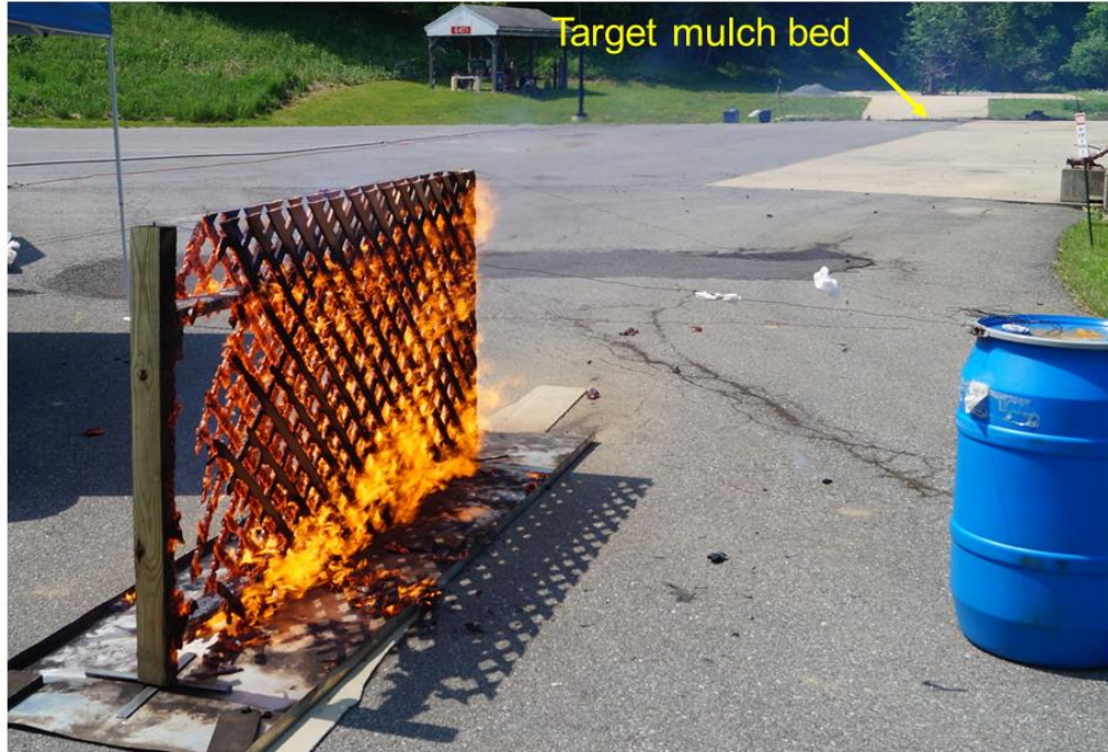
Fig. 148. Double lattice fence experiment without a structure and with a target mulch bed situated 47.6 m (156 ft) from the downwind end of the fence [Test C-3].
