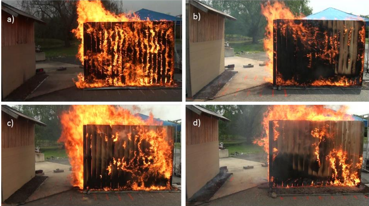
Fig. 121. Flames extending above and downwind of parallel WRC privacy fences at fence panel spacings of a) 20 cm at t = 5:00 [Test B-82], b) 30 cm at t = 5:00 [Test C-5], c) 46 cm at t = 4:00 [Test C-6], and d) 61 cm at t = 14:30 [Test C-7].
