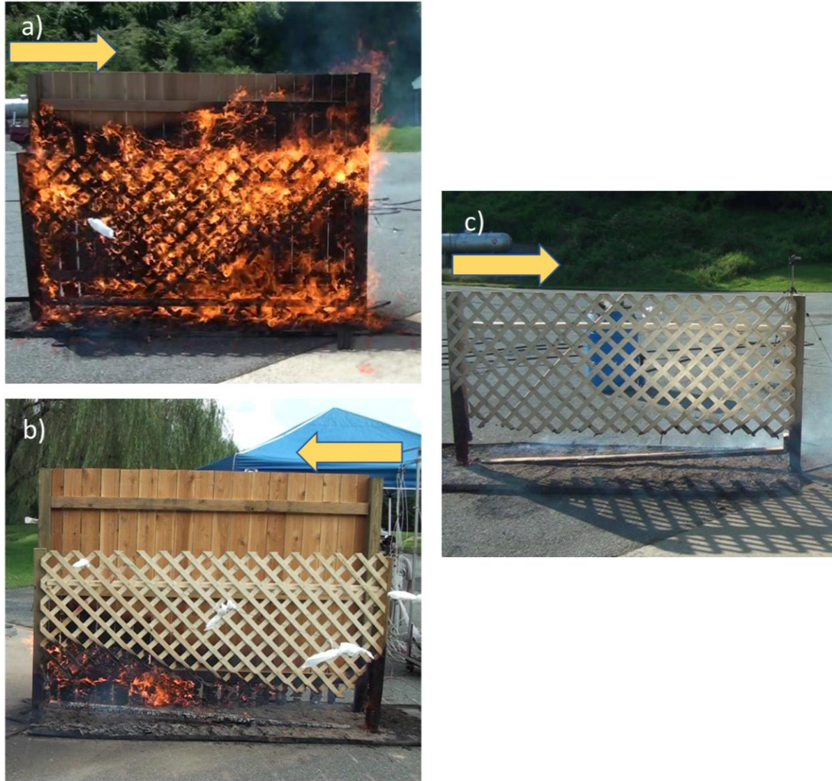
Fig. 141. Comparison of flame spread patterns for WRC privacy fence parallel to pine lattice fence at spacings of a) 31 cm (12 in) [Test D-8] and b) 46 (18 in) [Test C-17] with c) single panel PL fence [Test C-21] . Arrows indicate wind direction.
