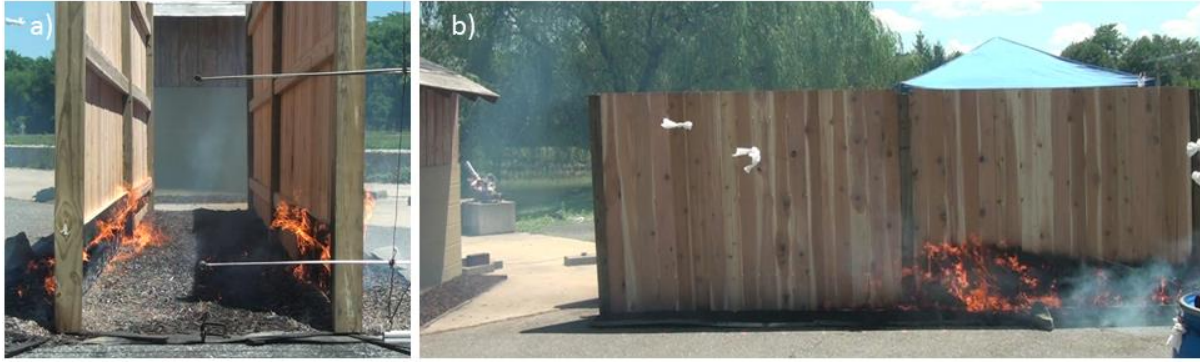
Fig. 124. Fire behavior at t = 5:00 for two-panel length parallel privacy fences at 91 cm spacing [Test C-13].
