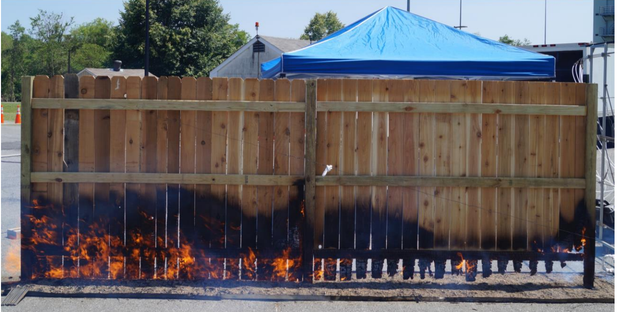
Fig. 80. Two-panel length western redcedar fence combined with shredded hardwood mulch without a structure downwind, at about t = 12 min [Test D-3].
