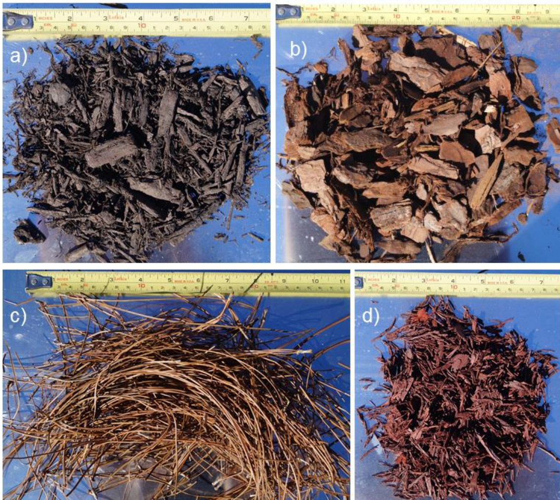
Fig. 8. Mulch types: a) shredded hardwood mulch, b) mini pine bark nuggets, c) pine straw, and d) shredded rubber mulch.
