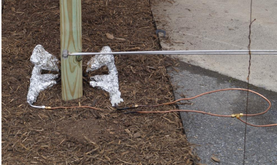
Fig. 15. Propane burner protected by Kaowool blanket and aluminum foil.
