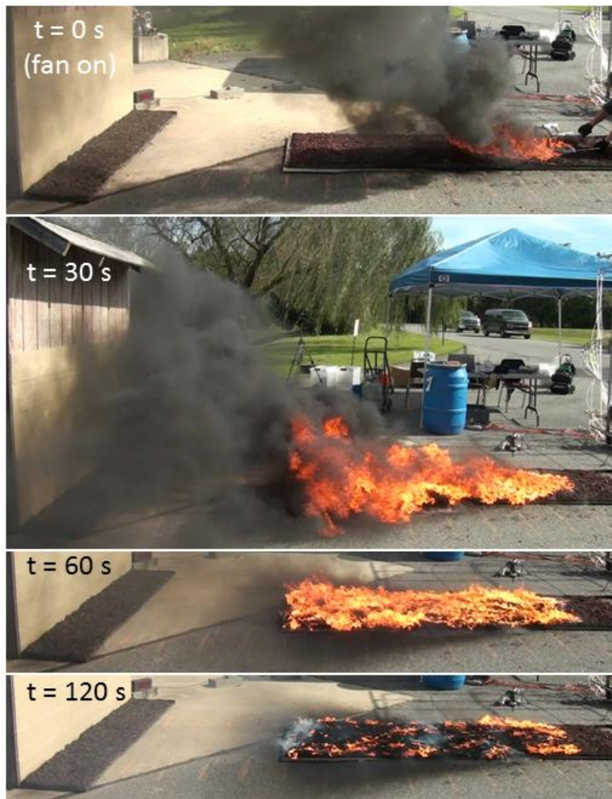
Fig. 43. Time sequence for rubber mulch bed in medium wind speed [ Test C-27 ].
