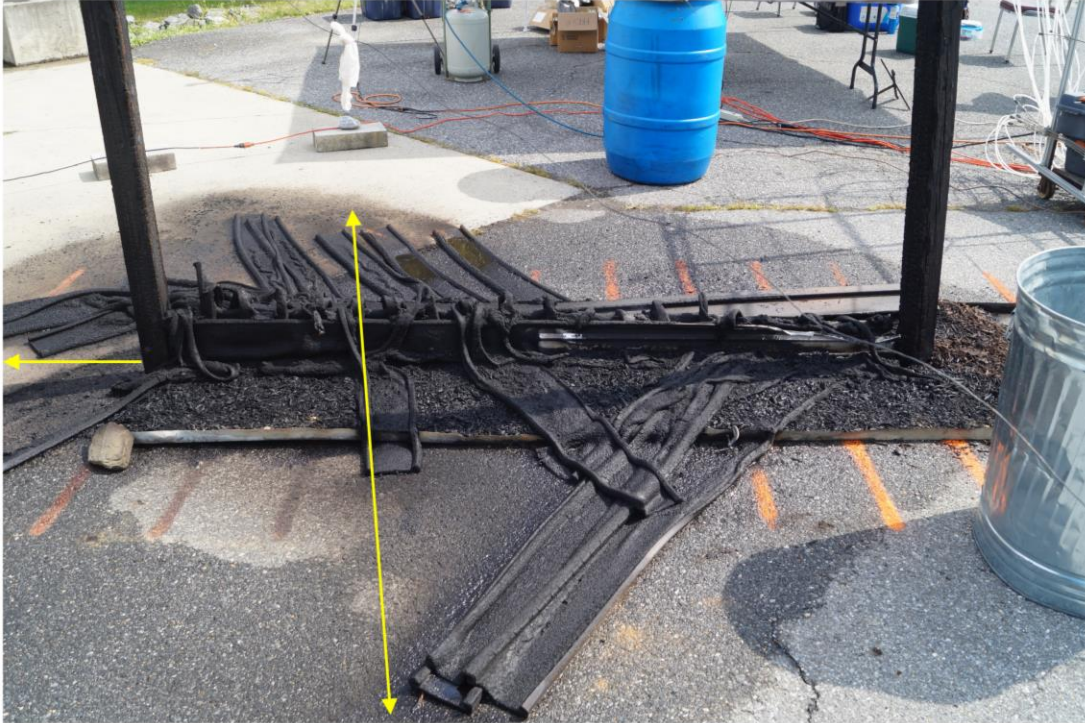
Fig. 98. Final configuration of wood-plastic composite boards after Test E-1 . Yellow arrows highlight the final positions of fallen fence boards.
