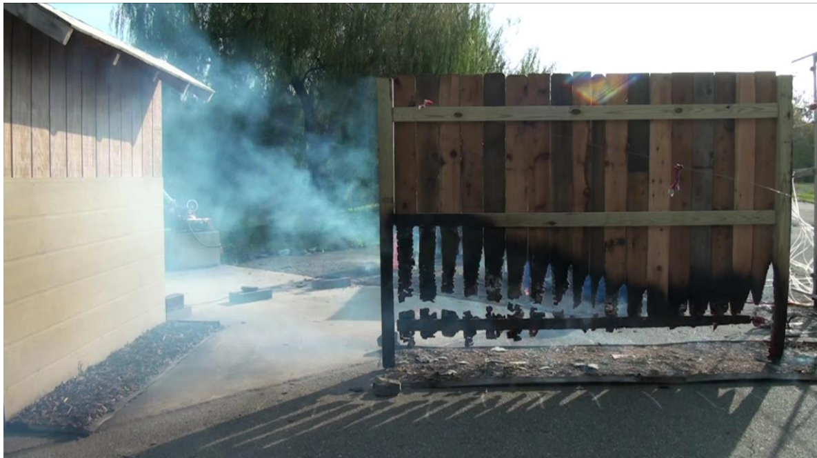
Fig. 78. Single panel western redcedar fence combined with shredded hardwood mulch, at low wind speed and 1.83 m (6 ft) separation distance [Test A-102], at t = 20 min.
