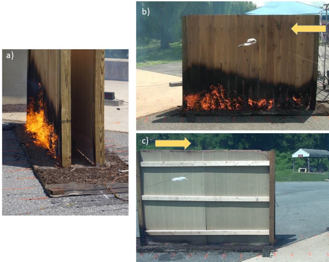
Fig. 132. Cement board (noncombustible) parallel to WRC privacy fence with 31 cm (12 in) spacing, near end of experiment ( t = 6 min), in camera views from a) near the fan, b) left side, and c) right side [Test D-7]. Arrows indicate wind direction.
