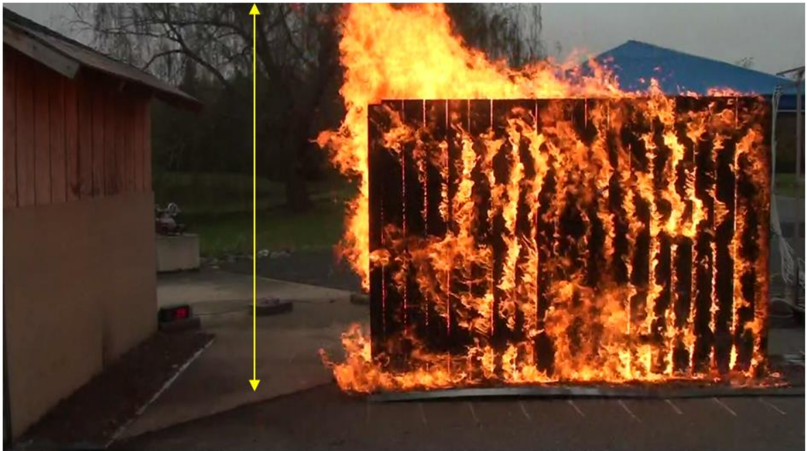
Fig. 118. Parallel western redcedar privacy fences with shredded hardwood mulch at 20 cm (8 in) spacing and low wind speed, at t = 5 min [Test B-82].
