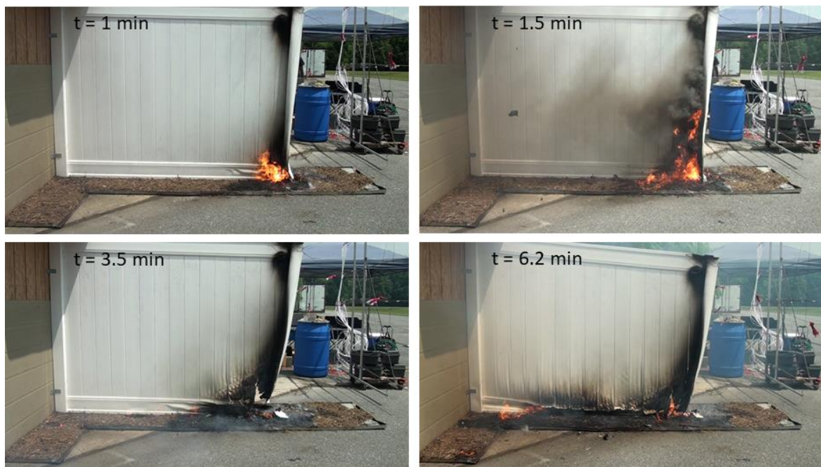
Fig. 89. Image sequence for vinyl privacy fence attached to wall with medium wind speed [ Test A-35 ].
