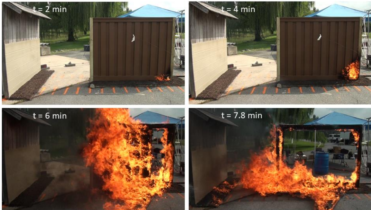
Fig. 97. Time sequence for wood-plastic composite fence #1 at low wind speed and 1.83 m (6 ft) separation distance [Test E-1].
