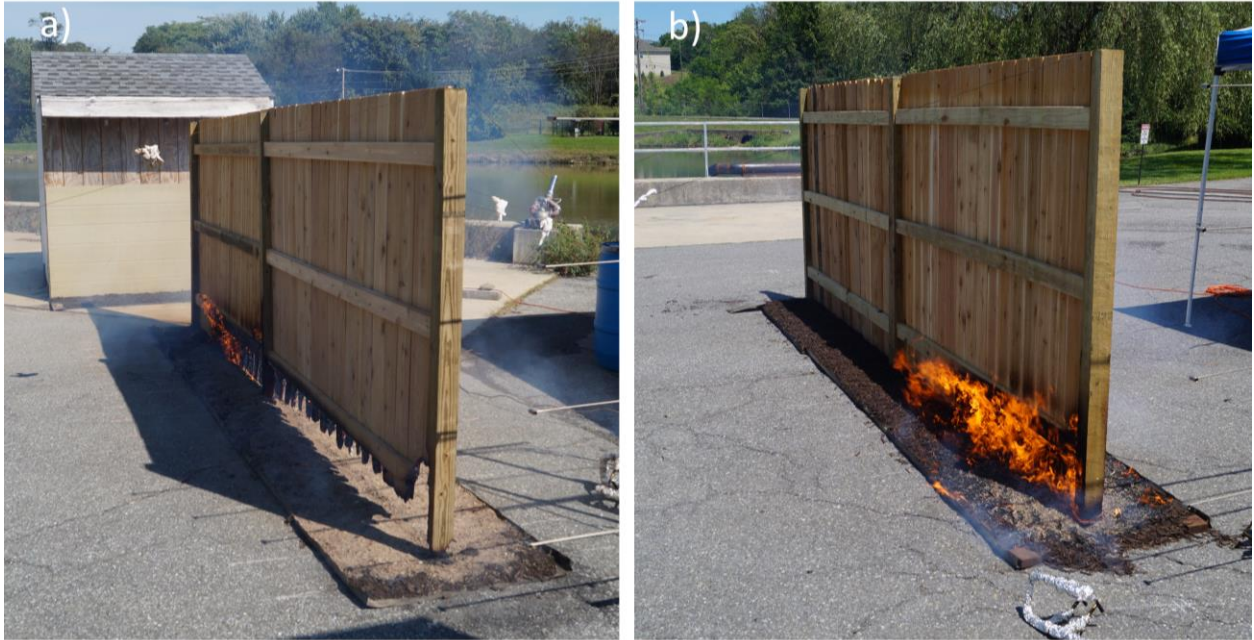
Fig. 76. Set-up for two-panel length western redcedar fence combined with shredded hardwood mulch a) with and b) without a structure downwind [ Tests C-19 and D-3 , respectively].
