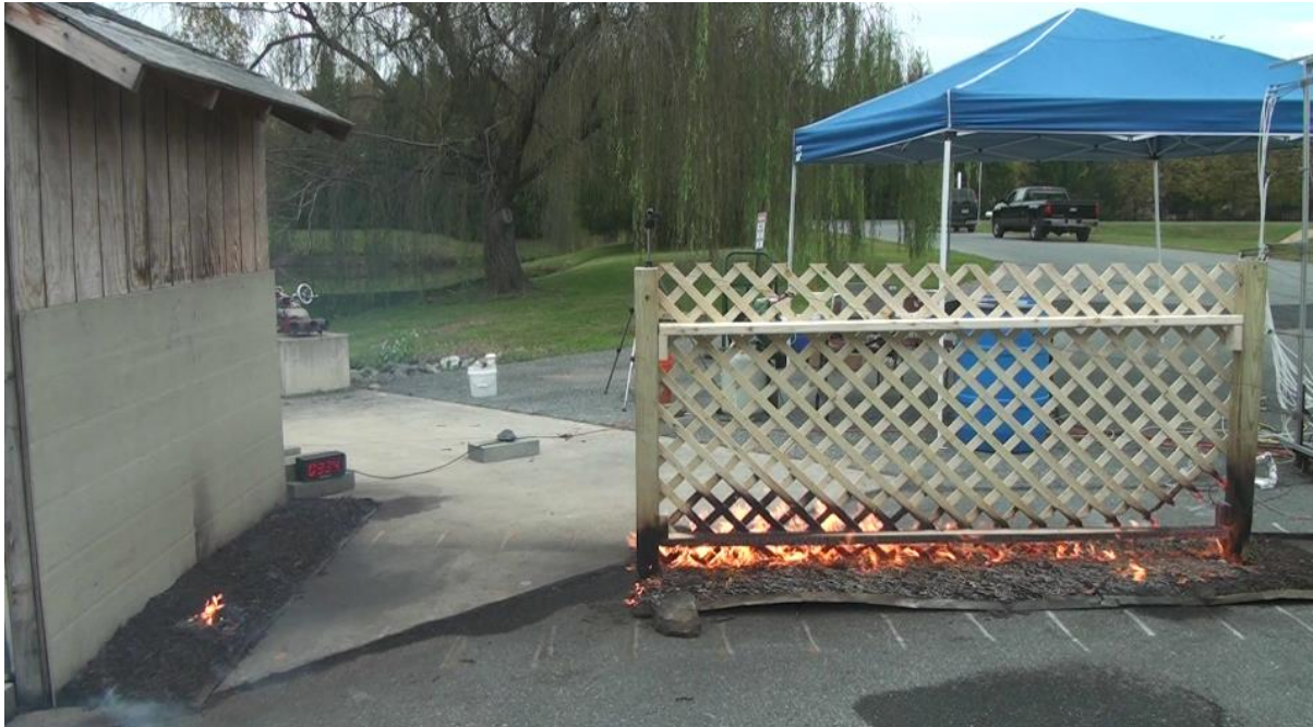
Fig. 92. Pine lattice fence combined with shredded hardwood mulch, 3 ½ min after fan on, at medium wind speed [Test B-81].
