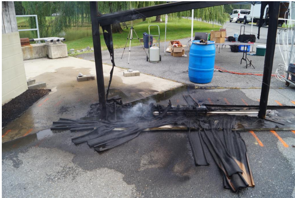
Fig. 64. Final configuration of wood-plastic composite boards after Test E-2 .
