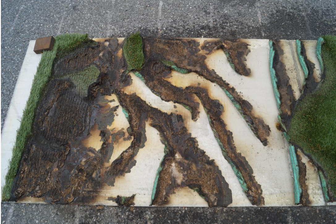
Fig. 48. Curled segments and char residue after burning of artificial turf [Test D-23].
