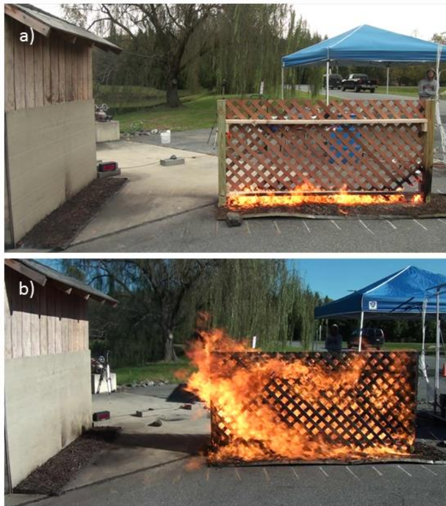
Fig. 115. Comparison of a) single ( Test B-79 at t = 3 min) and b) double ( Test B-75 at t = 1.5 min) RW lattice fences in medium wind speeds.
