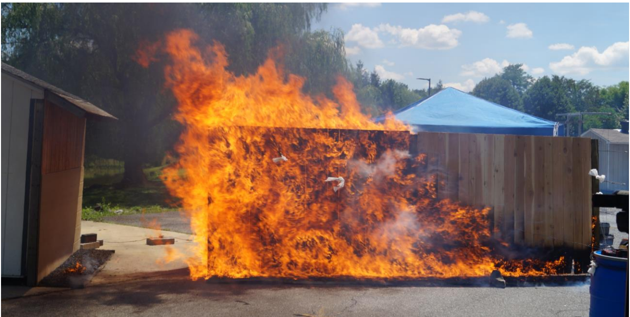
Fig. 125. Fire behavior at t = 6:15 for two-panel length parallel privacy fences at 91 cm spacing [Test C-13].
