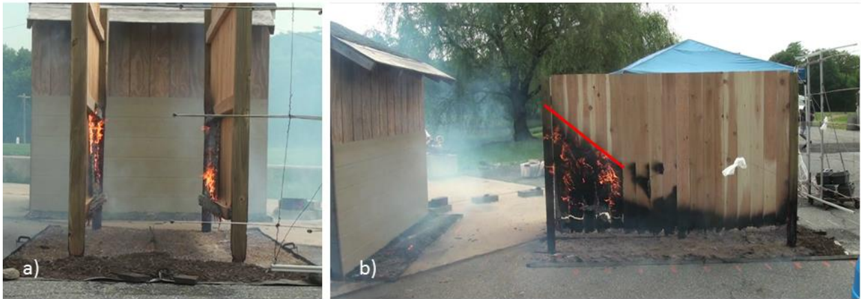
Fig. 123. Fire behavior for parallel privacy fences spaced apart by 91 cm [Test C-8] showing a) end view and b) left side view at t = 18:00 .
