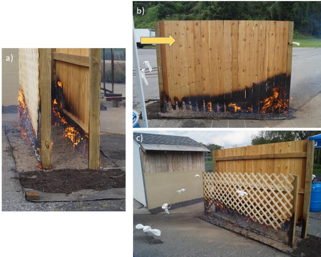
Fig. 139. Pine lattice fence parallel to western redcedar privacy fence with 46 cm (18 in) spacing, near end of test, in camera views from a) near the fan, b) right side, and c) left side [Test C-17].
