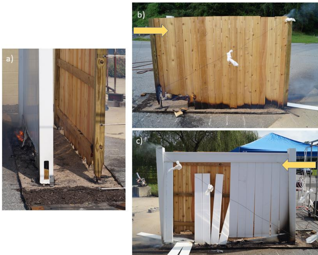
Fig. 136. Vinyl privacy fence parallel to western redcedar privacy fence near end of test in camera views from a) near the fan, b) right side, and c) left side [ Test C-16 ].
