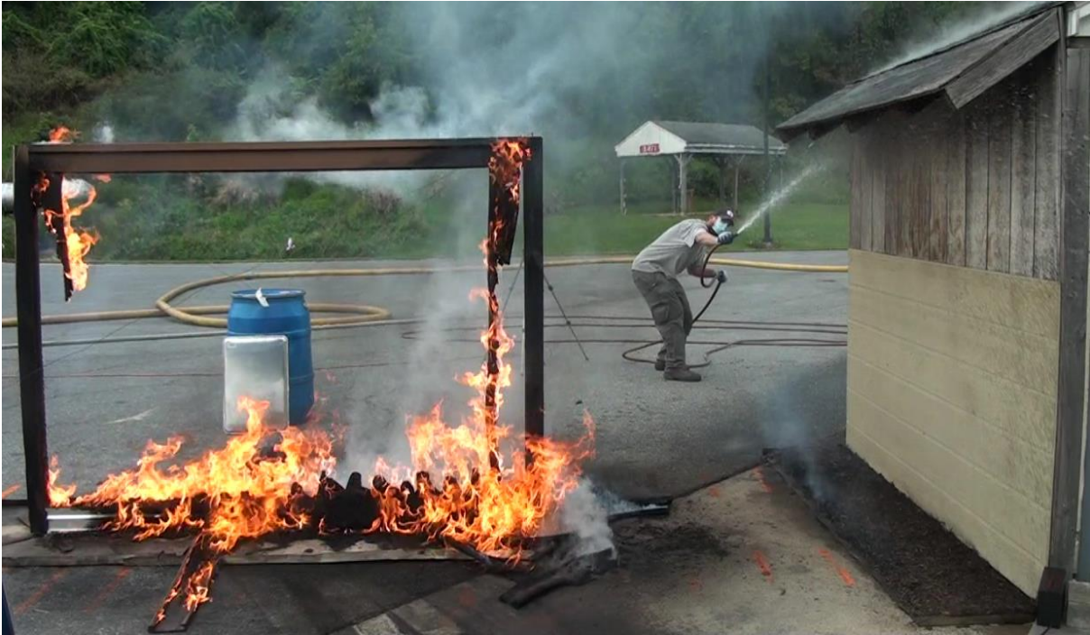
Fig. 65. Water being applied to the eaves of the shed after Test E-2 . Smoke rising from the roof is visible.
