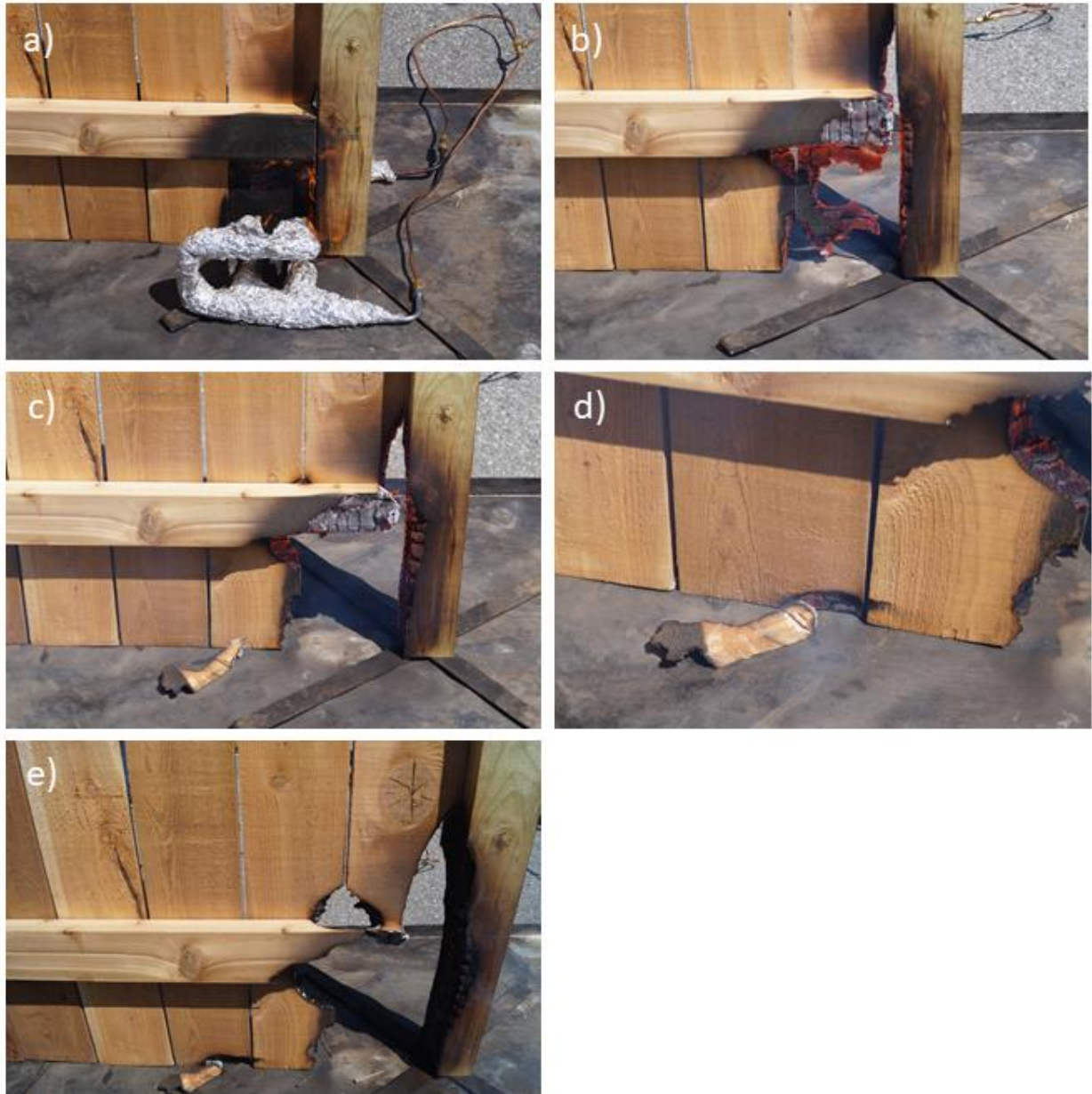
Fig. 55. Progression of glowing combustion over western redcedar privacy fence in high wind speed [Test A-26], showing a) ignition, b) erosion of board at t = 2.5 min, c) large firebrand at t = 4.5 min, d) secondary ignition by firebrand at t = 7.5 min, and e) burn pattern at t = 11.5 min.
