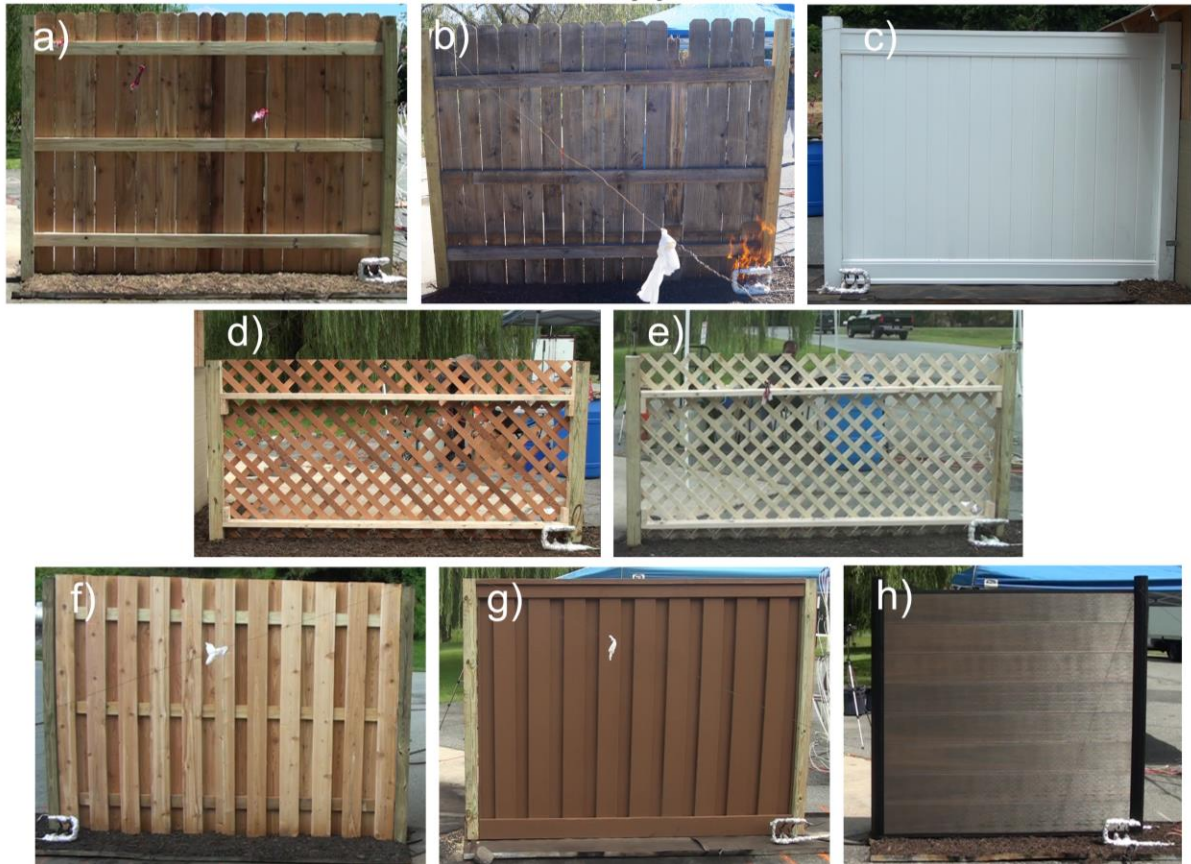
Fig. 11. Fence types: a) western redcedar privacy, b) aged privacy, c) vinyl privacy, d) redwood lattice, e) pressure treated pine lattice, f) western redcedar good neighbor, g) wood-plastic composite #1, and h) wood-plastic composite #2.
