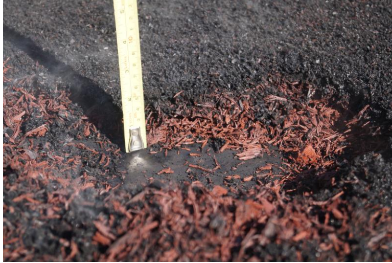
Fig. 44. Shredded rubber mulch extinguished after 6 min, showing upper layer of crumbly residue and lower layer of virgin material.
