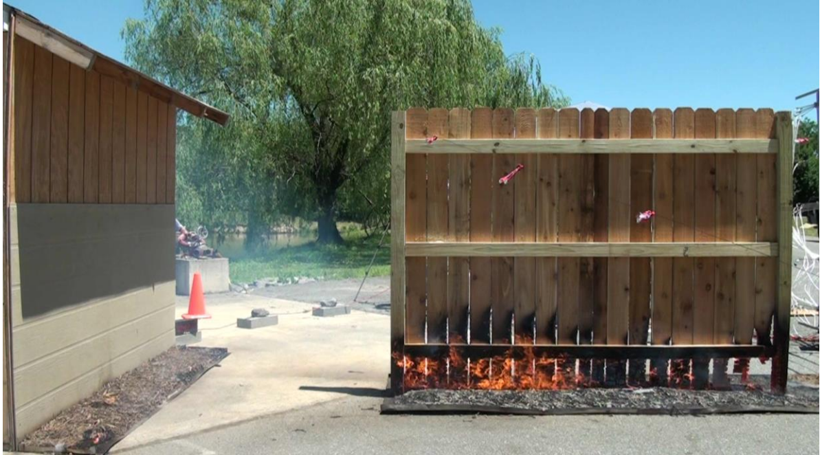
Fig. 85. WRC privacy fence with HW mulch at medium wind speed, at about t = 4 \frac{1}{2} min [Test A-29].
