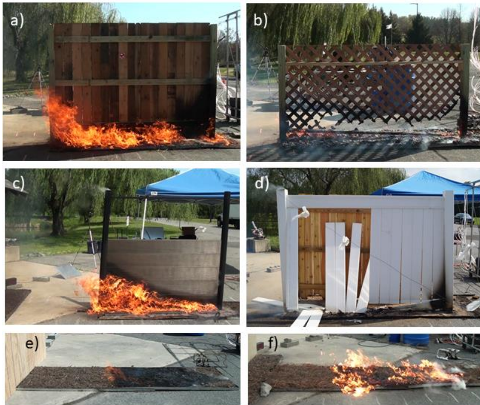
Fig. ES.3. Examples of High Hazard fence and mulch configurations: a) western redcedar (WRC) privacy fence with pine straw mulch, b) redwood lattice fence with shredded hardwood (HW) mulch, c) wood-plastic composite #2 fence with HW mulch, d) WRC privacy fence parallel to vinyl privacy fence, e) HW mulch f) pine straw mulch.
