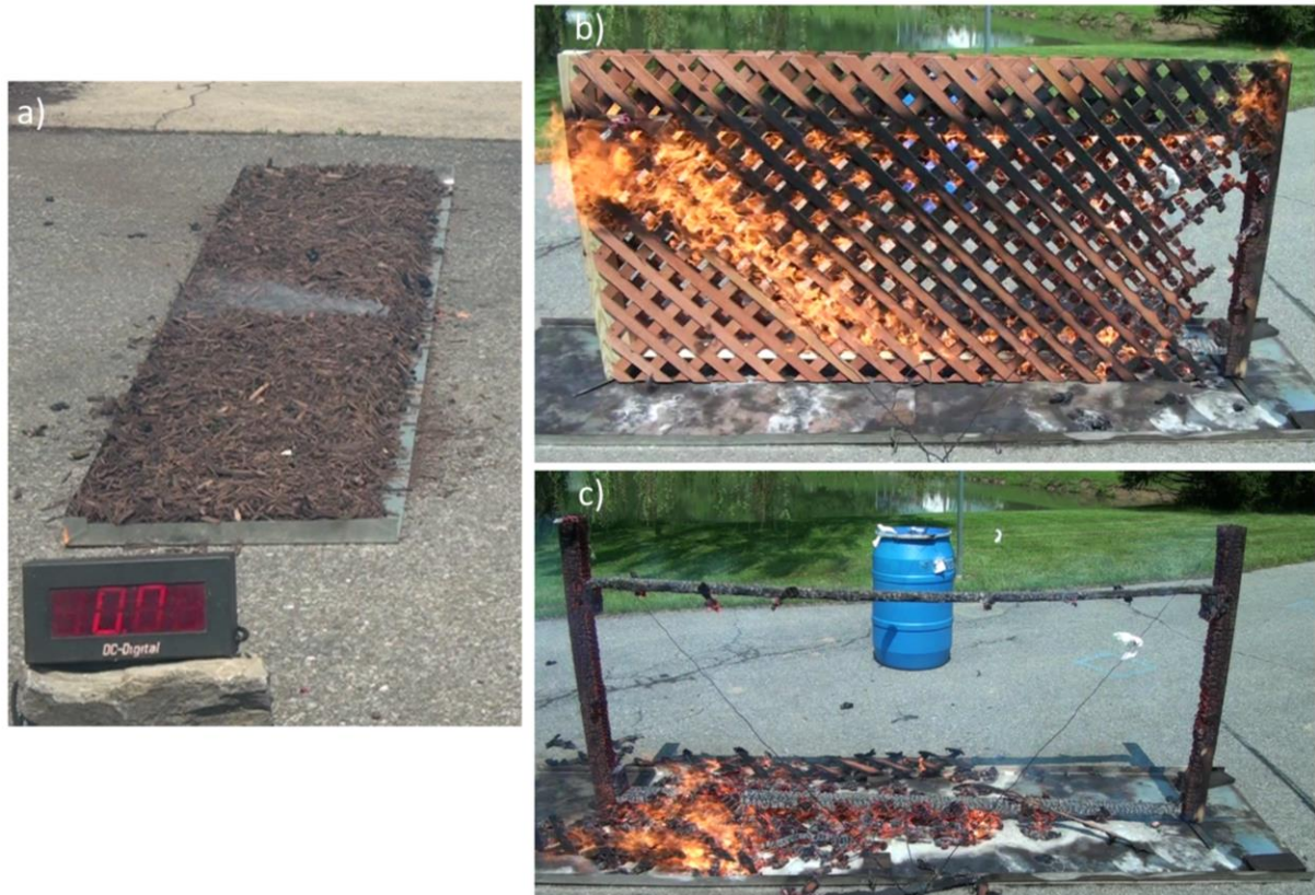
Fig. 150. Spot fire ignition resulting from double redwood lattice fence, showing a) the target mulch bed at t = 10 min, after 2 min at high wind speed, and the double lattice fence at b) t = 7 min and c) t = 10 min after the fan was turned on [Test C-3].
