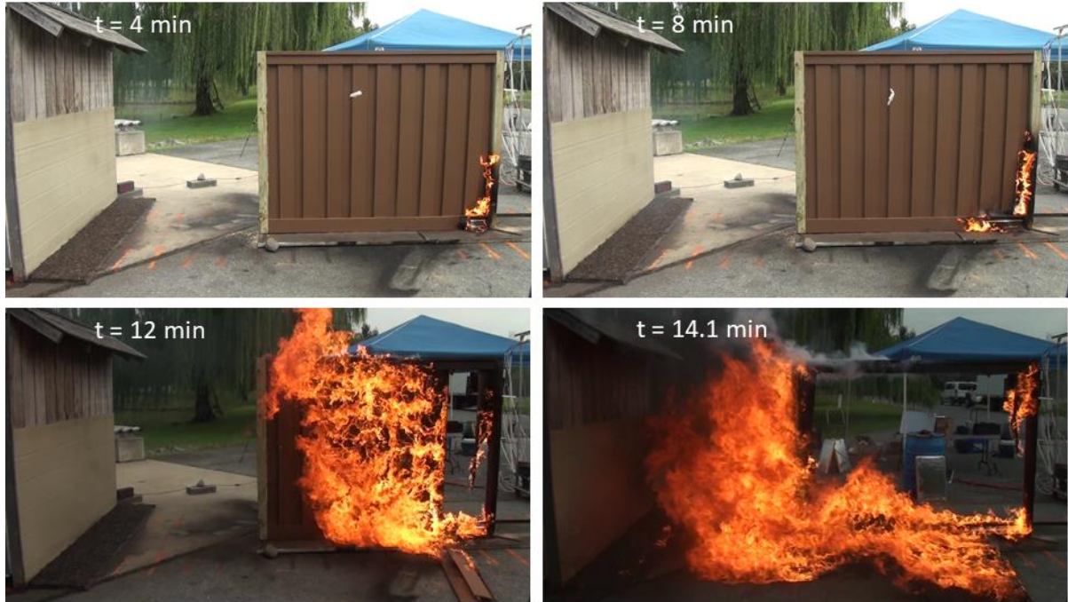
Fig. 63. Time sequence for Test E-2 , wood-plastic composite fence WPC1 alone (without mulch), with low wind speed at 1.83 m (6 ft) separation from shed.
