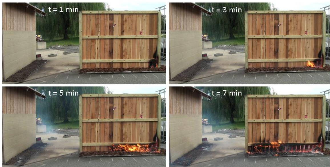
Fig. 106. Time sequence for WRC privacy fence and PB mulch in medium wind speed [Test A-90].
