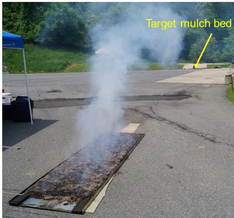
Fig. 149. Shredded hardwood mulch experiment without a structure and with a target mulch bed situated 47.0 m (154.5 ft) from the downwind end of the mulch bed [Test C-2].
