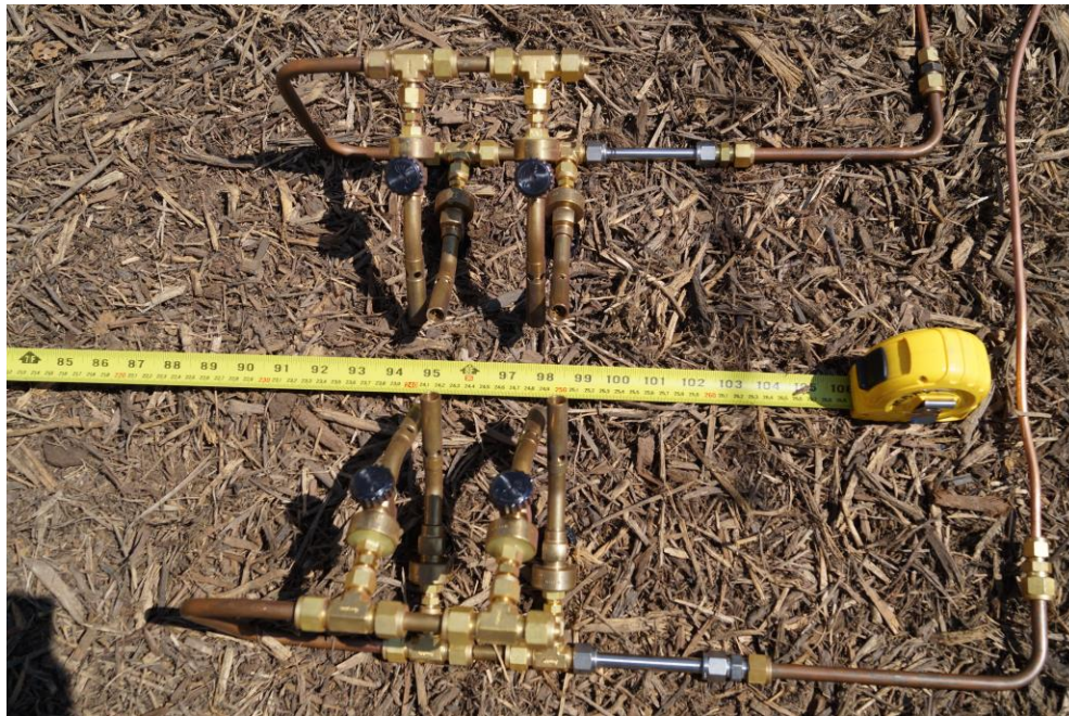
Fig. 14. Propane burner for igniting fence and/or mulch, with torches exposed.
