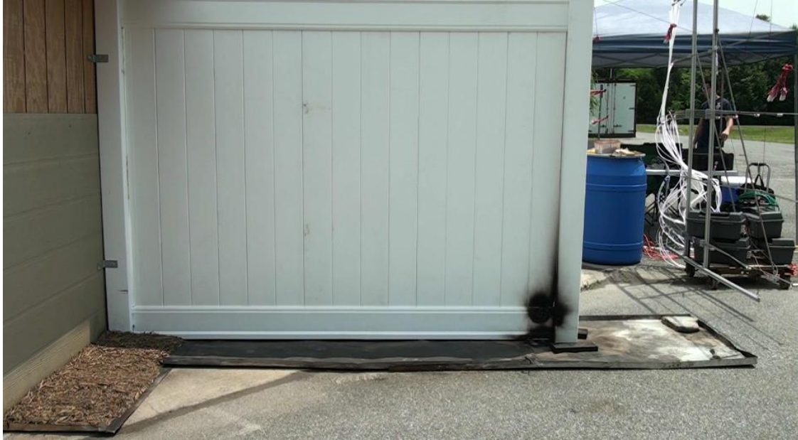
Fig. 62. Vinyl privacy fence in high wind conditions at 0 m separation distance [ Test A-34 ].
