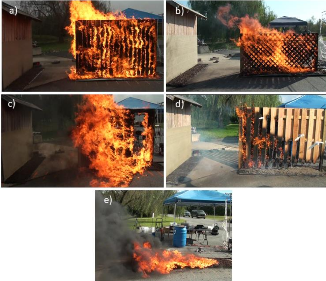
Fig. ES.2. Examples of Very High Hazard fences and mulch: a) parallel privacy fences, b) double lattice fences, c) wood-plastic composite #1 fence, d) good neighbor fence, e) rubber mulch.
