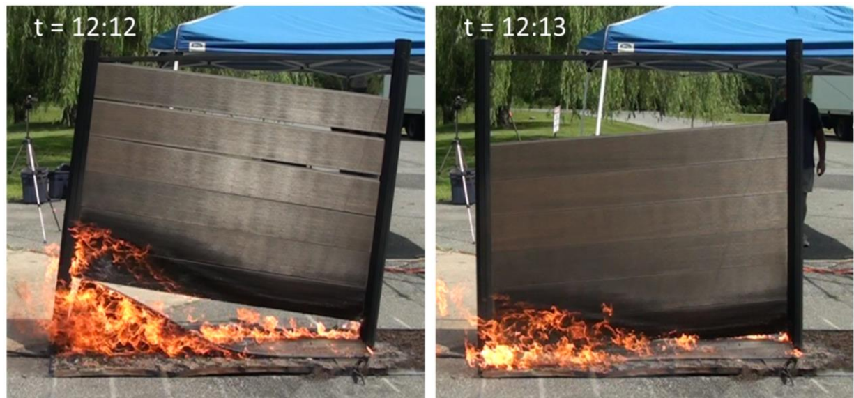
Fig. 100. Collapse of horizontal planks shortly after t = 12 \text{ min} [Test F-1].
