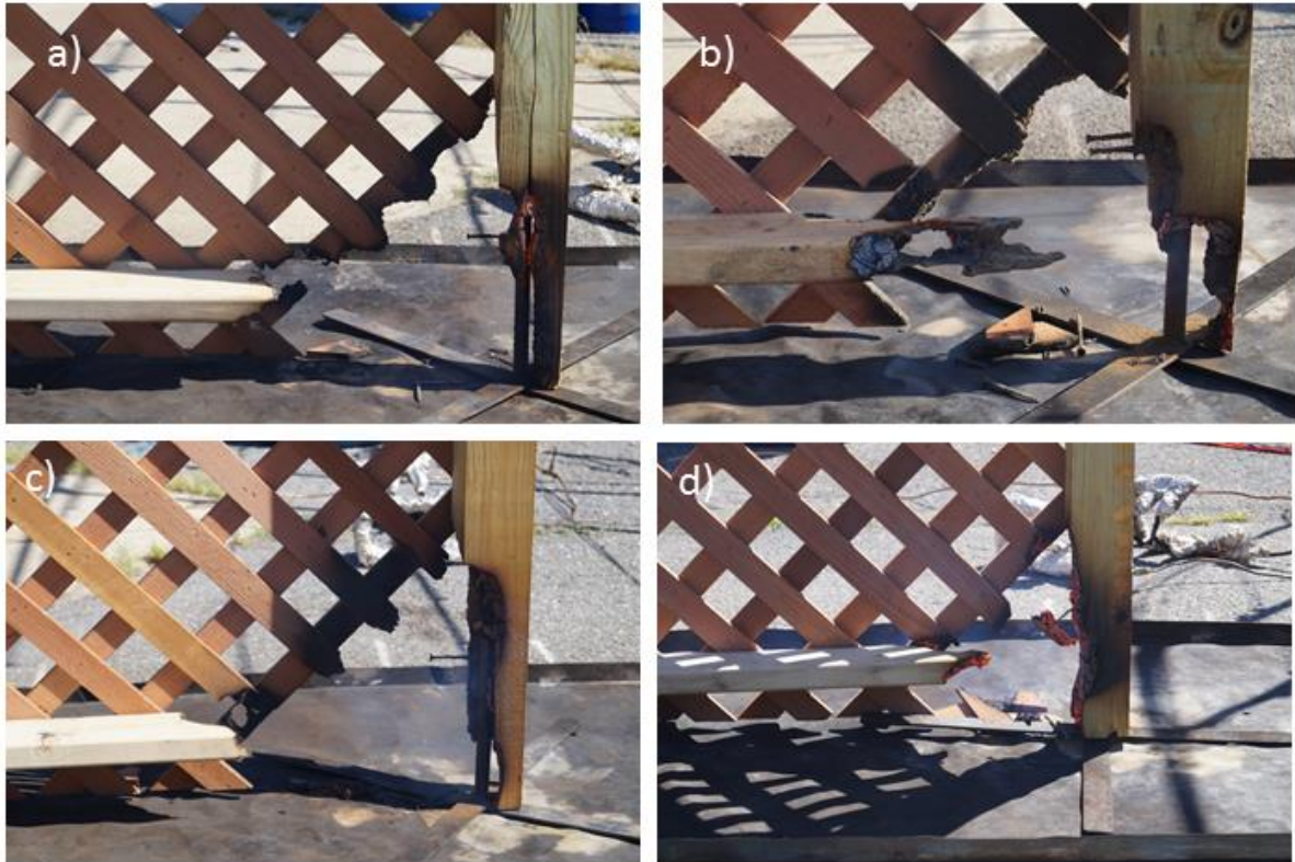
Fig. 61. Redwood lattice fence only, in medium wind speed at separation distances of a) 0 m [Test A-82], b) 0.30 m (1ft) [Test A-113], c) 0.91 m (3 ft) [Test A-77], and d) 1.83 m (6 ft) [Test A-75].
