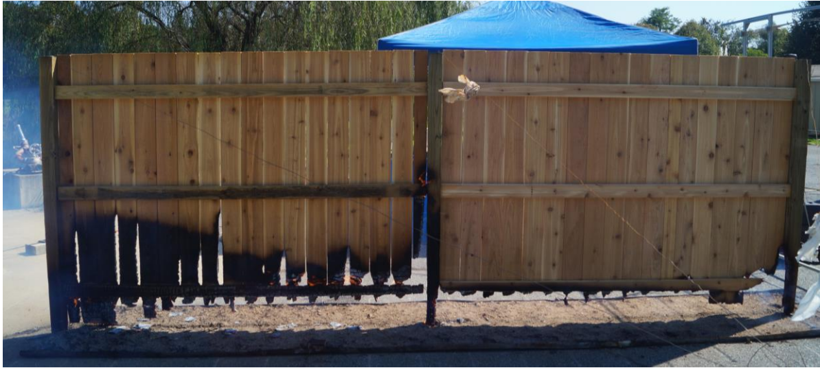
Fig. 77. Two-panel length western redcedar fence combined with shredded hardwood mulch, at low wind speed and 1.83 m (6 ft) separation distance [Test C-19], at t = 45 min.
