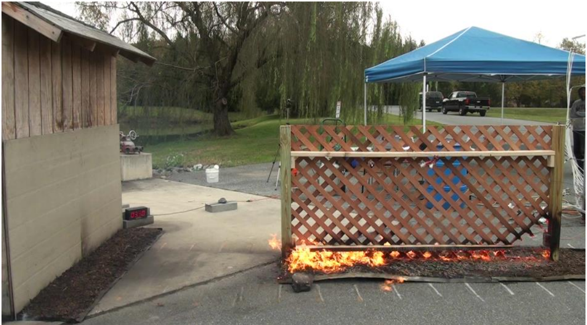
Fig. 90. Redwood lattice fence combined with shredded hardwood mulch, 3½ min after fan on, at medium wind speed [Test B-79].
