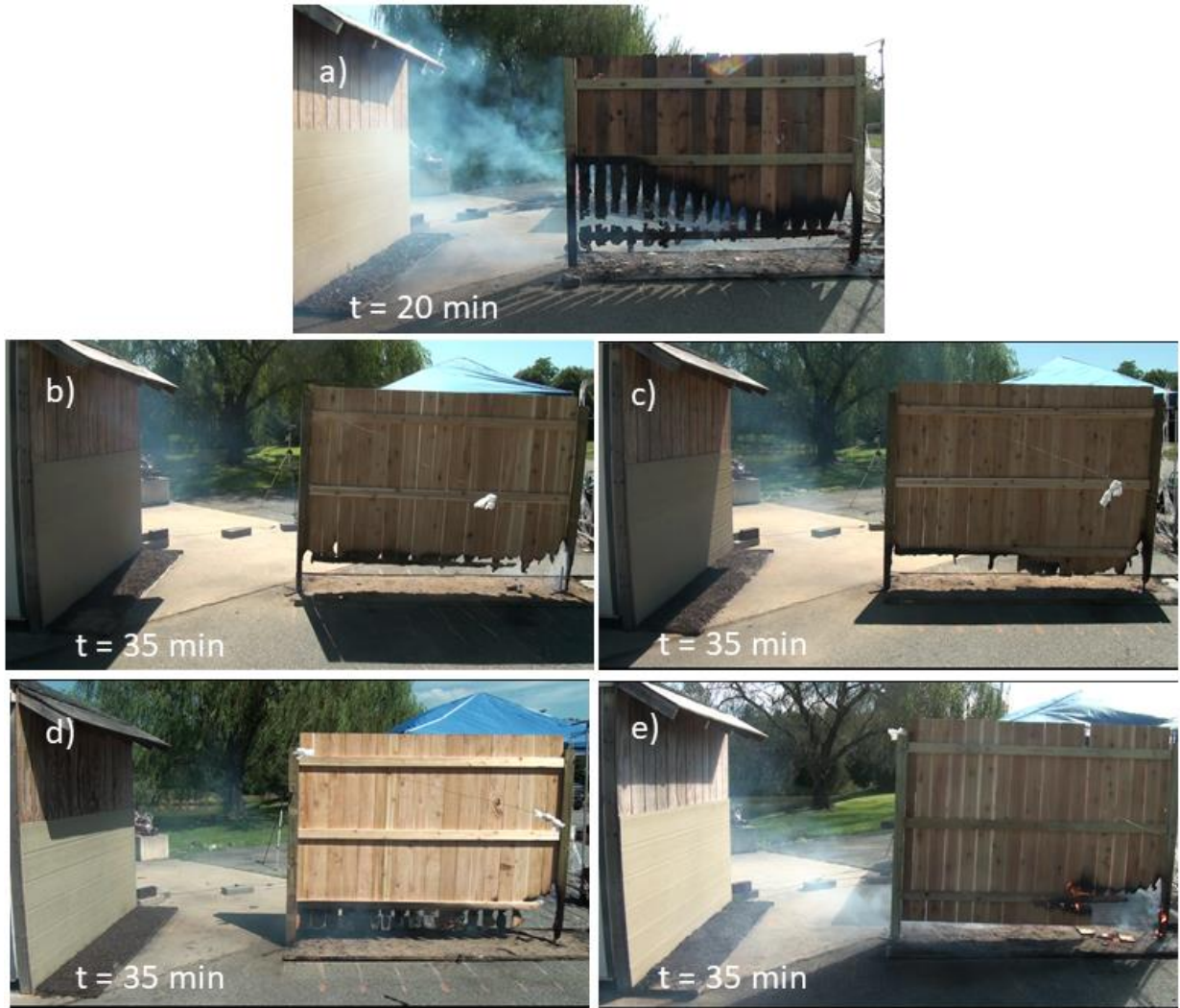
Fig. 83. Comparison of results from privacy fences raised above the hardwood mulch pan by a) 0 cm [ Test A-102 ], b) 5.1 cm (2 in) [ Test C-10 ], c) 7.6 cm (3 in) [ Test C-11 ], d) 10.2 cm (4 in) [ Test C-14 ], and e) 15.2 cm (6 in) [ Test C-28 ].
