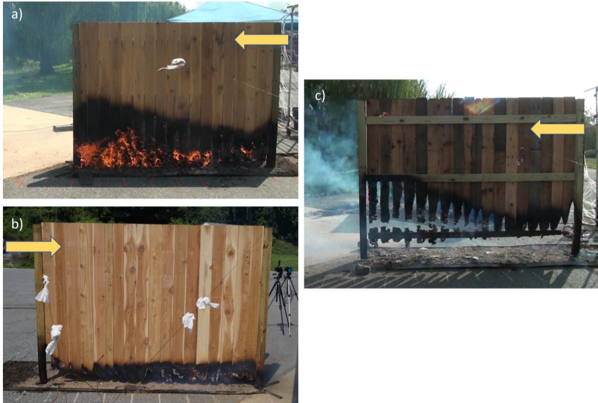
Fig. 134. Comparison of char patterns near the end of experiments with parallel WRC fence / cement board at a) 31 cm (12 in) spacing [Test D-7] and b) 46 cm (18 in) spacing [Test C-15] and c) single WRC panel [Test A-102]. Arrows indicate wind direction.
