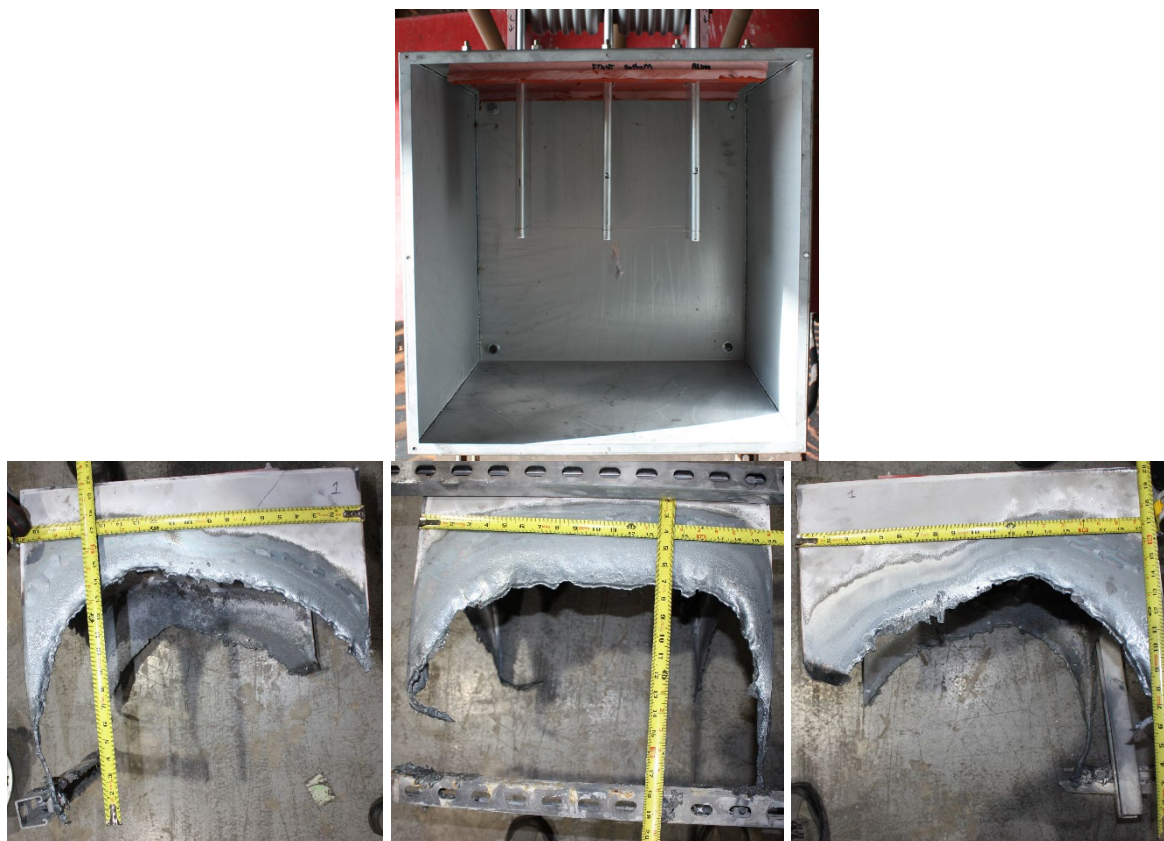
Fig. 60. Experiment OBMV01 pre-experiment (top) and post-experiment (left side (bottom left), back (bottom center), right side (bottom right)). Phase sequence from left to right is C-B-A.
