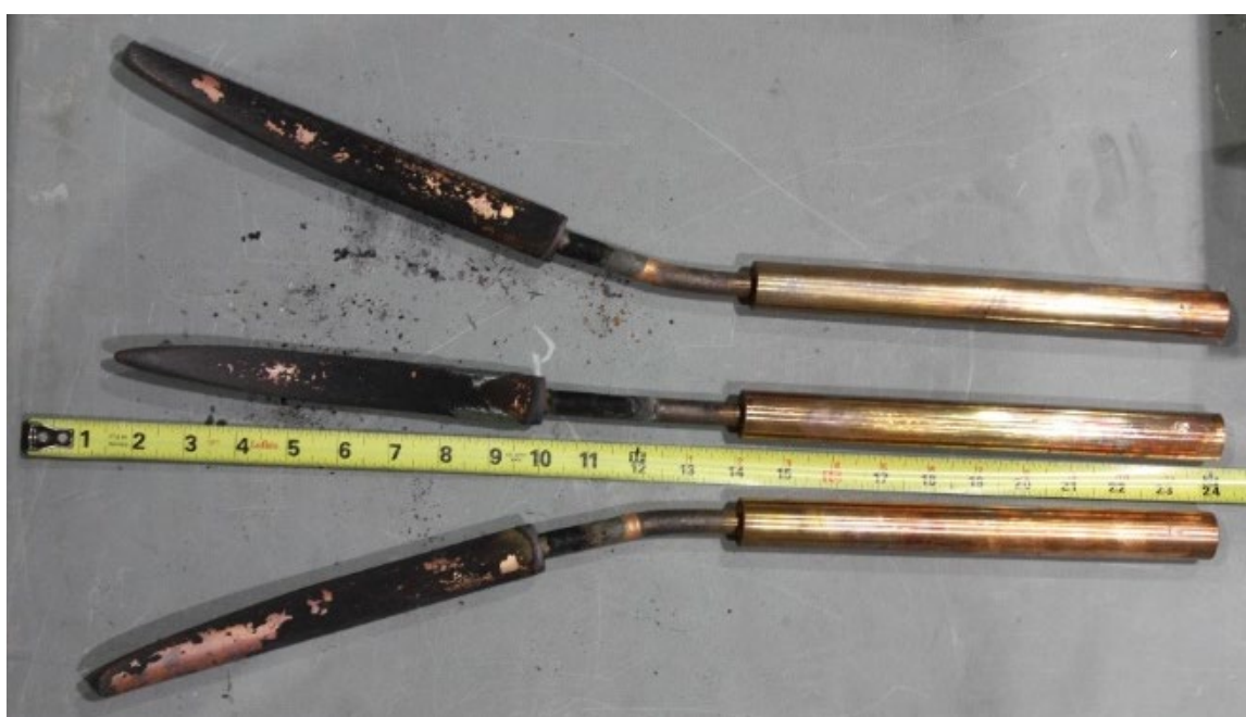
Fig. 38. Experiment OB04 electrode deflection post-experiment.
