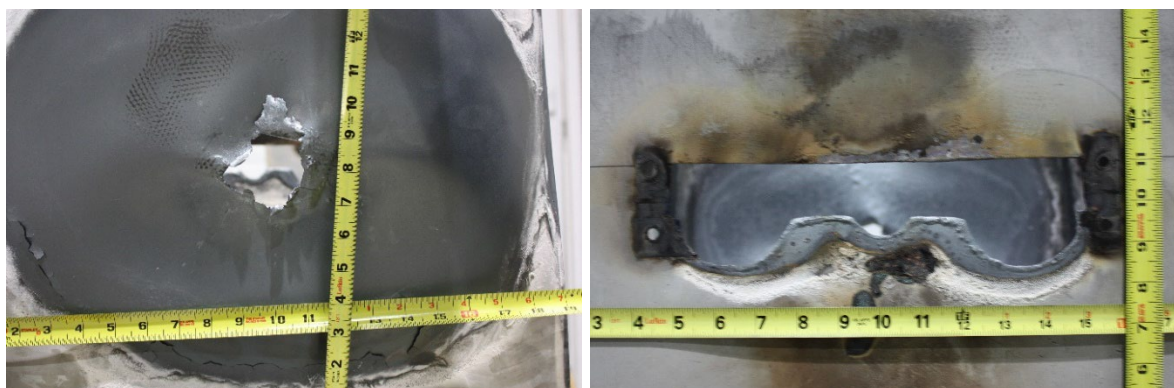
Fig. 37. Experiment OB04 enclosure breach (bottom side (left); top side (right)).
