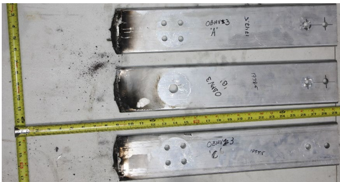
Fig. 71. Experiment OBMV03 aluminum electrode post-experiment.
