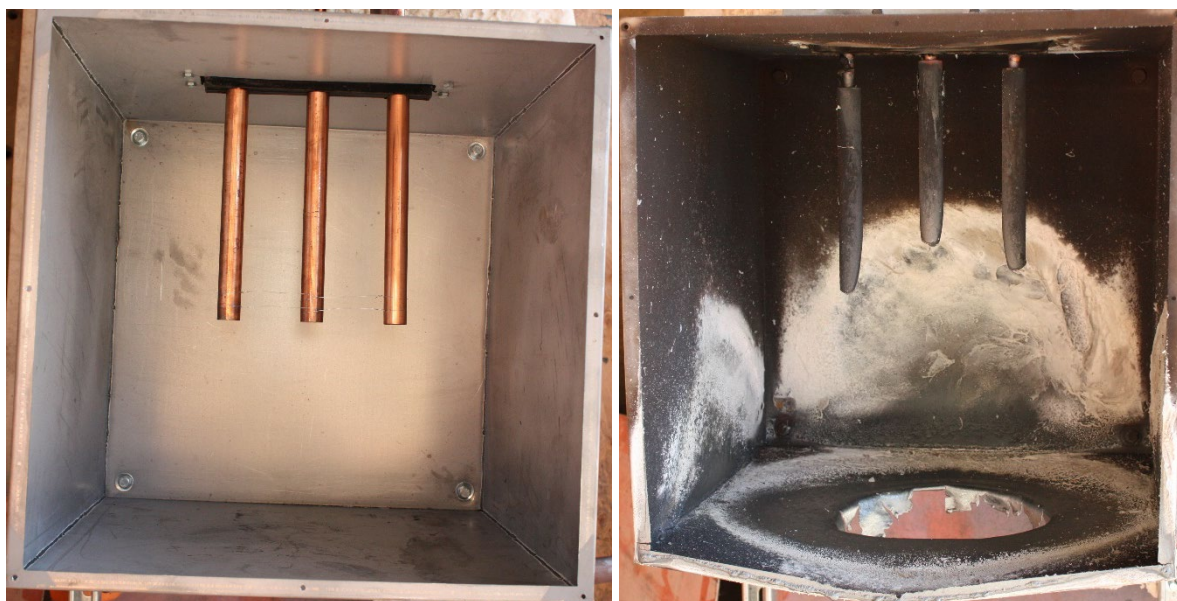
Fig. 30. Experiment OB02 pre-experiment (left) and post-experiment (right) copper electrodes. Phase sequence from left-to-right is C-B-A.
