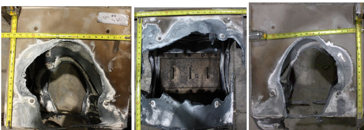
Fig. 56. Experiment OBMV04 enclosure breach (Left-to-right: Right side, back side, left side).
