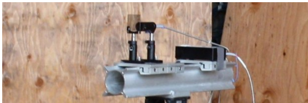
Fig. 7. The spectrometer is mounted to the top of the base plate.
