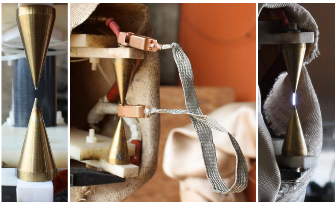
Fig. 19. Breakdown sensor (electrode configuration (left), safety jumper (center), operational experiment (right)).
