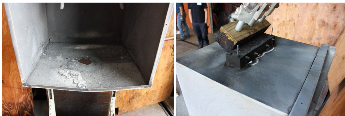
Fig. 50. Experiment OB08 enclosure breach (bottom and sides (left); rear top (right)).
