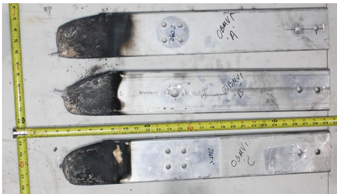
Fig. 61. Experiment OBMV01 aluminum electrode post-experiment.
