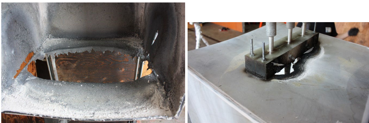
Fig. 45. Experiment OB06 enclosure breach (bottom and sides (left); rear top side (right)).
