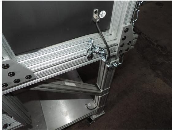
**Fig. 17.** The grounding connection on the lower right exterior for the spark ignitors.
