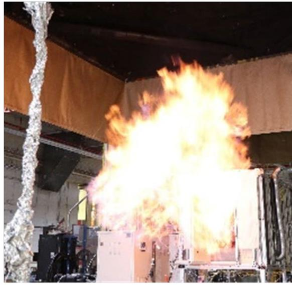
**Fig. 29.** A representative 25.0 kW methane fire after ignition (top, BSEE 61), a non-event after the front opens (bottom left, BSEE 61), and maximum flame extension during a backdraft event (bottom right, BSEE 52).
