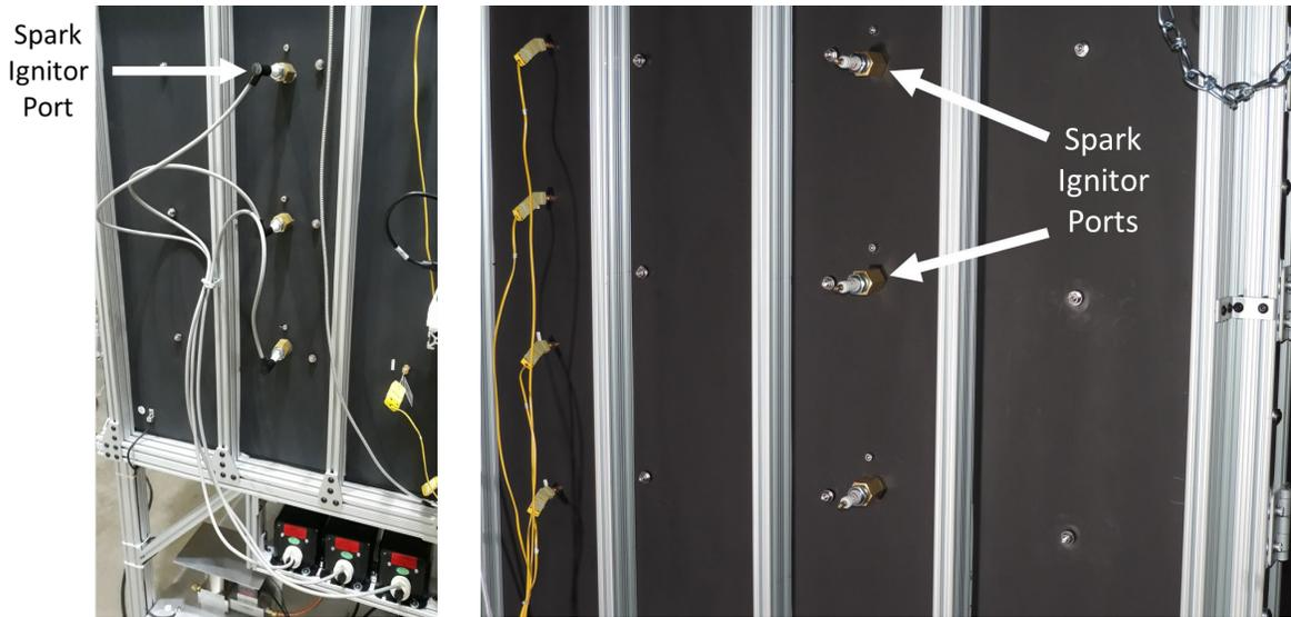
**Fig. 16.** The spark ignitor ports on the left exterior wall of the compartment with spark ignitors attached and electronics below the compartment (left) and the three spark ignitor ports with unattached spark ignitors aligned vertically on the right exterior wall of the compartment (right).
