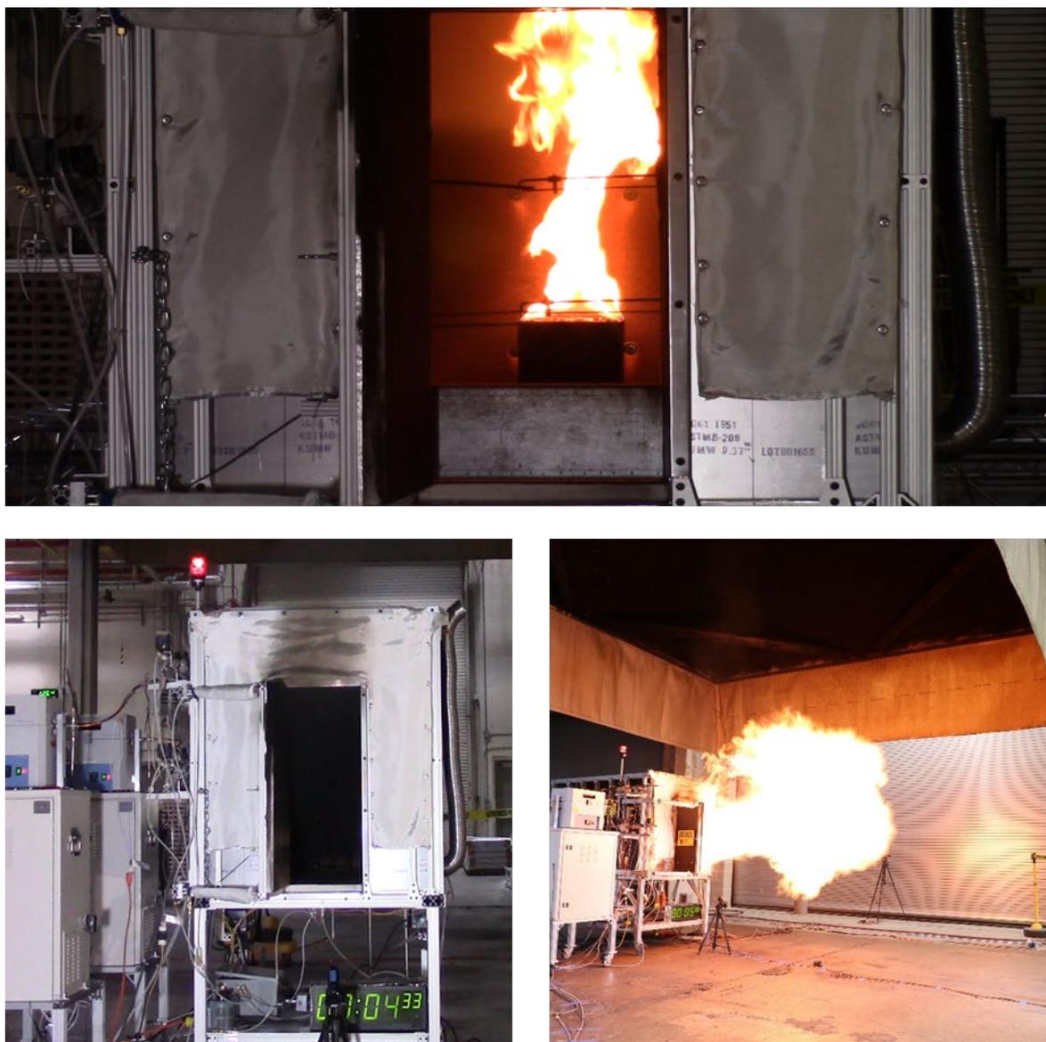
**Fig. 34.** A representative 25.0 kW propane fire after ignition (top, BSEE 132), a non-event after the front opens (bottom left, BSEE 132), and maximum flame extension during a backdraft event (bottom right, BSEE 167).
