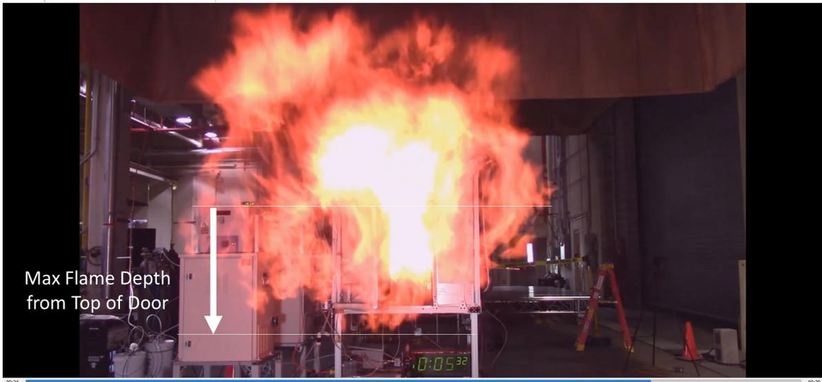
**Fig. 26.** Maximum vertical flame depth measurement from the top of the door from the front camera (BSEE 239).
