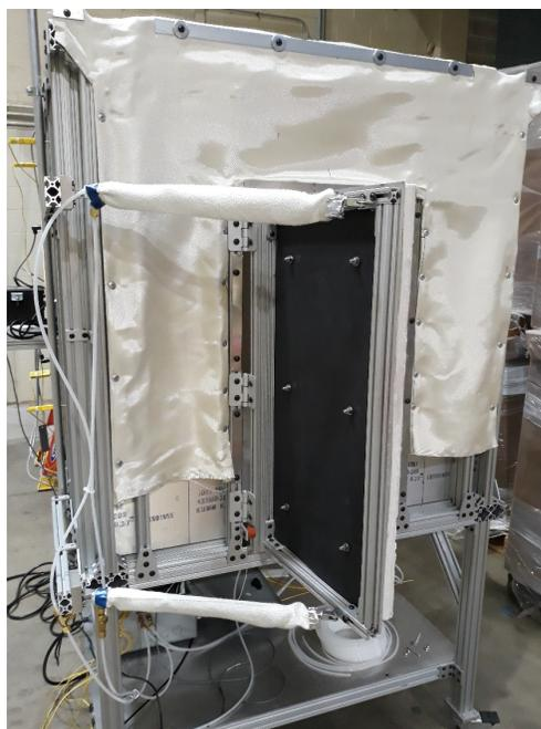
**Fig. 6.** The open front door with two pneumatic arms.
