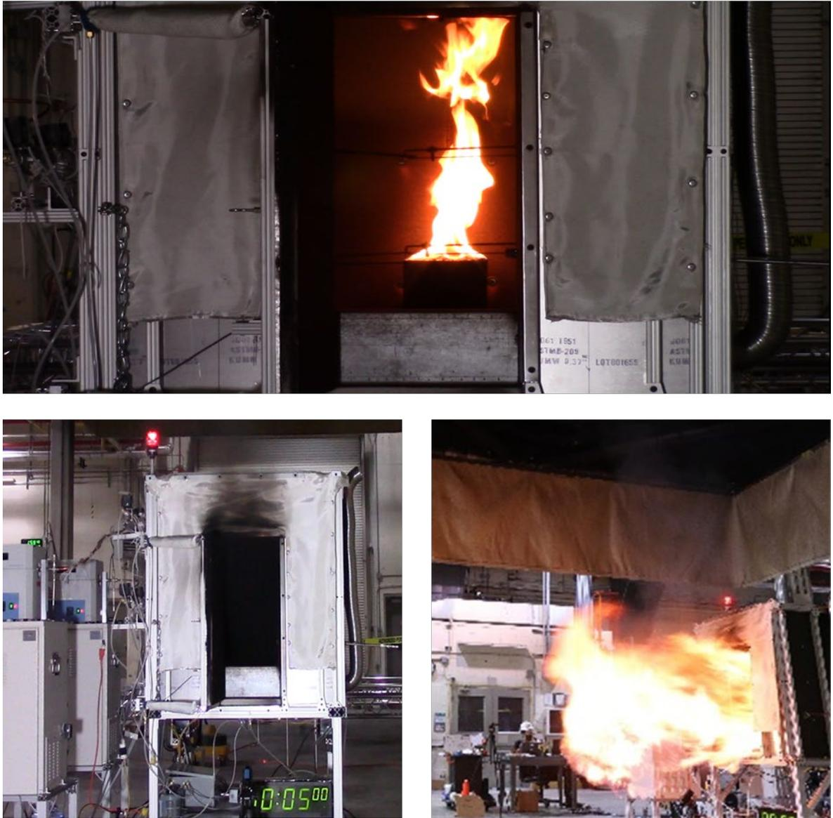
**Fig. 33.** A representative 16.7 kW propane fire after ignition (top, BSEE 203), a non-event after the front opens (bottom left, BSEE 203), and maximum flame extension during a backdraft event (bottom right, BSEE 191).
