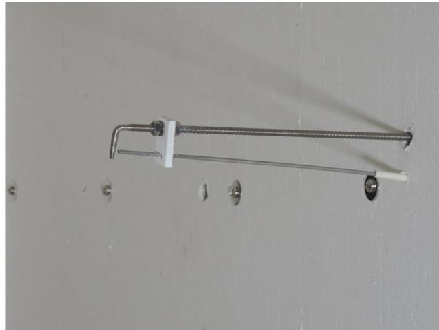
**Fig. 15.** One spark ignitor probe extending 5.4 cm out from the interior wall of the compartment (grounding rod positioned above).
