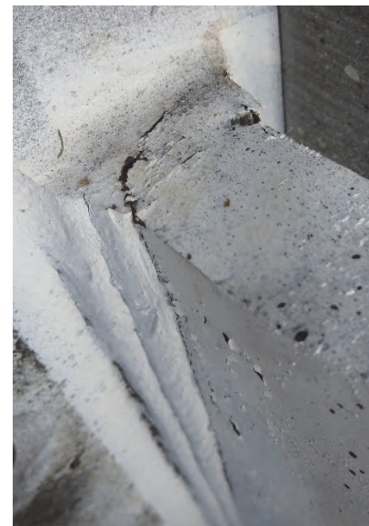
Figure 7.10 Specimen 21M-VAU: Column Flange CJP Weld Fracture
