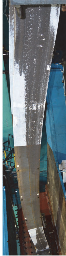
Figure 3.43 Specimen 1H: Out-of-Plane Global Buckling at End of Test (Side View)
