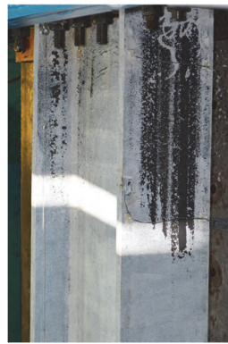
Figure 3.33 Specimen 1L: Yielding and Buckling Progression at Member Ends
