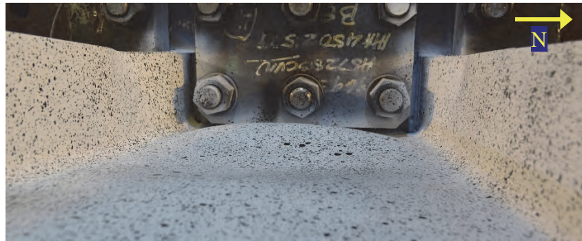
(c) Web Local Buckling at West End
