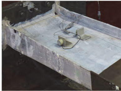
Figure 3.78 Specimen 5M: Yielding and Buckling Progression at Member Ends
