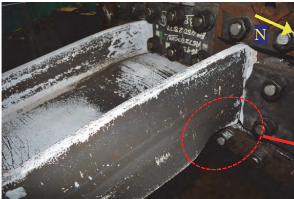
Figure 5.12 Specimen 11H-BC: LTB-Induced Flange Local Buckling at End of Test (West End)
