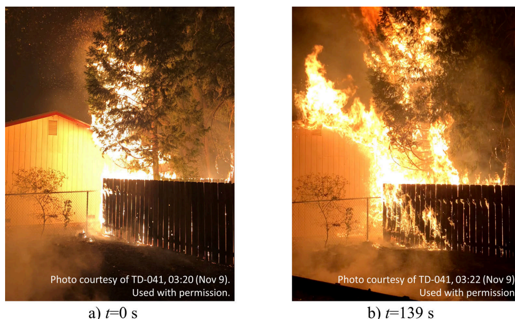
Figure 53. Structure ignition on Dade Ct in Magalia. Images are two minutes apart and show fire spread from surface fuels to fence to vegetation to eaves. The combustible fence is estimated to be approximately 1.8 m (6 ft) away from the structure.
