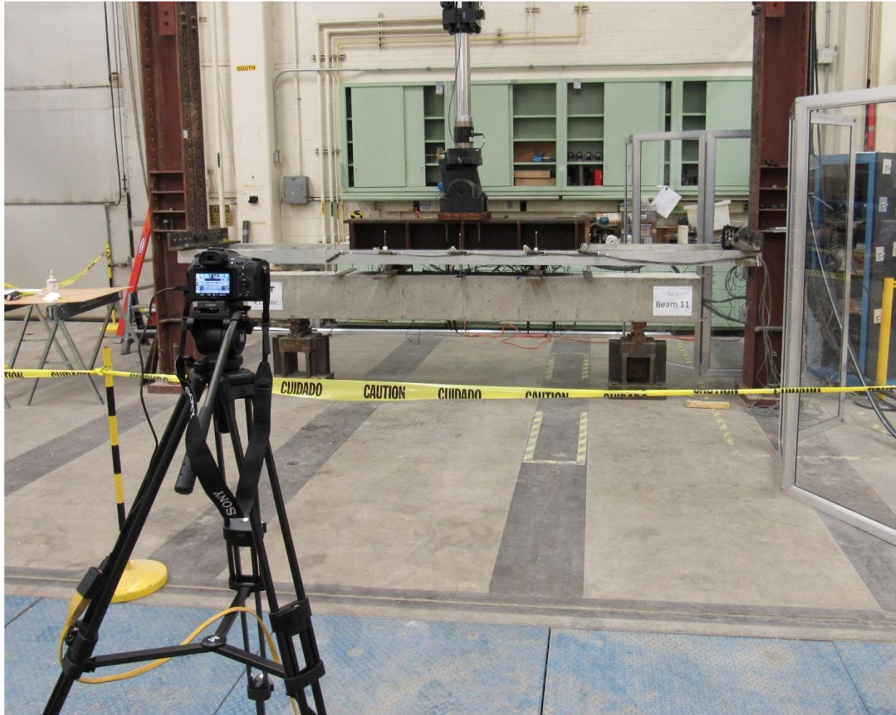
Figure 2.20. High-resolution camera position, relative to beam specimen
