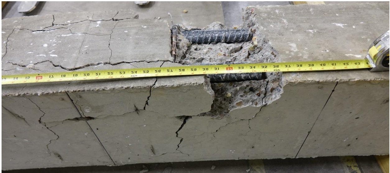
Figure 3.11. Beam 6 failure pattern (taken after testing with the beam flipped upside-down)
