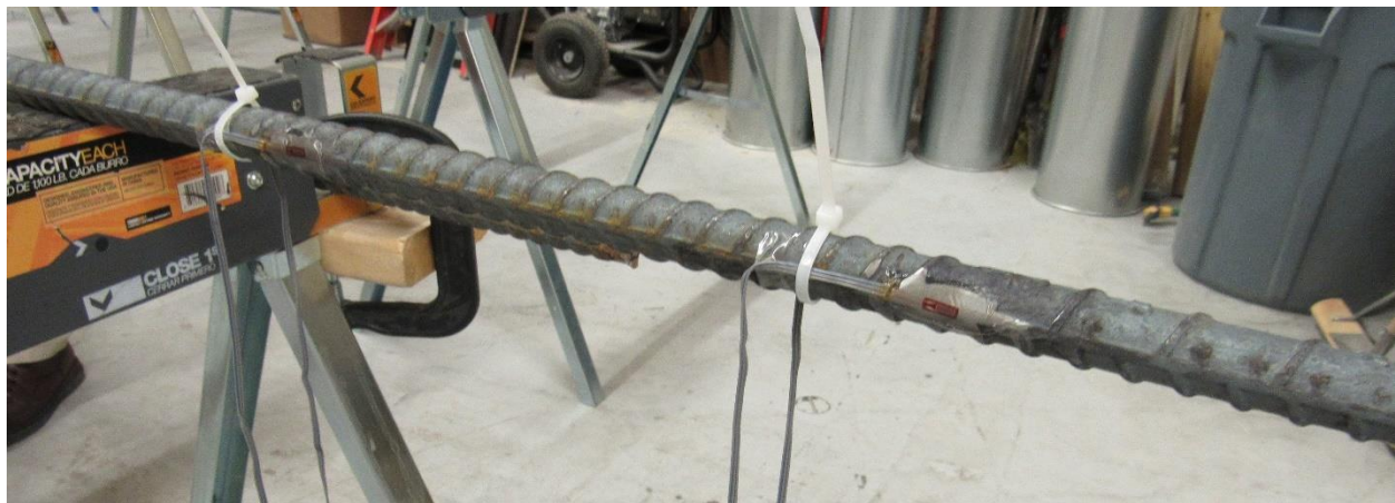
Figure 2.18. Strain gage application on longitudinal reinforcement
