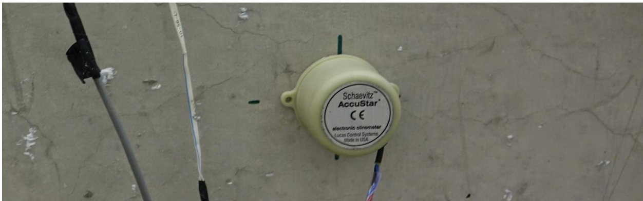
Figure 2.16. Inclinometers used to measure beam end rotation
