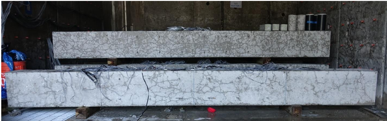
Figure 3.2. Beam specimens in environmental chamber
