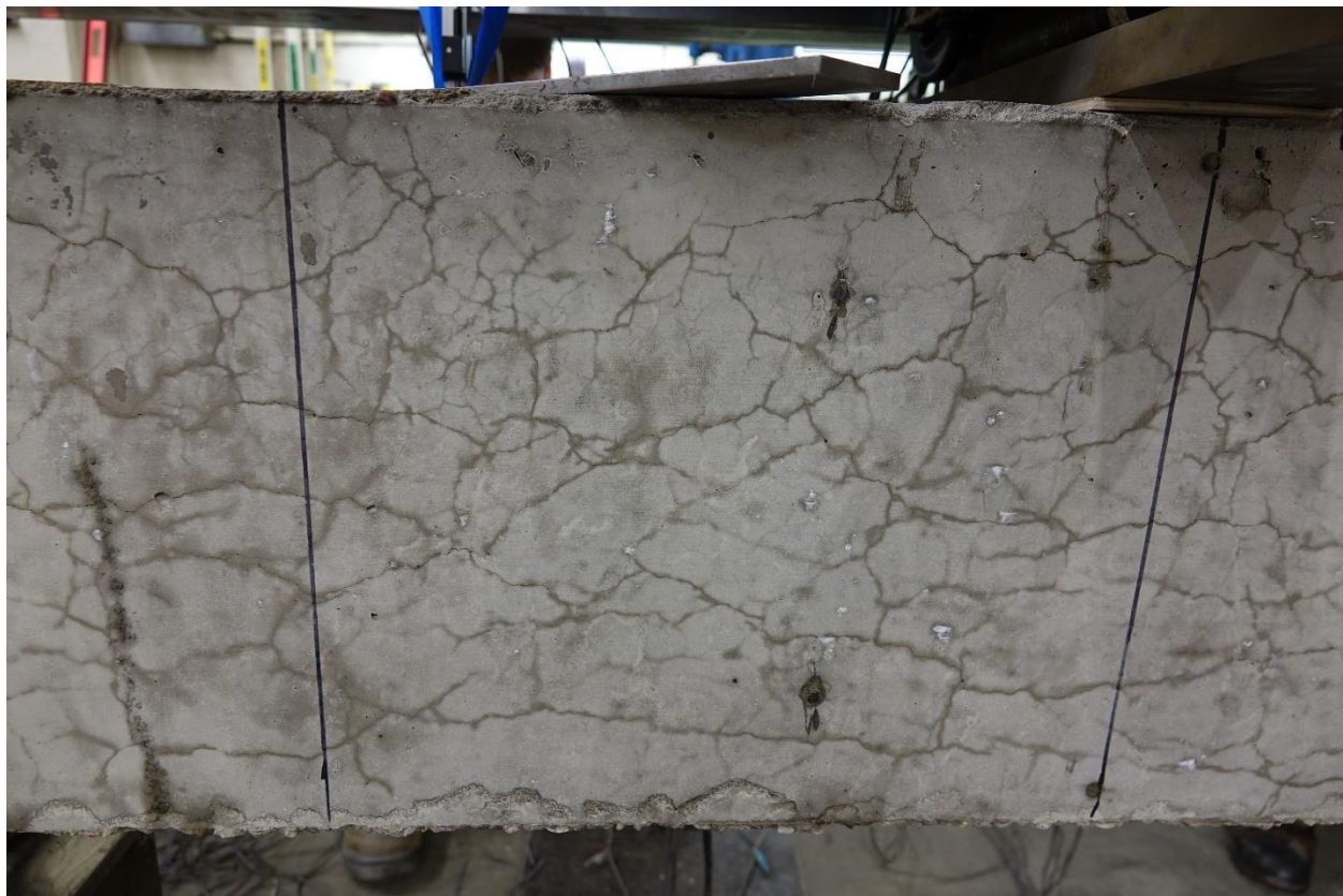
Figure 3.3. Beam 6 concrete condition prior to testing (with the surface of the beam wetted with rag to improve contrast)
