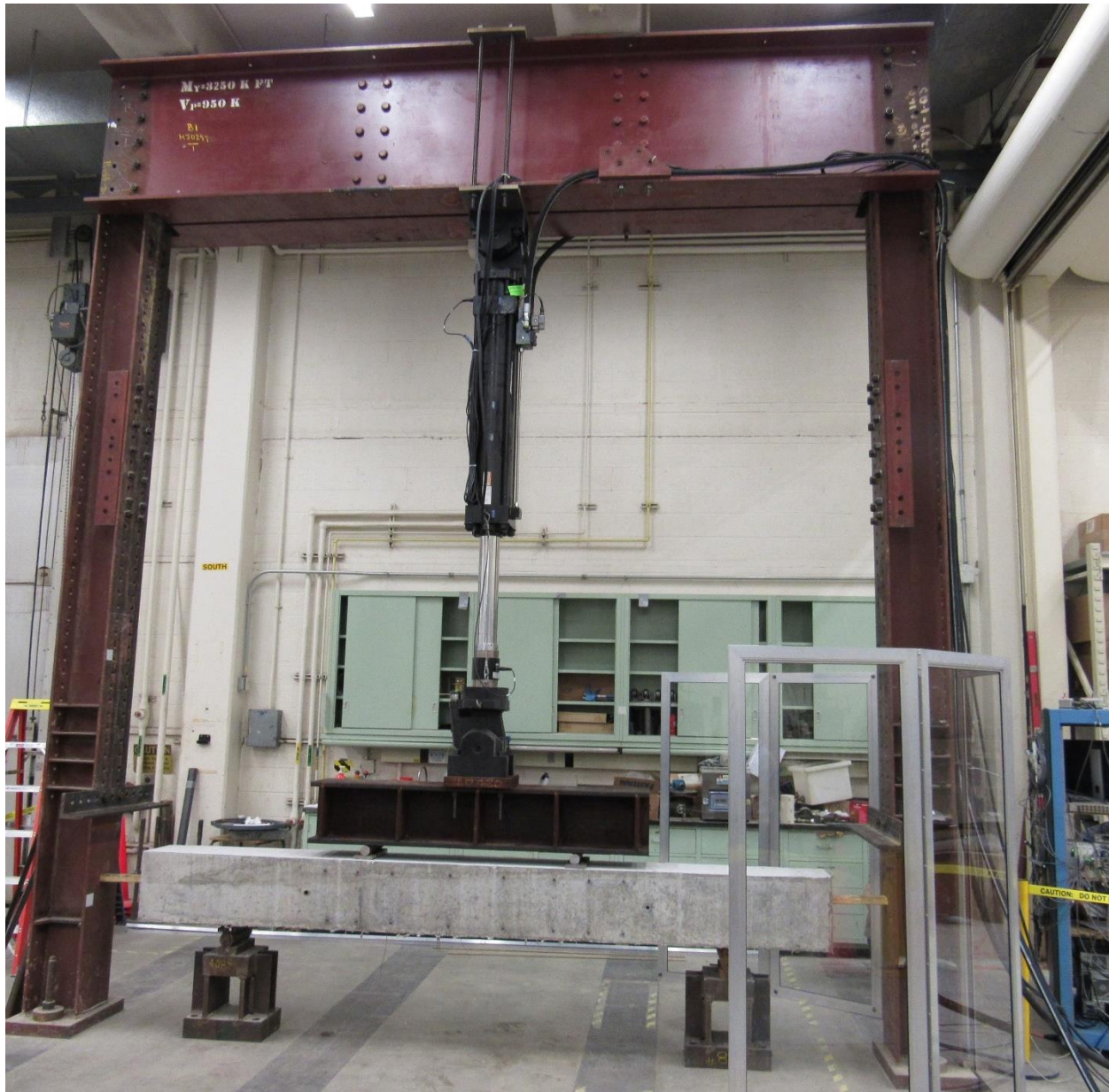
Figure 2.9. Beam test setup
