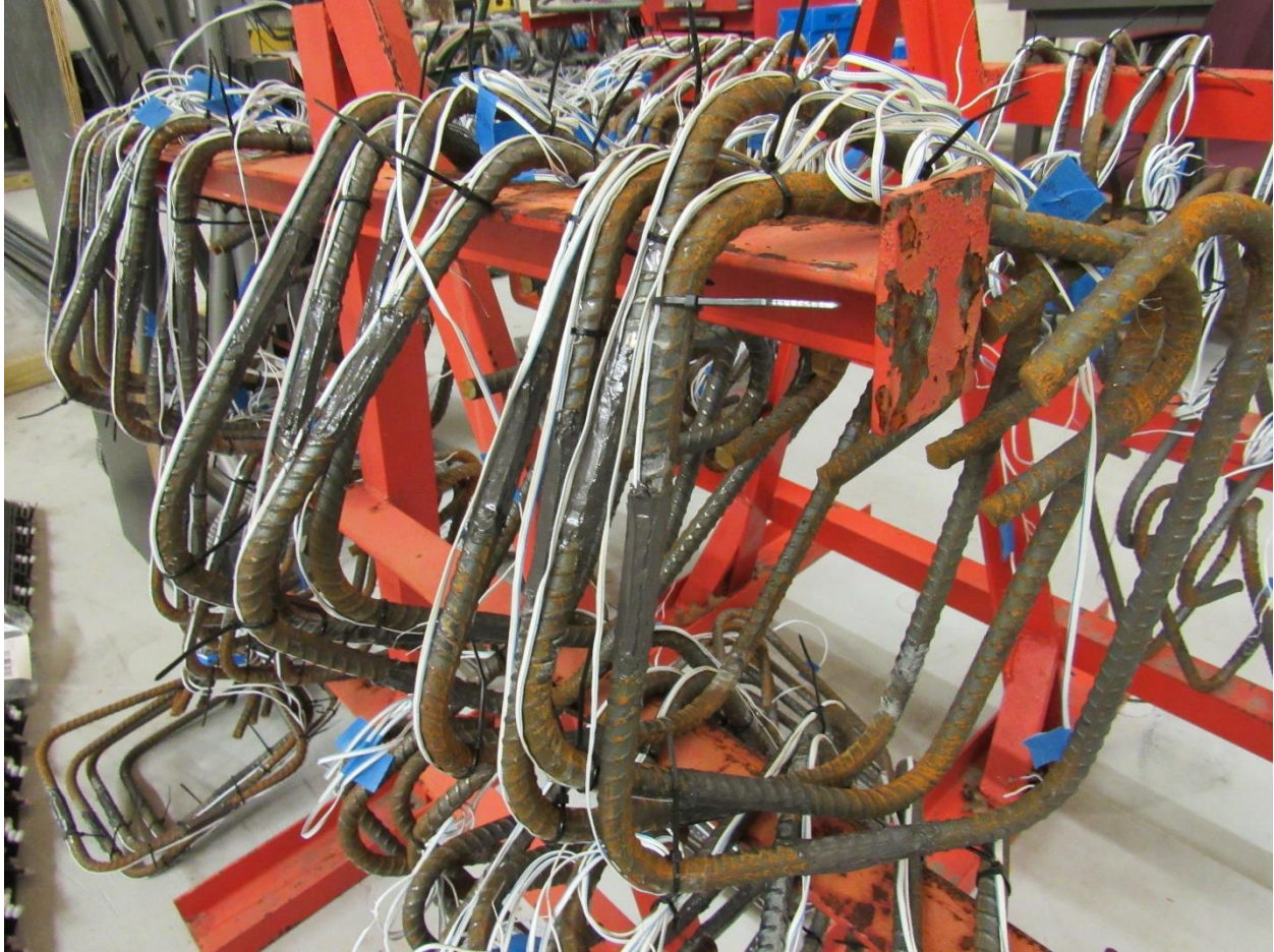
Figure 2.19. Strain gage protective coating on beam stirrups
