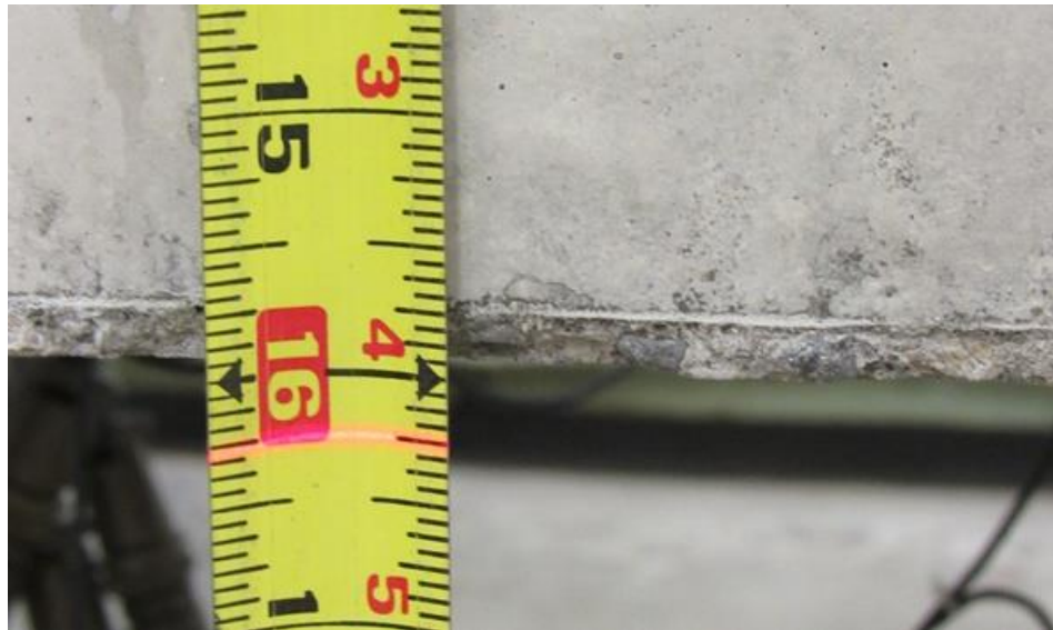
Figure 3.5. Beam 19 camber prior to testing
