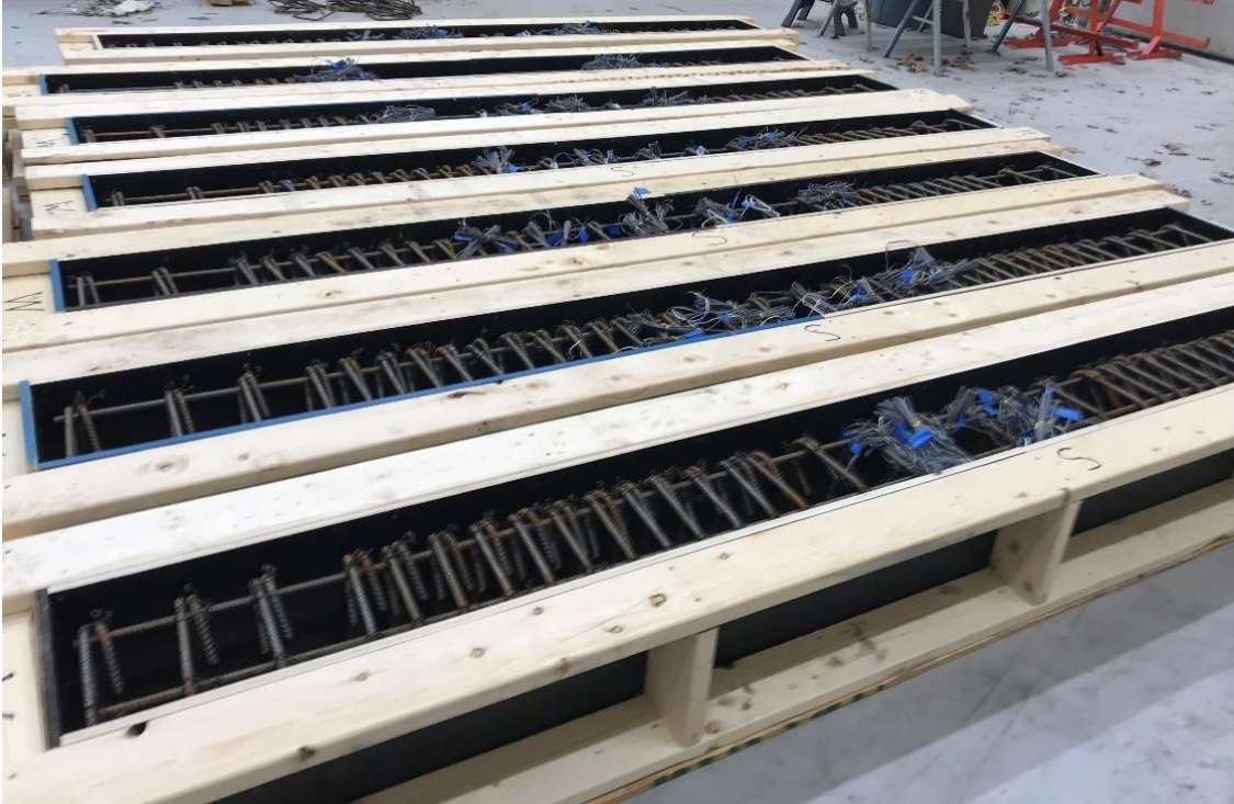
Figure 2.3. Formwork, reinforcement, and instrumentation of beam specimens
