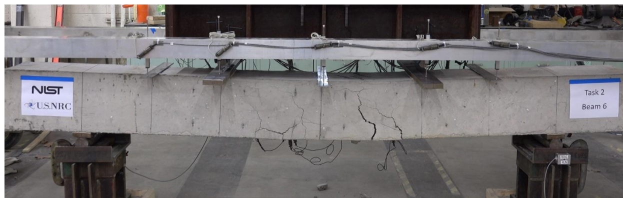
Figure 3.9. Beam 6 crack pattern at the end of testing
