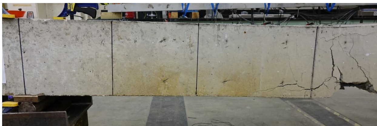
Figure 3.6. Beam 12 shear span and bearing regions at end of testing
