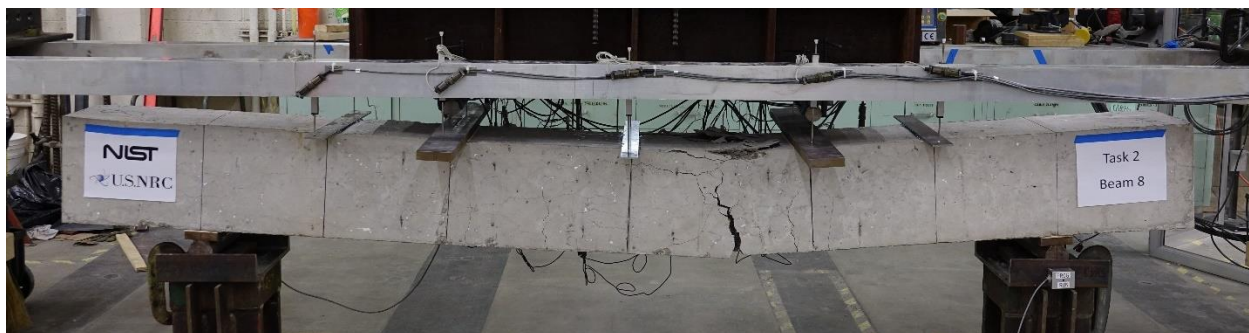
Figure 3.8. Beam 8 crack pattern at the end of testing
