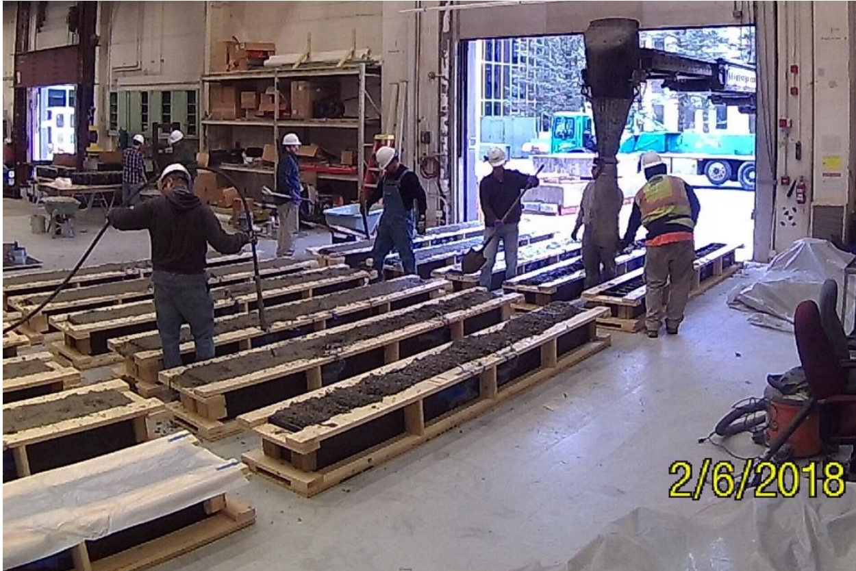
Figure 2.6. Concrete placement into beam's formwork and consolidation using vibrators
