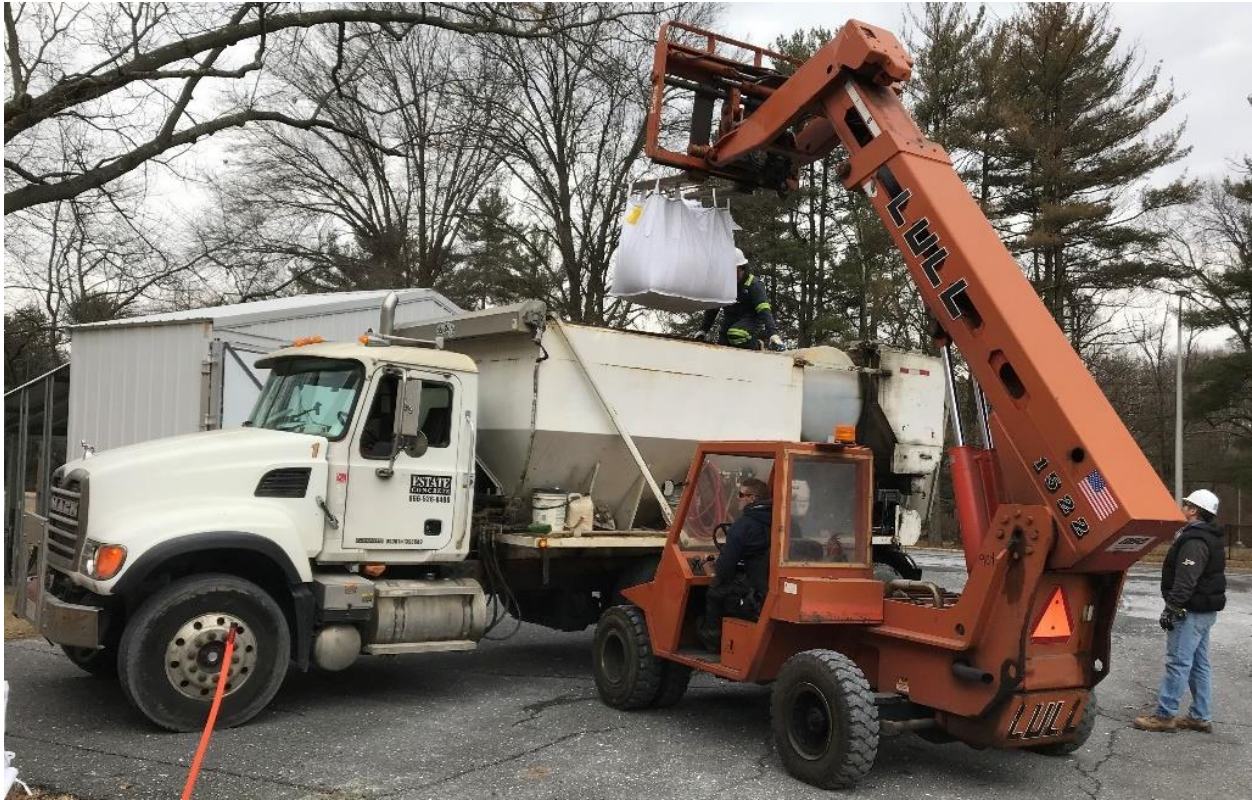
Figure 2.4. Loading of aggregates into volumetric truck mixer
